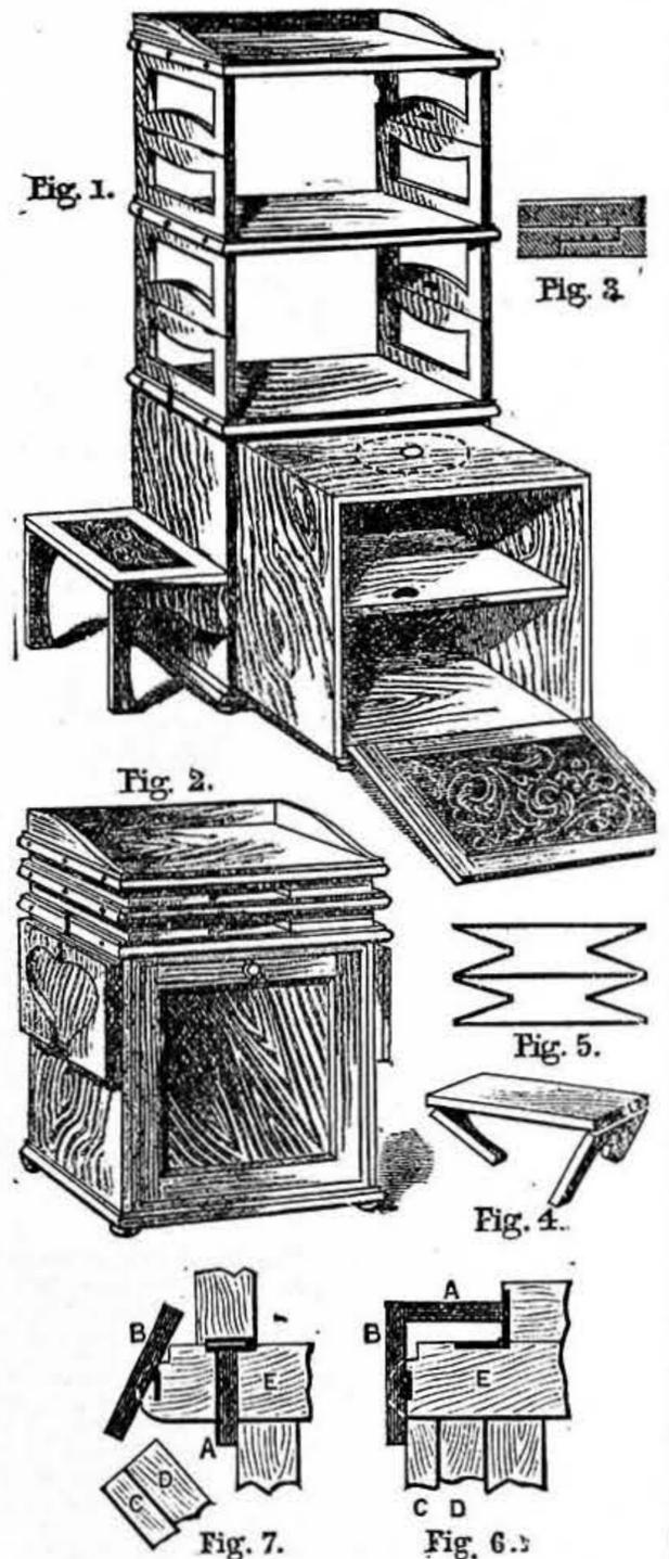
Fig. 1.—Commode, Clothes-holder, and Bed-steps fully displayed. Fig. 2.—Commode entirely closed. Fig. 3.—Bed-step Supports overlapping each other when folded. Fig. 4.—Diagram showing how Bed-step Supports fold. Fig. 5.—Skeleton Diagram, showing how Top Parts fold. Figs. 6 and 7.—Movement to retain Bed-step in Vertical Position.
