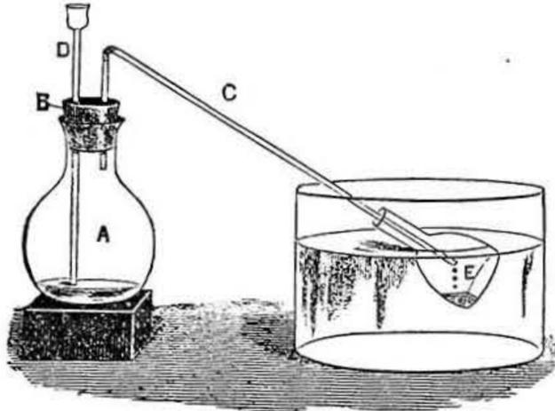
Apparatus for making Bromine—A, Flask; B, Cork or Caoutchouc Stopper; C, Delivery Tube; D, Acid Safety Tube; E, Condensing Flask.
