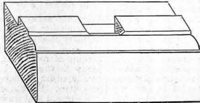
Fig. 5.—Diagram showing Mortise with Mitre to receive Top End of Tenon.
