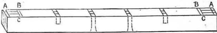
Fig. 2.—Top Rail set out showing Mortises and Tenons.
