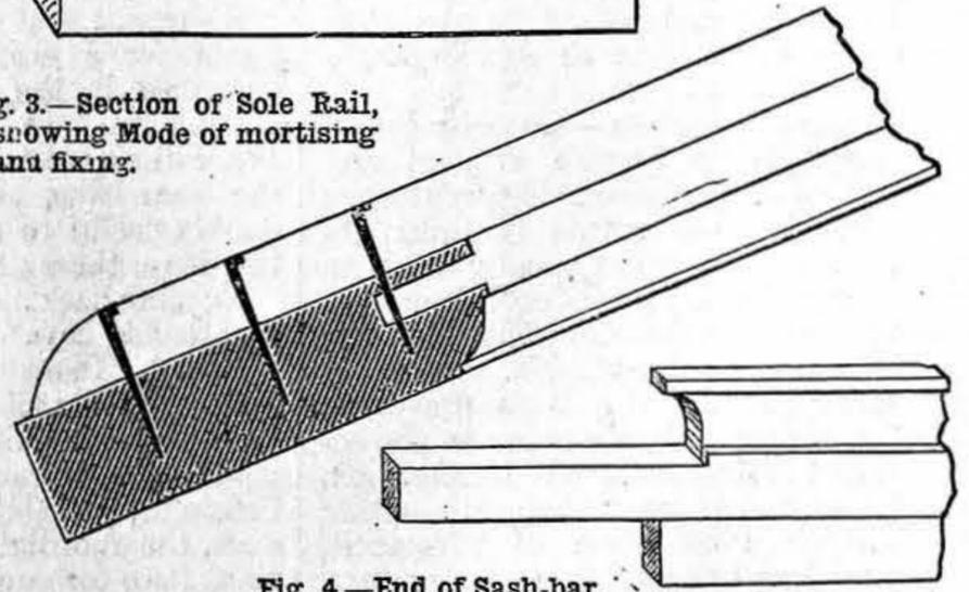
Fig. 4.—End of Sash-bar, showing Mode of fitting to Rail.
