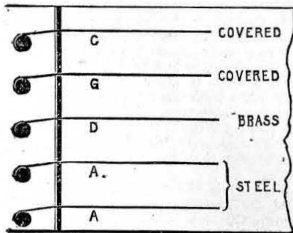
Fig. 4.—The Vienna Method, the one in Ordinary Use. The Strings bracketed are tuned alike.
