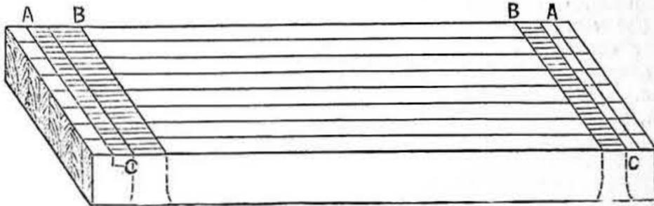
Fig. 1.—Stiles laid on Bench for setting out and showing Markings for Mortises.
