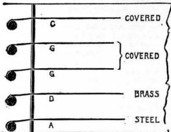
Fig. 3.—The Stuttgart Method, seldom used in England. The Strings bracketed are tuned alike.
