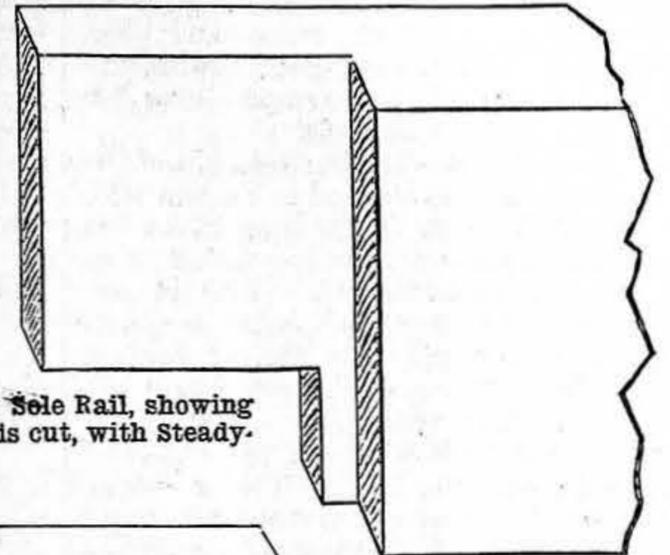
Fig. 6.—End of Sole Rail, showing how Tenon is cut, with Steadying Piece.
