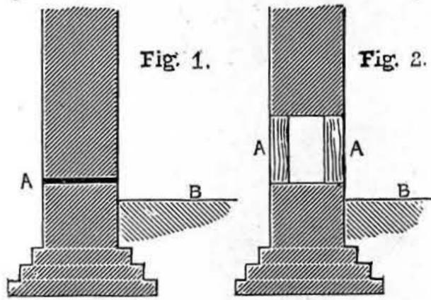
Fig. 1.—Diagram showing Position of Damp Course (A) and Ground Line (B). Fig. 2.—Diagram showing Method of Shoring Old Wall during Insertion of New Damp Course (A) and Ground Line (B).
