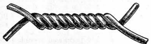
Fig. 50.—Section of Twisted Wire.
