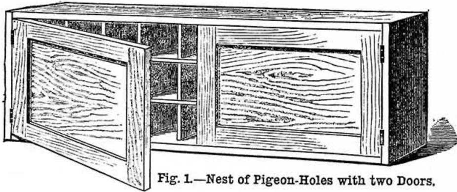
Fig. 1.—Nest of Pigeon-Holes with two Doors.
