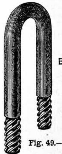
Fig. 49.—Staple of Twisting Machine.
