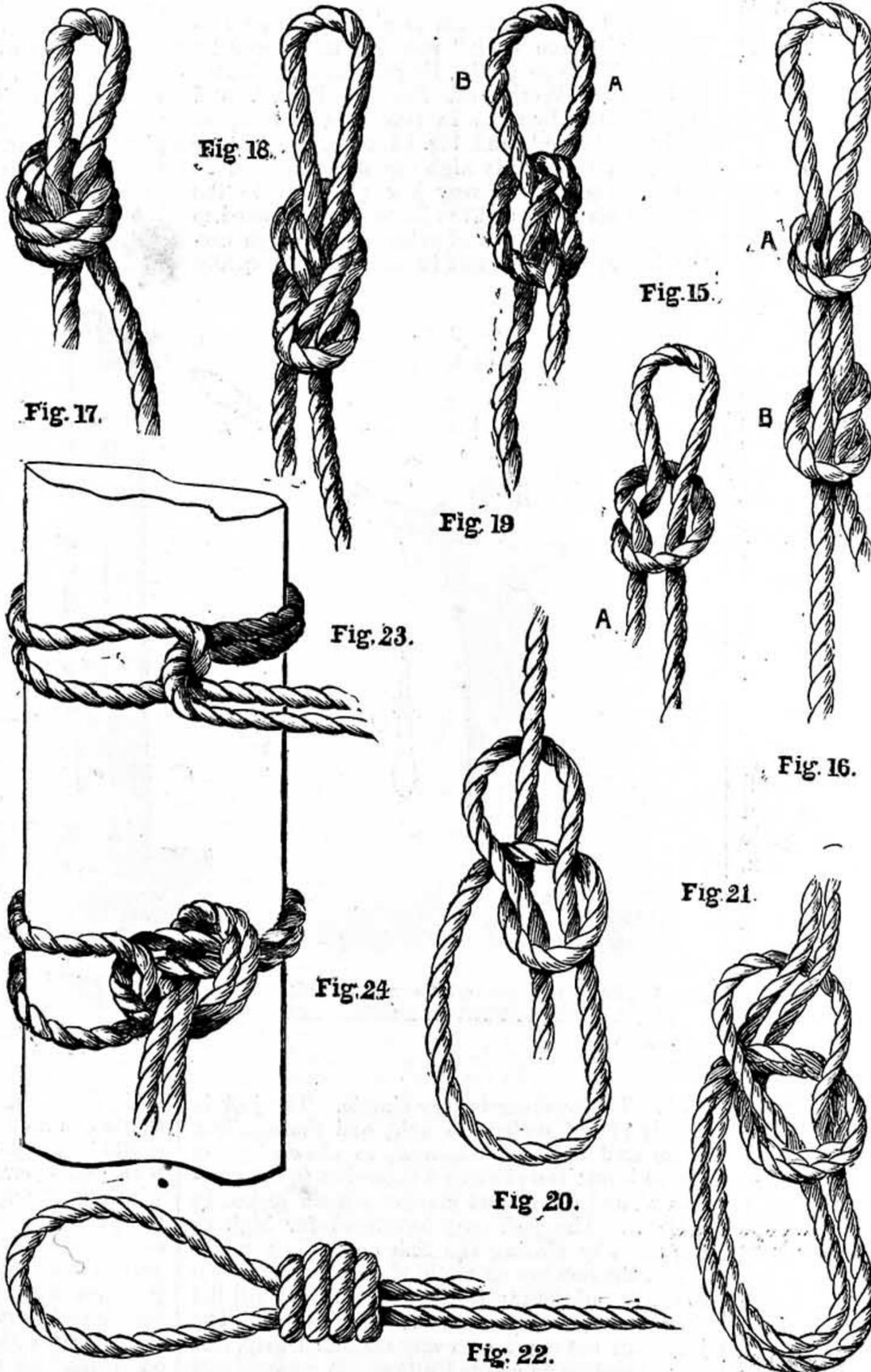
Fig. 15.—Running Knot. Fig. 16.—Fisherman's Eye. Fig. 17.—Openhand Eye. Fig. 18.—Flemish Eye. Fig. 19.—Crabber's Eye. Fig. 20.—Bowline. Fig. 21.—Running Bowline on Bight. Fig. 22.—Hangman's Knot. Fig. 23.—Running Knot with Two Ends. Fig. 24.—Ditto fastened.
