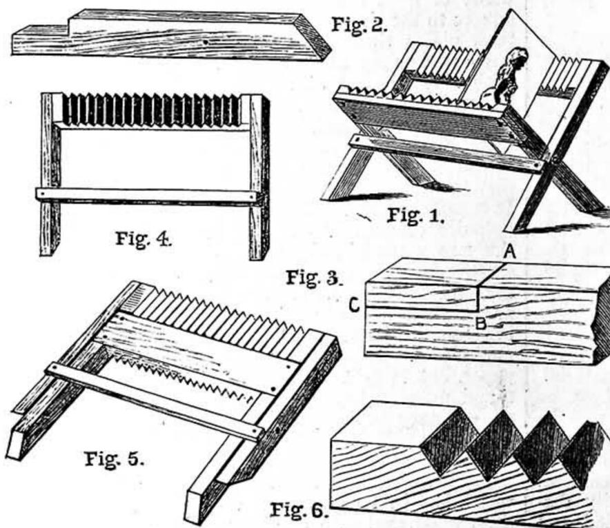
Fig. 1.—Folding Plate Draining Rack complete. Fig. 2.—Leg of Rack rebated. Fig. 3.—Mode of cutting Rebate. Fig. 4.—Grooved Strip at top of Side. Fig. 5.—Rack when folded. Fig. 6.—Mode of grooving Strips.
