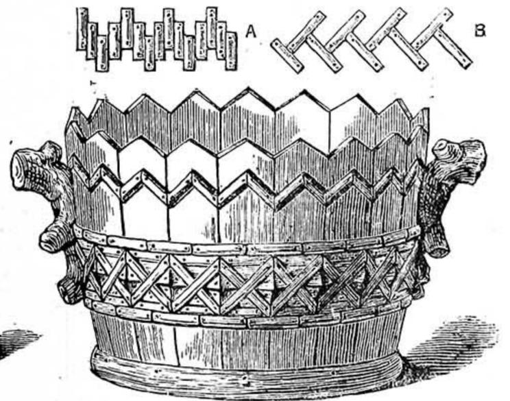
Fig. 2.—Garden Plant Tub made of other Half of Paraffin Cask—A, B, Alternative Modes of Moulding.
