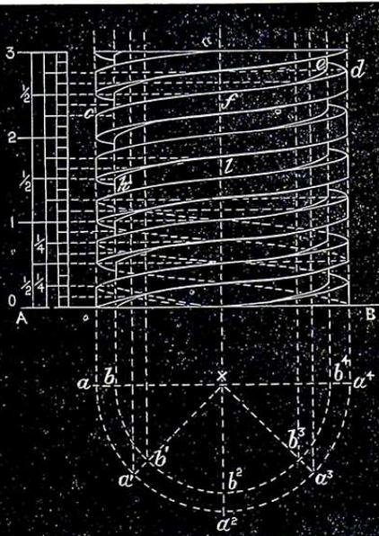
Fig. 17.—Double Square Thread Screw.
