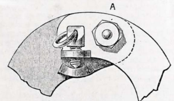
Tig. 1. - Joint of Metal Tree with Joint-Pin and Nut (A).
