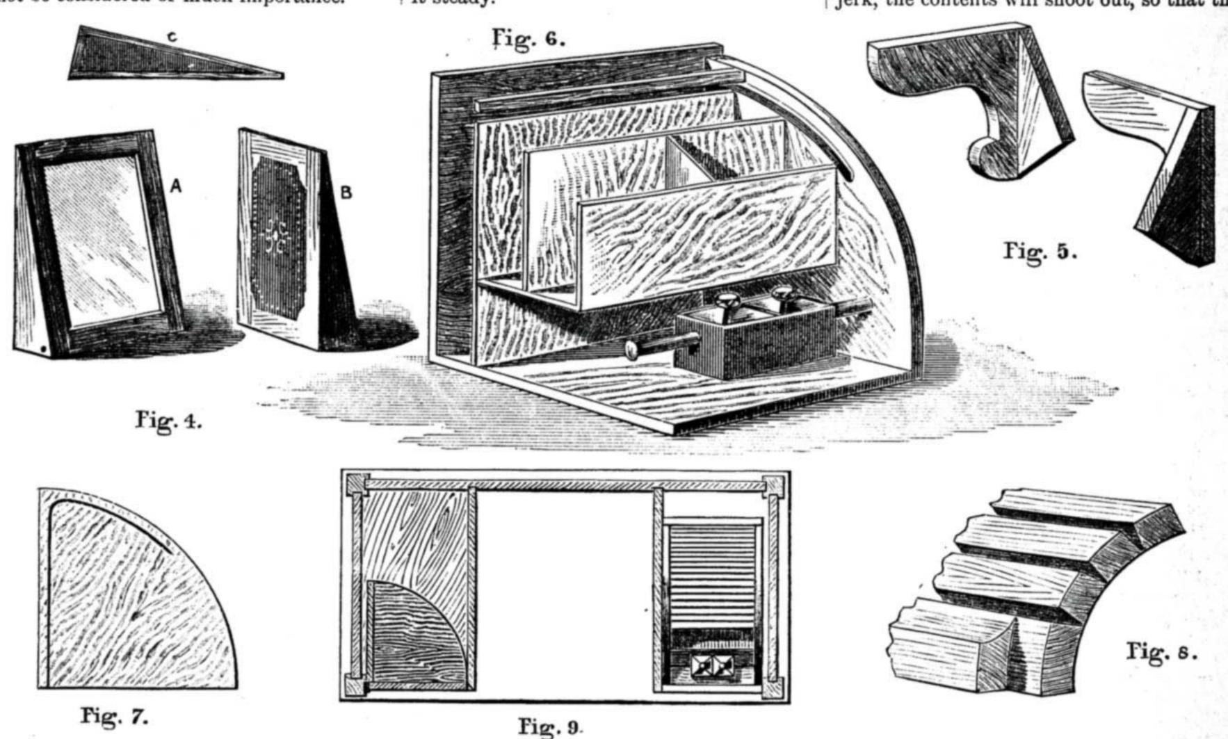
Fig. 4.—Diagram showing Desk and Glass Frame—A, Looking Glass Side; B, Desk Side; C, Section. Fig. 5.—Two Views of Bracket to support Desk and Glass Frame. Fig. 6.—Inside of Right-hand Lower Cupboard as Stationery Box with Revolving Inkpot Case. Fig. 7.—Side of Stationery Box, the Black Line indicating how Groove should be cut to receive Revolving Shutter. Fig. 8.—Bottom Lath. Fig. 9.—Plan of Lower Carcase.
