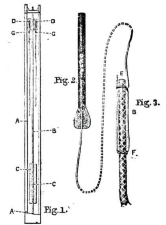
Sash-Hanging Parts. Fig. 1.—Sash Beadings, etc. Fig. 2.—Lead flattened and then bent round Cord. Fig. 3.—Method of fastening Mouse, on to End of Sash Line.
