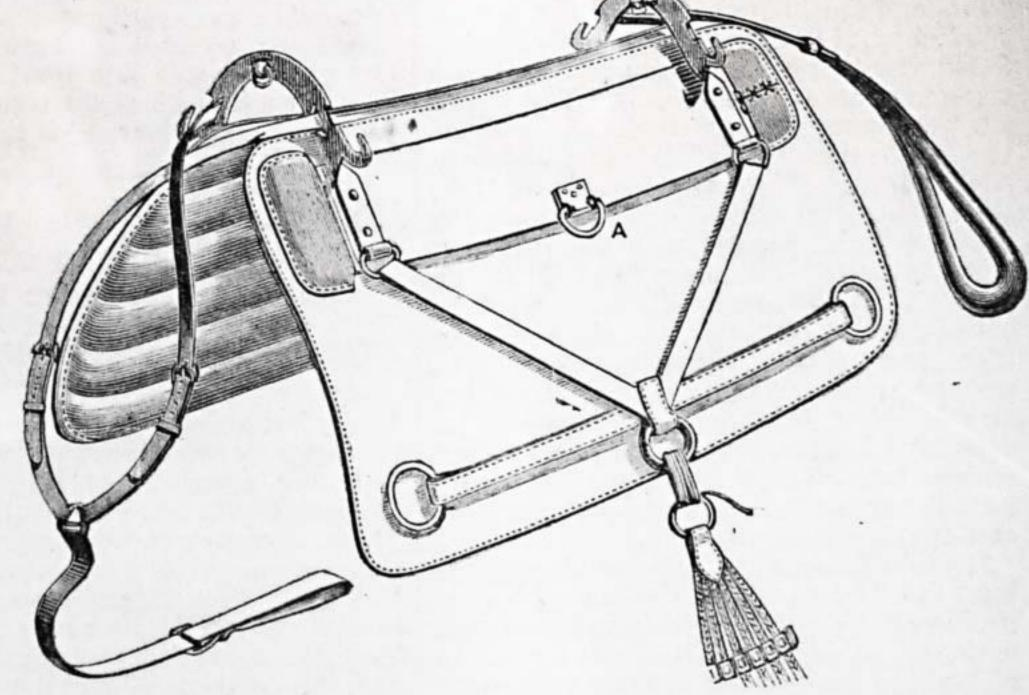
Fig. 2.—Pack-Saddle, showing Metal Trees above Panels, Tie-bars, etc., and Ring (A) placed on the Bars of the Tree for Girthing up to a Donkey.
