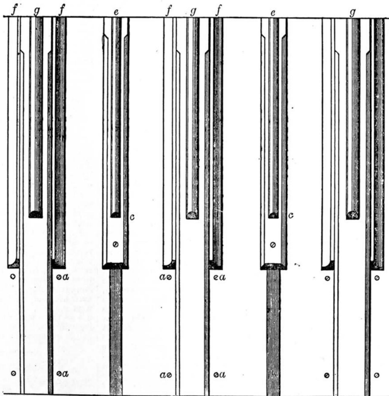
Fig. 2.—Wood Ceiling with Floor above, in Plan.
