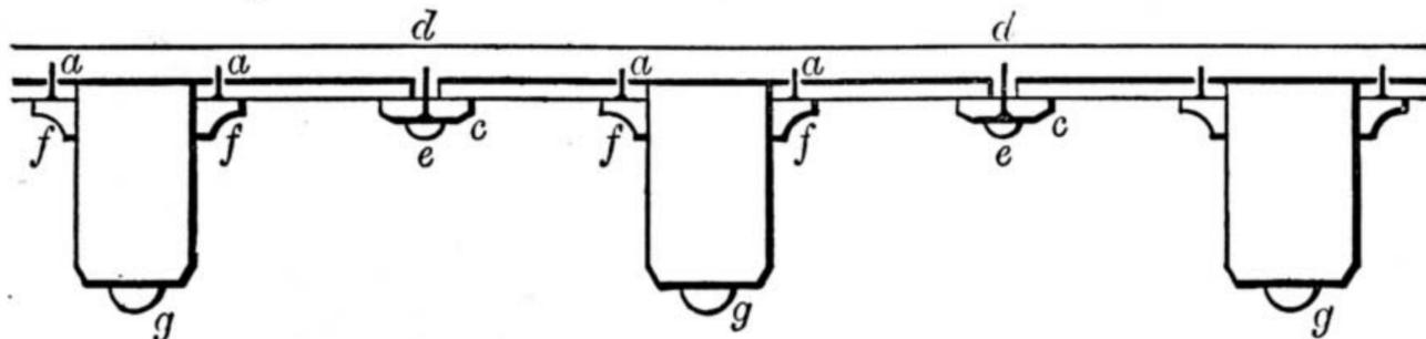
Fig. 1.—Wood Ceiling with Floor above, in Section.
