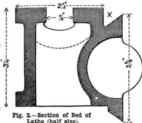
Fig. 2.—Section of Bed of Lathe (half size).
