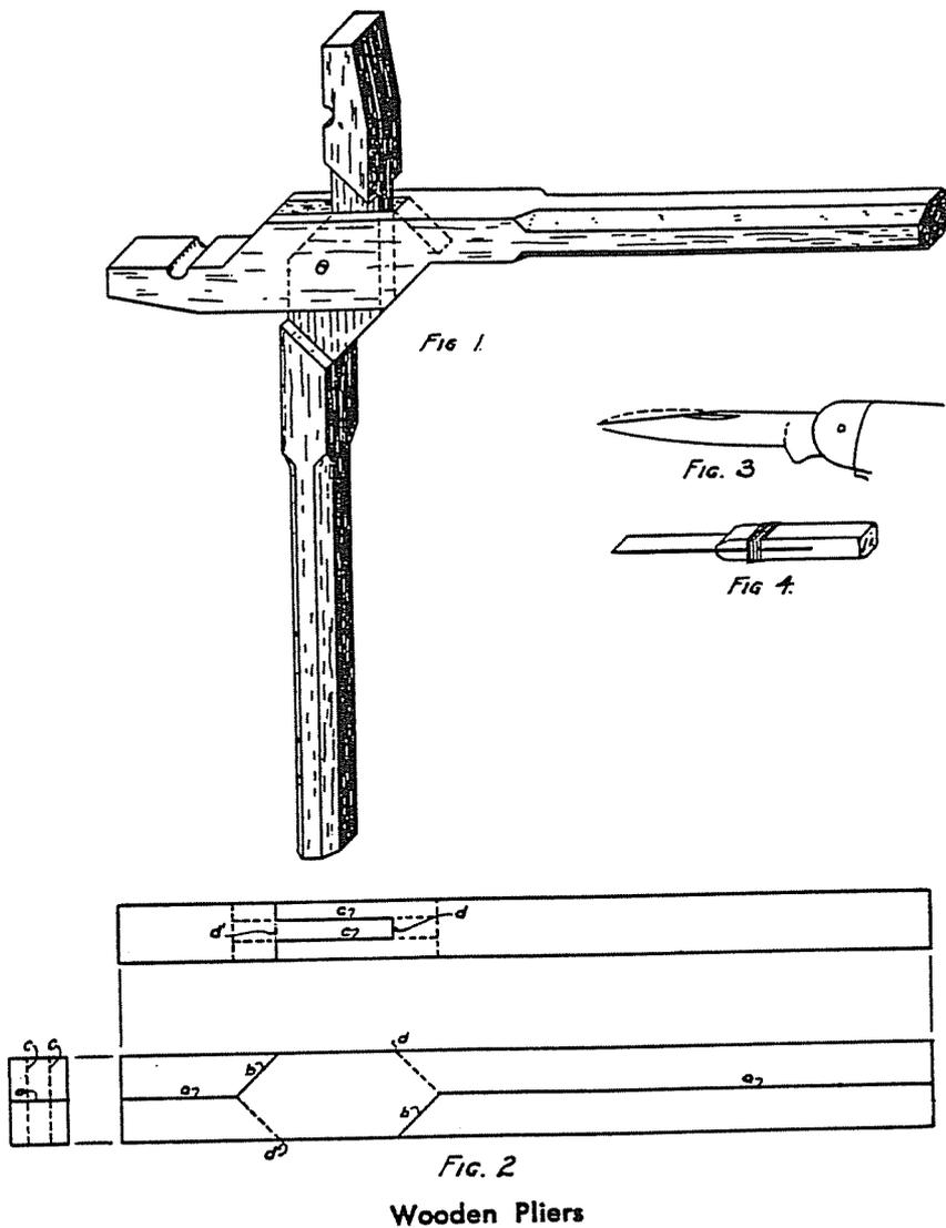
First, the piece should be scored part way through the two center lines marked *a* in Figure 2. These should be scored on both sides and ends, omitting the hexagonal space shown that should be at least twice the width of the piece.
