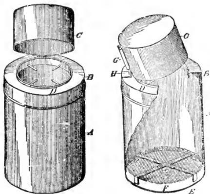
Fig. 4—Varnish Brush Keeper.
