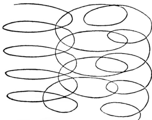
Fig. 19—The Motions in French Polishing.
