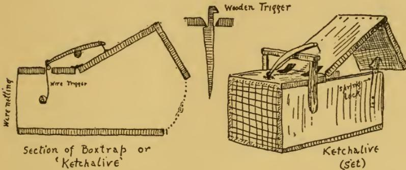
ketchalive or old-fashioned box trap is made in a hundred different ways; but the main principles are shown in the illustration. The lock on the side is necessary for some species, such as skunks, that would easily lift the lid and escape.
