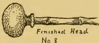
Now pad the head an inch thick with the ordinary horsehair stuffing that is used in furniture, and bind all with strong burlap, sewing it at the seams, and lashing it around the bamboo with string (No. 8). This completes the dry land spear. If for use in the water, make a final cover out of rubber cloth. This keeps the spear dry. A completed spear weighs about  $1\frac{1}{2}$  lbs.
