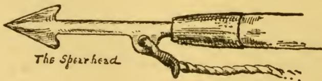
attached twenty feet of one-quarter-inch rope. On each rope, six feet from the spearhead, is a fathom mark made by tying on a rag or cord.
