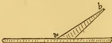
Place it on a level, solid post or stump in the open. At night set the dial so that the twelve o'clock line points exactly north, as determined by the Pole Star and nail it down. Then, fix a stick or pointer with its upper edge on the centre and set it exactly pointing to the Pole Star (a b); that is, the same angle as the latitude of the place, and fix it there immovably;
