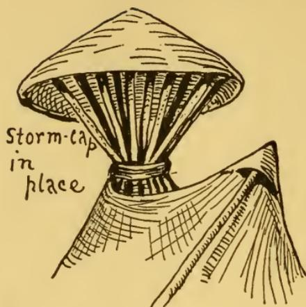
canvas with a hem edge in which is a limber rod to keep it in circular shape. It is usually put on with a loose teepee pole, and sits on top of the poles as shown, held down if need be by cords to its edge.
