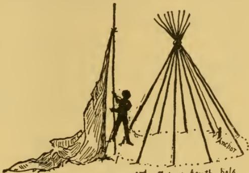
3<sup>rd</sup> Set up tenth pole with teepee cover fastened to it by lark rope
