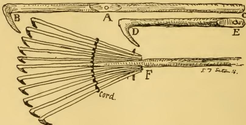
thick (*BC*) and 4 feet long, of the shape shown. Flatten it on each side of *A*, and make a gimlet-hole through. Now cut ten branches of the shape *DE*, each about 20 inches long. Flatten them at the *E* end, and make a gimlet-hole through each. Fasten all together, 5 on each side of the handle,
