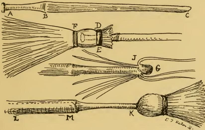
an inch thick, and shape it to a shoulder, as in *A B C*. Lash on birch or other fine twigs, one layer at a time, until sufficiently thick, as *D E*. Now at *F*, put a final lashing of cord. This draws the broom together, and binds it firmly to the handle. Trim the ends even with the axe, and it is ready for use.
