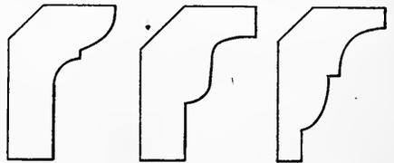
FIG. 160.—CROWN MOULDS.
