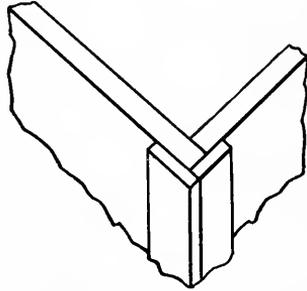
FIG. 116.—BUTT JOINT (CLEATED).
