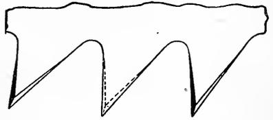
FIG. 196.—TEETH OF RIP SAW (CIRCULAR).
