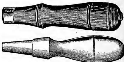
FIG. 48.—CHISEL HANDLES. UPPER, TANG; LOWER, SOCKET FIRMER.
