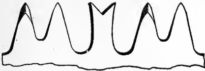
FIG. 195.—TEETH OF TWO-MAN CROSS-CUT SAW.
