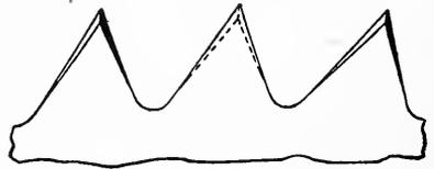
FIG. 197.—TEETH OF CUT-OFF SAW (CIRCULAR).
