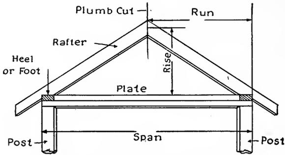
FIG. 177.—RUN AND RISE—COMMON RAFTER.
