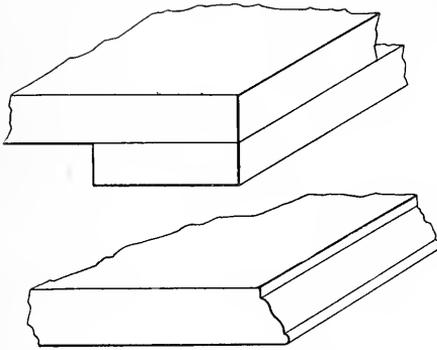
FIG. 143.—TRIMMING THE TOP.
