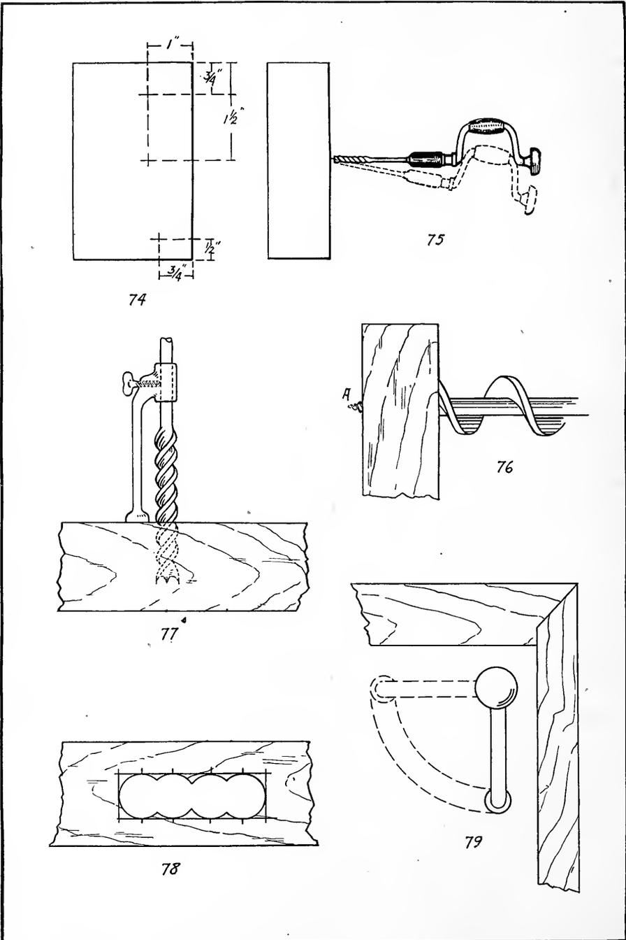
FIG. 74.—LOCATING CENTERS. FIG. 75.—STARTING BIT. FIG. 76.—BORING THROUGH.
