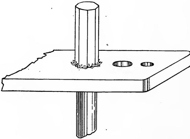
FIG. 99.—USE OF A DOWEL PLATE.
