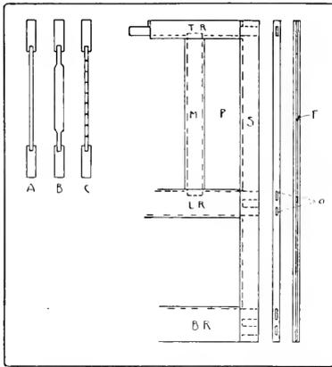
Fig. 288. Door, illustrating Panel Construction: S, Stile; T. R., Top Rail; L. R., Lock Rail; B. R., Bottom Rail; M., Muntin; P., Panel; A, Double Mortise-and-Tenon; F., Fillet; A, B, C, Forms of Panels.
