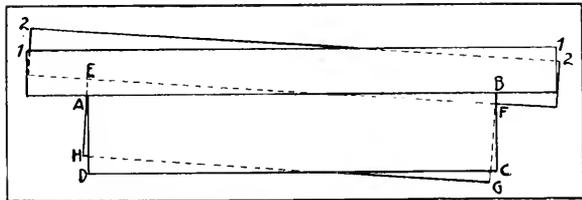
Fig. 206. Method of Using the Winding-Sticks.
