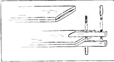
Fig. 58. Clamping up Boards to Prevent Warping.
