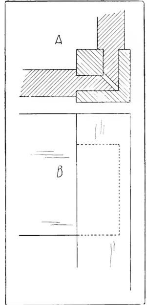
Fig. 291. A. Cross-Section Thru Back Leg and Adjoining Rails of Table. (Plan). B. Elevation, Showing Wide Shoulder on Tenon of Rail.
