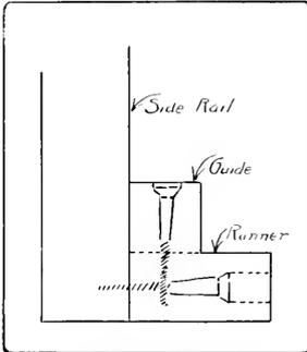
Fig. 295. Drawer Mechanism.
