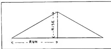
Fig. 198. The "Run" and "Rise" of a Rafter.
