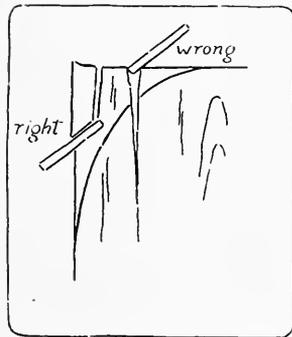
Fig. 75. Right and Wrong Ways of Perpendicular Chiseling.
