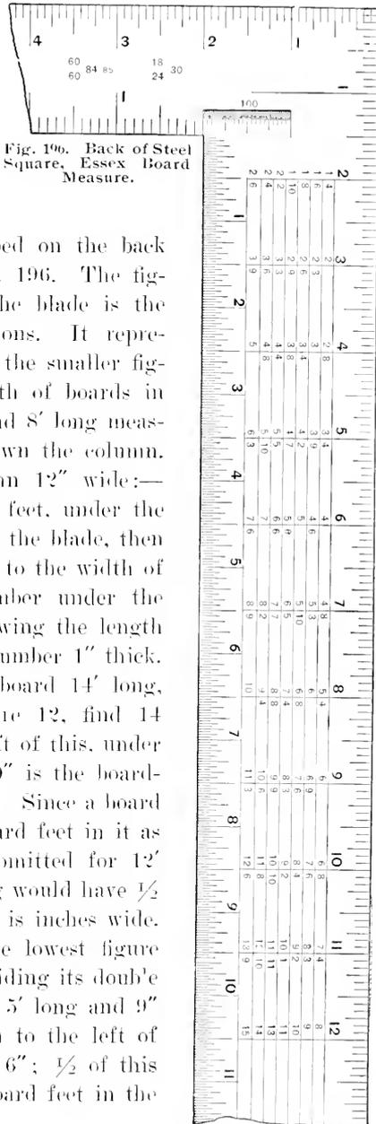
Fig. 196. Back of Steel Square, Essex Board Measure.
