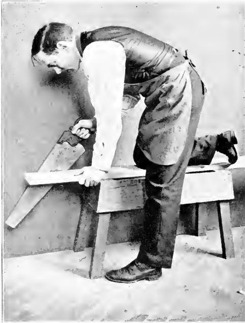
Fig. 88. Rip-Sawing on a Horse.
