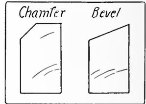
Fig. 271. Difference Between Chamfer and Bevel.
