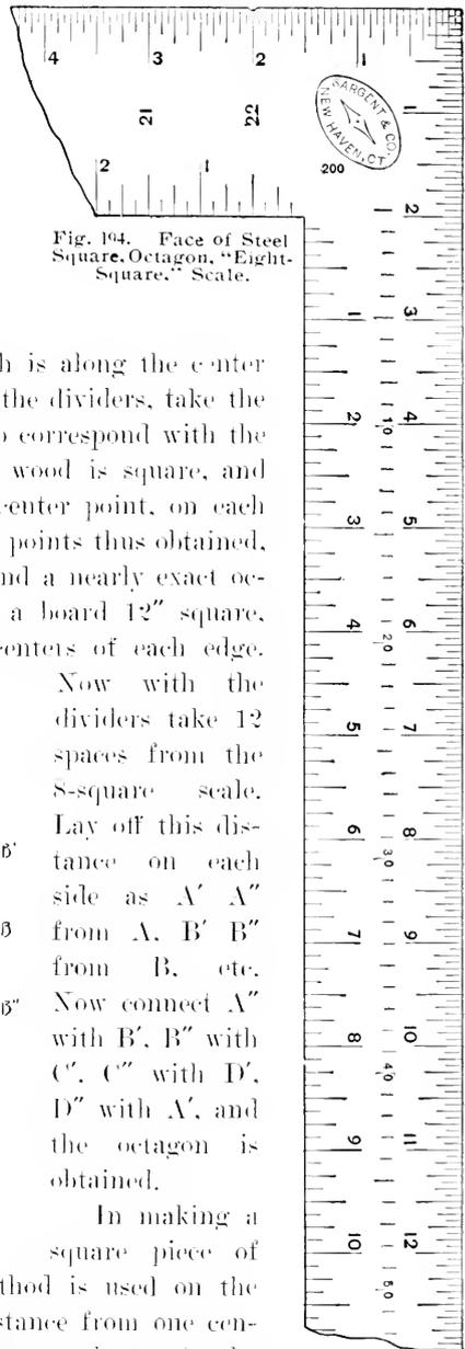
Fig. 194. Face of Steel Square, Octagon, "Eight-Square," Scale.
