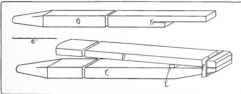
Fig. 223. Holder for Grinding Chisels or Plane-Bits.
