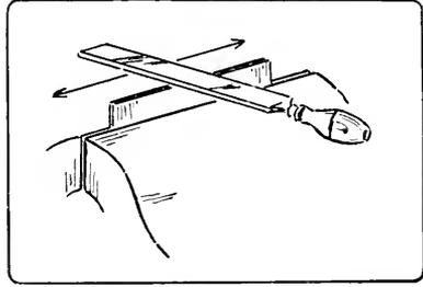
Fig. 153. Sharpening a Cabinet-Scraper: 1st Step, Drawfiling.
