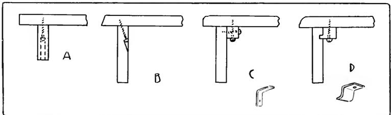
Fig. 297. Methods of attaching Table Top to Rails.
