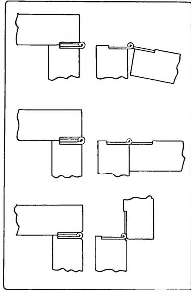
Fig. 235. Three Positions of Hinges.
