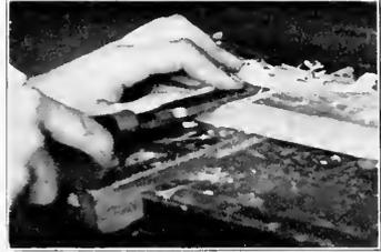
Fig. 71. Chiseling Out a Dado (Second Step).
