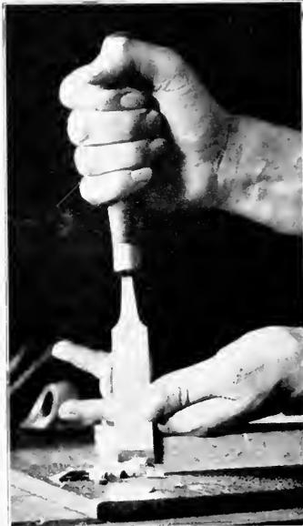
Fig. 72. Perpendicular Chiseling.
