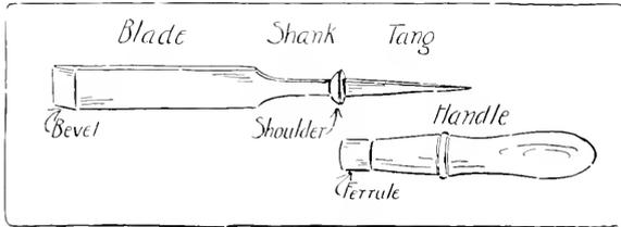
Fig. 65. Firmer-Chisel.
