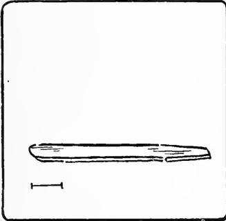
Fig. 110. Cutter of Scrub-Plane.
