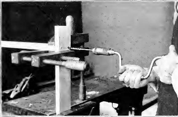
Fig. 247. Thru Boring for a Butt Joint.
