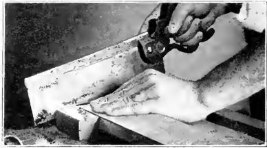
Fig. 90. Using the Back-Saw with Bench-Hook.
