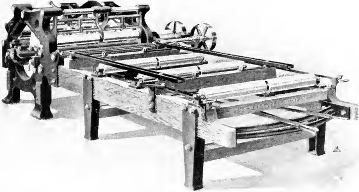
Fig. 43. Double Gang Edger. This machine trims off the rough edges<sup>s</sup> of the "wancy" boards by means of the four saws in the main frame of the machine.
