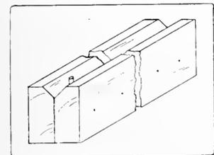
Fig. 274. Trough for Planing Chamfers.
