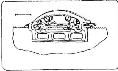
Fig. 97. A Saw-Jointer.
