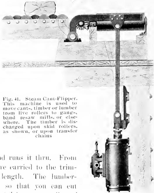
Fig. 41. Steam Cant-Flipper. This machine is used to move cants, timber or lumber from live rollers to gauges, band resaw mills, or elsewhere. The timber is discharged upon skid rollers, as shown, or upon transfer chains.
