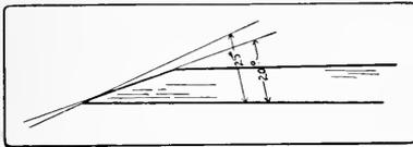
Fig. 78. Grinding Angle, 20°;
