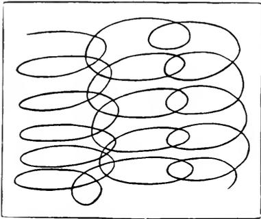
Fig. 304. Direction of the Pad in French Polishing.
