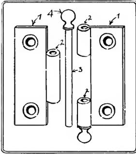
Fig. 234. Parts of a butt-hinge.
