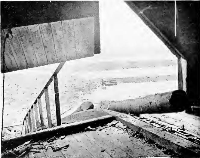
Fig. 36. Jack-Ladder, with Endless Chain.
