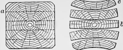
FIG. 15.—Warping of planks cut from an unseasoned log.
