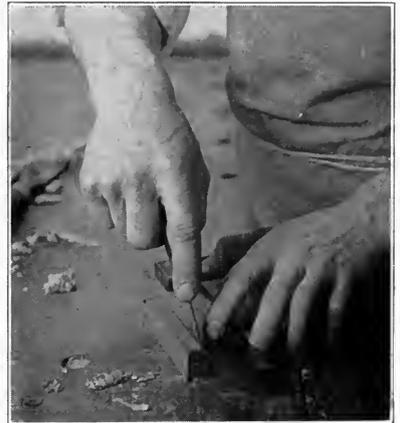
Fig. 35. Scoring with a knife along the try-square.
