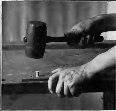
Fig. 132. Driving dowel thru dowel-plate.
