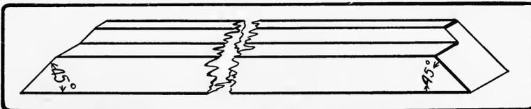
Fig. 79. Rabbeted and mitered member of picture-frame.
