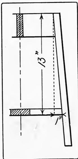
Fig. 151. Obtaining the batter for slanting legs.
