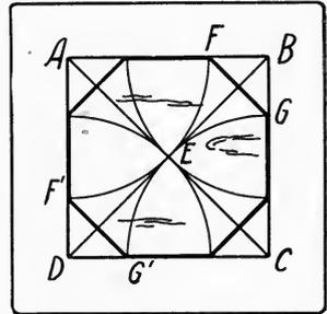
Fig. 144. One method of laying out an octagon.
