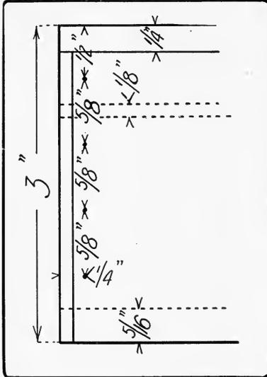
Fig. 188. Location of brads in end of box.
