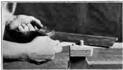
Fig. 139. Sawing off projecting end of dowel-pin.
