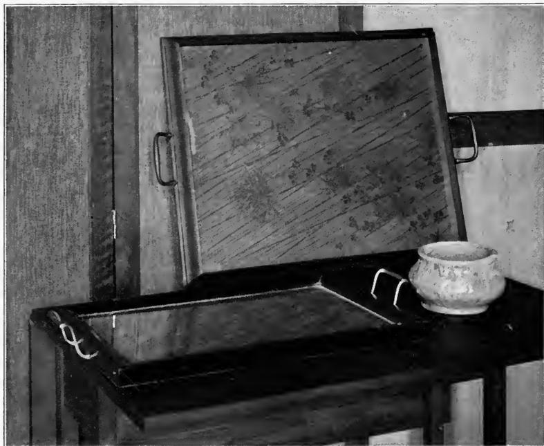
Fig. 94. Glass bottomed trays made with mitered frames.
