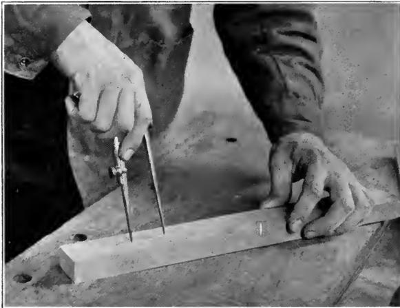
Fig. 58. Stepping off distances with the dividers
