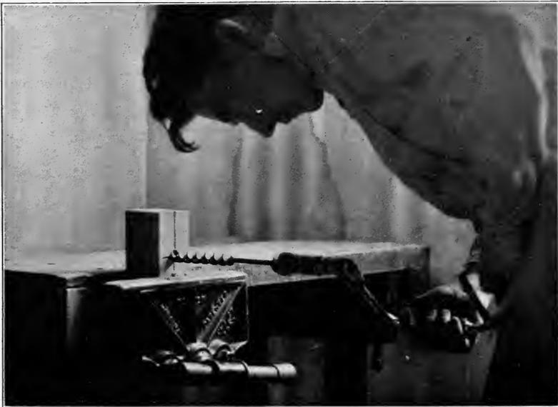
Fig. 156. Boring hole in head of mallet.
