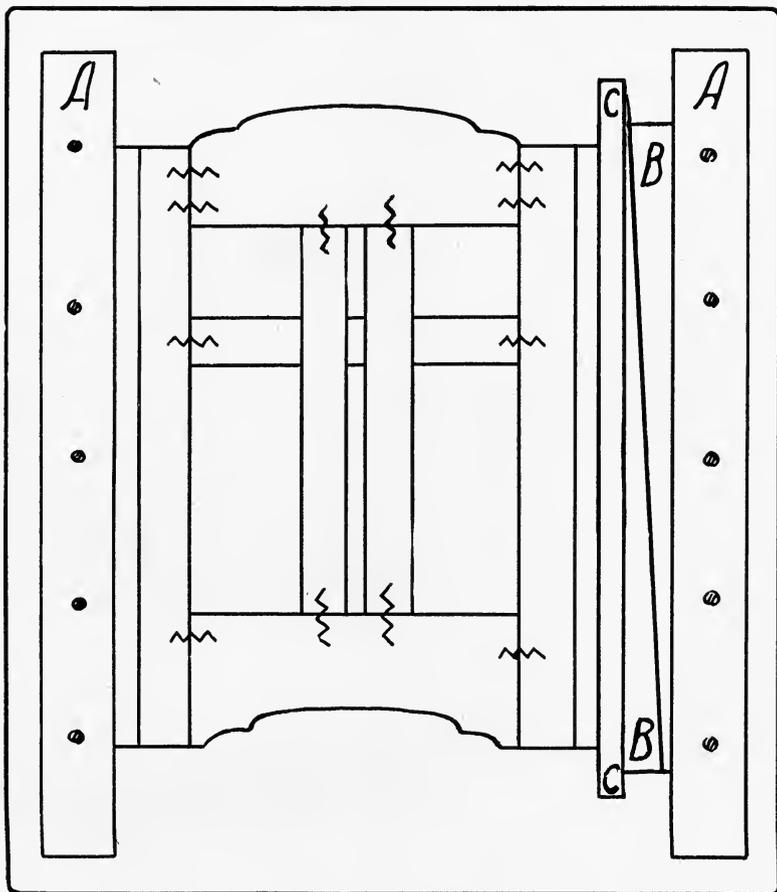
Fig. 200. Method of clamping up the parts.
