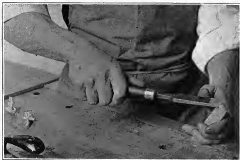
Fig. 33. Slicing off an arris with a chisel.
