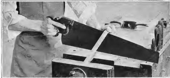
Fig. 30. Ripping with wood held in vise.
