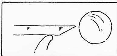
Fig. 183. Scraping the knob on the lathe.
