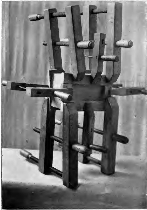
Fig. 192. Gluing the top on to the box.
