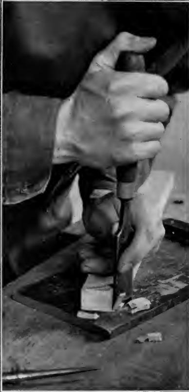
Fig. 56. Perpendicular chiseling.
