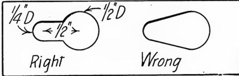
Fig. 59 Shape of holes in picture-frame-clamp.
