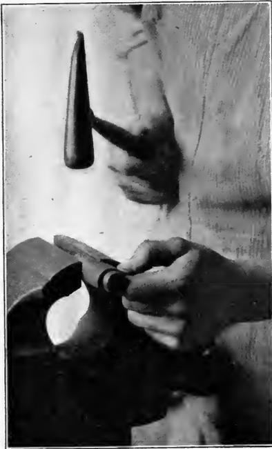
Fig. 108. Hammering a strip into a cylinder.
