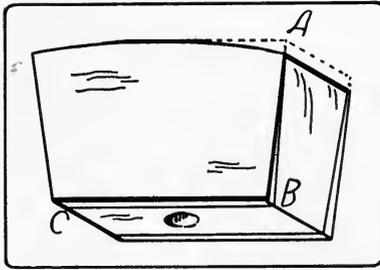
Fig. 161. Lay-out for beveled sides. (Seen from below.)
