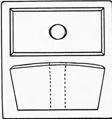
Fig. 157. How the handle hole tapers out.
