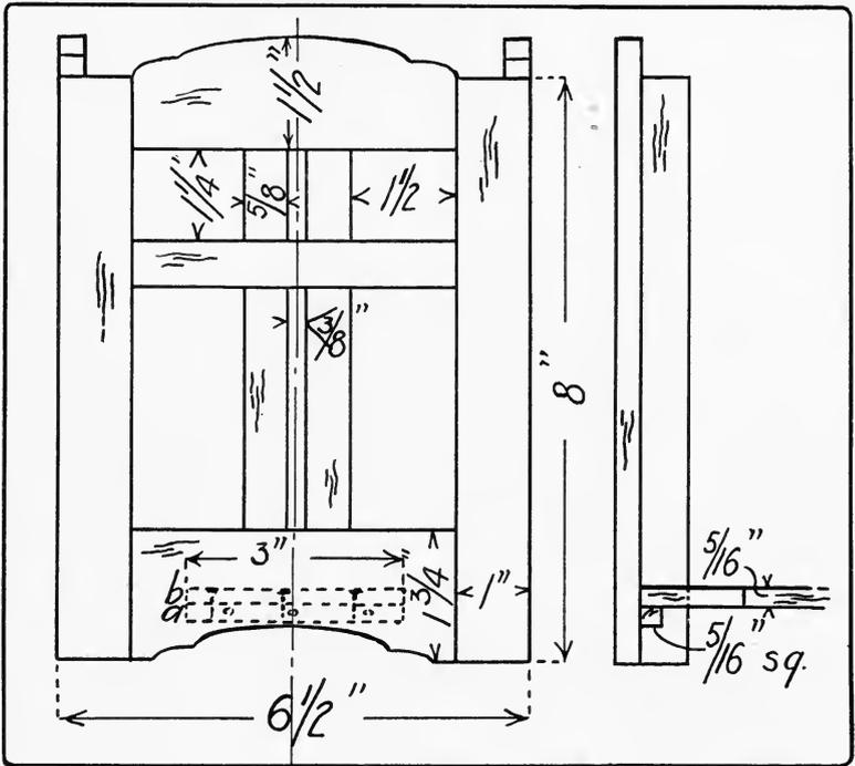
Fig. 201. Working drawing of lantern shown in Fig. 196.
