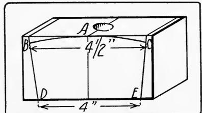
Fig. 158. Lay-out of sides of mallet-head.
