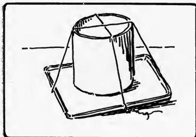
Fig. 112. Socket and pan wired together for soldering.
