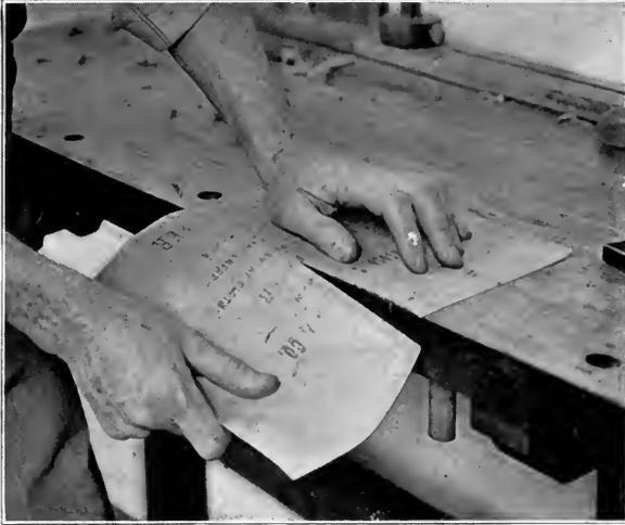
Fig. 37. Tearing sandpaper.
