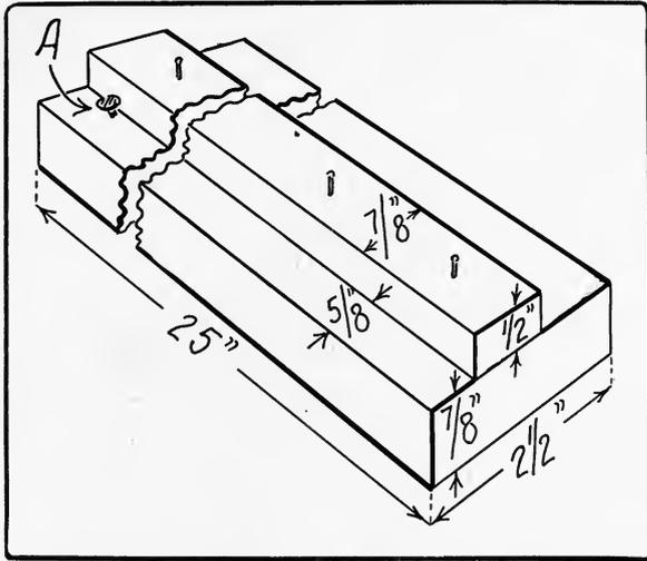
Fig. 77. Device for holding strips when rabbeting.
