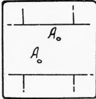
Fig. 104. Drill holes in pedestal for brads.
