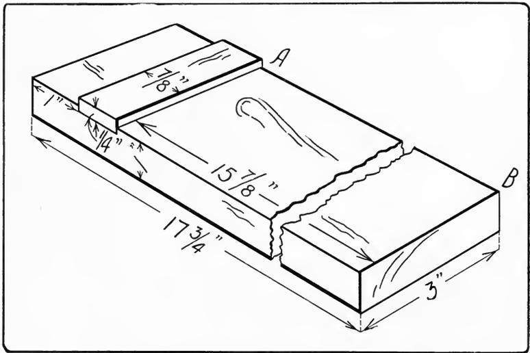
Fig. 31. Device for holding thin strips for planing.
