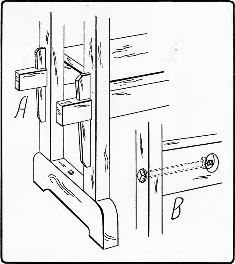
Fig. 6. *A*, Mortise and-tenon construction in frame of bench;
