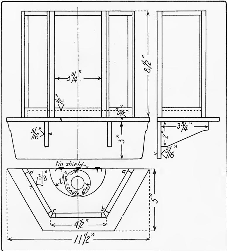
Fig. 202. Working drawing of lantern shown in Fig. 198.
