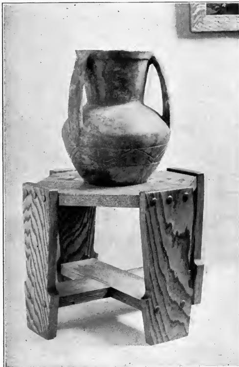
Fig. 142. Dowel ends covered with upholstery nails.
