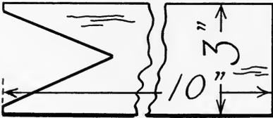
Fig. 116. Wood notched to hold copper while sawing.
