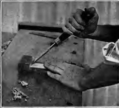
Fig. 41. Trimming a miter.
