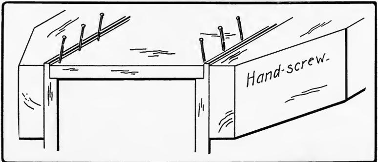
Fig. 189. Method of driving brads in box.
