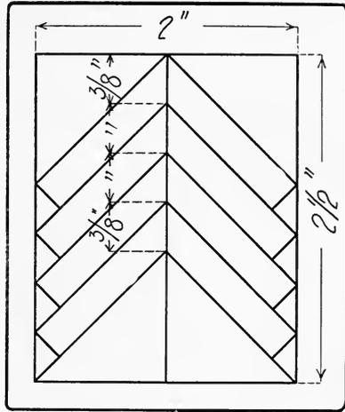
Fig. 43. Lay-out of the tin braces.
