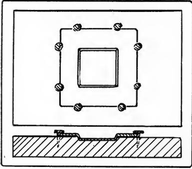
Fig. 119. Rim pan tacked down over mold.
