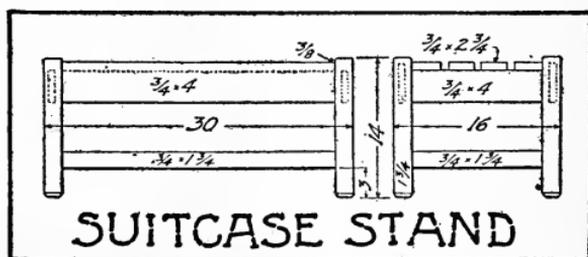
on the inside angles. It now remains to place on the four top slats, and the stand is ready for finishing. It can be stained any color desired, or left in its natural color, with a coat of filler thoroughly rubbed in and then wax applied.
