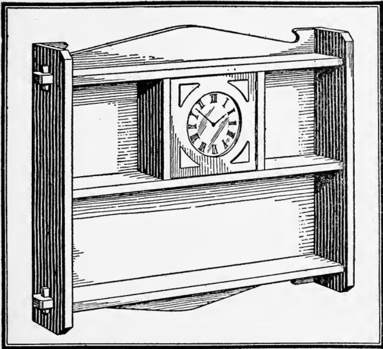
of both the top and bottom pieces will have to be notched out to fit in the backing. (See end view.) Fit the two ends and shelves together, then nail on backing, after which place the intermediate shelf. Work up curved strips at top and bottom from heavier material than backing and secure in place with nails set in from behind. The two vertical pieces that form the sides of the clock-case are now in order, after which the face should be fitted.
