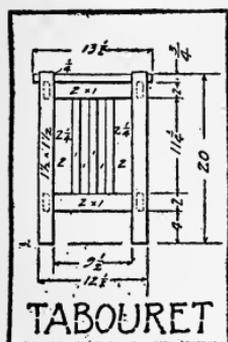
one-fourth by one inch need not be cut down, but should be let into the crosspieces full size for a distance of three-eighths of an inch. The two sides should be set up complete with glue, and clamped until dry, after which the remaining slats and crosspieces may be placed in position and glued. The top
