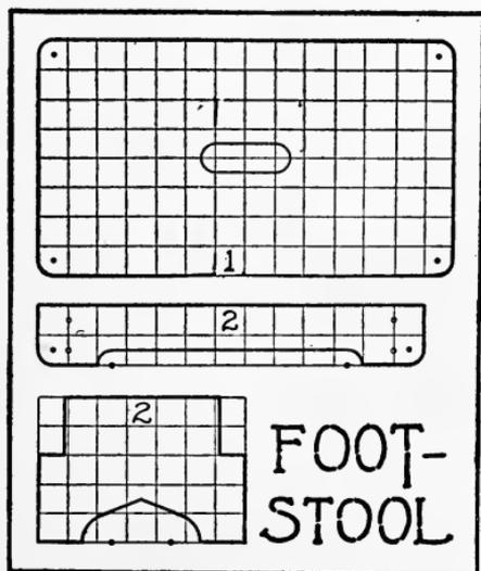
and saw out the wood in between, after which the edges should be worked smooth with sandpaper. Nail the sides to the two ends, and then fasten on the top. This may be done by nailing in through the top, or more neatly by screws put in from underneath from the inside at an angle.
