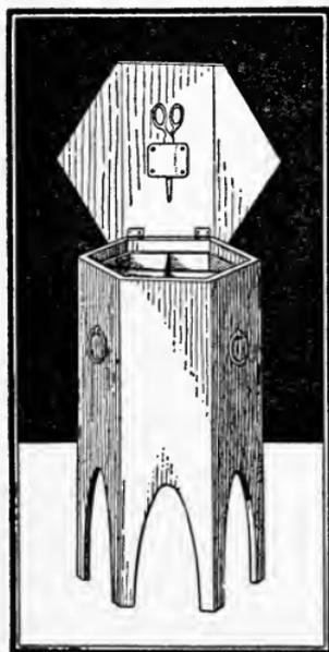
any difficulty is contemplated in assembling make a second hexagon to act as a temporary top. This latter will keep the side pieces in their proper relation while they are being fastened to the bottom and glued along the edges. Before assembling,
