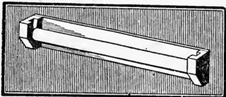
be about a half inch thick and twenty inches long, although this measurement may have to be changed a little if the toweling is of some special width. The shape of the end blocks is clearly shown in the drawing. A hole about a half or three-quarters of an inch in diameter is to be bored in the center half-way
