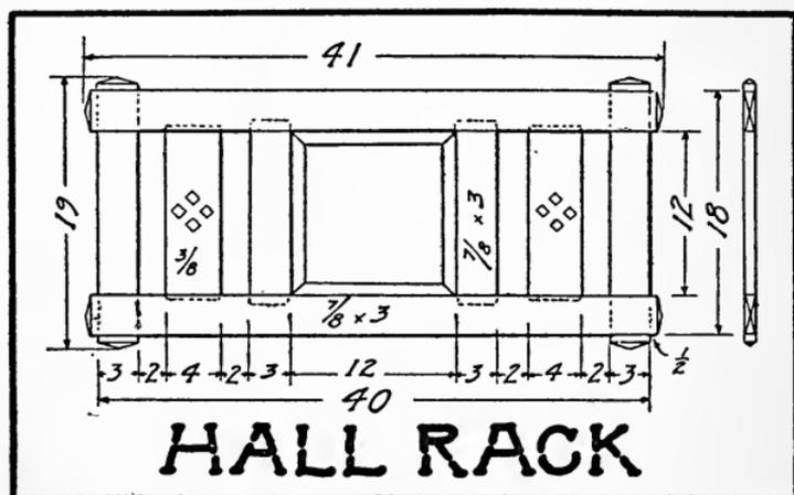
their respective mortises, after which the entire frame may be assembled. Use glue at all connections and clamp firmly until thoroughly dry. The mirror is held in place by notching out the back edges of the four pieces that surround it, so that it can be set in from the rear.
