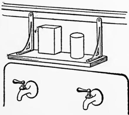
and a board on top, and the job is done. But supposing there is no room for brackets, as, for example, is usually the case over the kitchen sink,—what then? Just turn the brackets upside down and “hang” the shelf in place. If the place where
