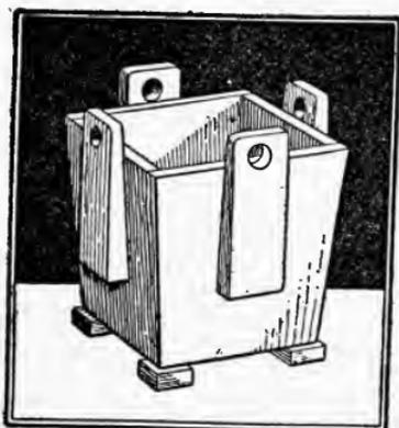
After studying the drawing you will notice that two of the side boards must be narrower than the other two, because they fit inside, just like the ends of any box. The only way to do, therefore, is to stand the
