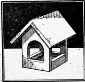
covering the ridge with a strip of zinc or tin. A small strip of wood should then be nailed on along each of the two sides to hold the nesting material in position.
