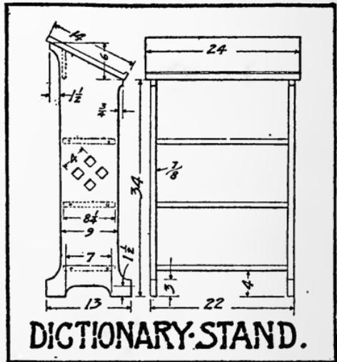
absolutely of a length and perfectly square on the ends, or in time the structure will surely work loose.
