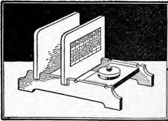
the compasses and then cut the wood exactly to line. The upright pieces are set into slots cut in the sides, so be sure that these slots are just large enough to make a tight fit. After the two sides are cut to line, place them together, sandpaper the edges flat and smooth, and hollow out the places for the pen and pencil. The two upright pieces require no attention aside from having their ends made smooth and the corners rounded. The last of the five pieces is for the ink pot, and should
