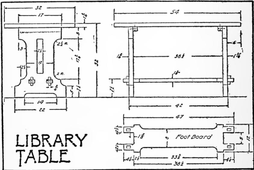
the under side with a strip of one-inch stuff and then covering with real or imitation leather. This arrangement has every appearance of a heavy top, and the large-headed brass or copper nails, which hold the leather on, give the edge an attractive appearance.
