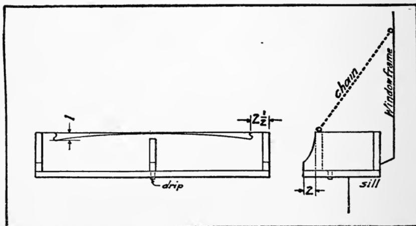
board near the front, to accommodate the drip spout, which should be soldered tightly to the zinc lining, and which should preferably extend a trifle
