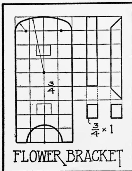
which case a more slender bracket would be appropriate. When a change, such as this, appears desirable, always mark out the lines of the new piece full size on a sheet of paper in order to be sure that it will look well.
