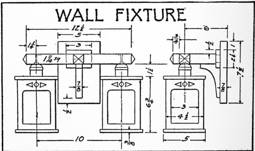
are now in order, the smaller one being mortised to match the central arm. The curved bracket remains to be shaped up, after which the whole may be put together, using glue and a few nails so placed as to be invisible. The completed wall
