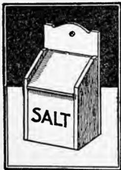
lift up and down easily without binding or leaving gaping seams at the sides. After rounding the back edge of the lid, set it in place and very carefully drive in a small nail through each side at the top corner into the lid so as to serve as a hinge. The place for these nails is indicated by the black spot on the pattern for the side, but do not drive the nails clear in
