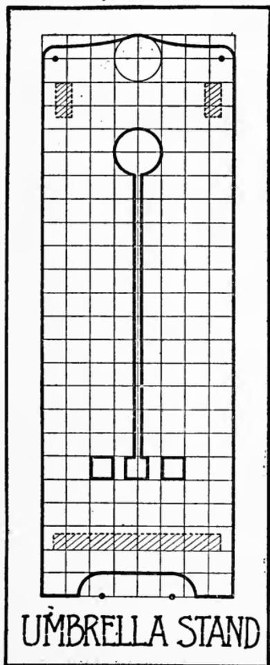
fectly square and flat on the ends. Mark off on the inner surface of each side board just where the other pieces are to be fastened. Fasten one of the sides to the bottom, and then nail on the cross pieces, after which turn over and put on the other side.
