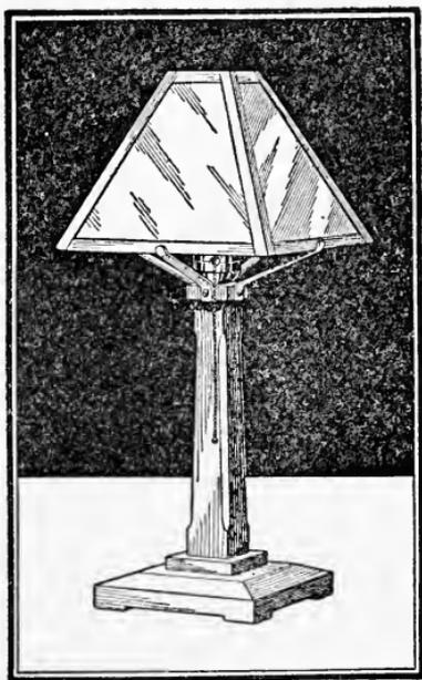
the same size as the one in the standard and another in through one side about the size of a lead pencil to connect therewith. At each corner on the underside glue on a small block one inch square and a quarter of an inch thick. The block on top of the base is next to be prepared with a square hole in the center to match the bottom of the standard. Fasten this piece to the base with glue and a few
