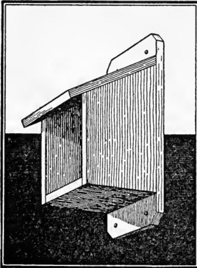
prefer to nest under the eaves, and require nothing more than a little nook or corner. The accompanying sketches illustrate a suitable form of nesting shelf, the construction of which is very simple. If several of these are to be put up, make one or more with one side open as well as the front.
