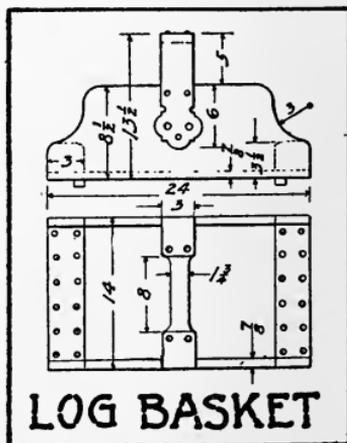
which each should be mortised or notched out so as to make a good connection with the handle uprights, which are now in order. As soon as the top piece is shaped up so as to afford a comfortable grip the whole may be put together and stained. The addition of the metal trimmings will complete the basket.
