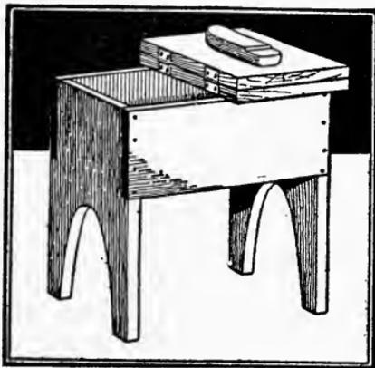
The working drawing clearly shows the method of laying out the end boards. These and all of the other pieces are made of inch lumber after it has been dressed smooth.
