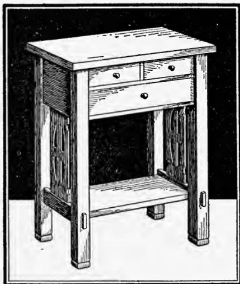
sure that nothing is on the floor to mar it.) Fasten each leg to the top with glue and three long screws set in at an angle. With very fine sand-paper go over the table and slightly remove the corners. When sand-papering the top and legs do not hold the paper in
