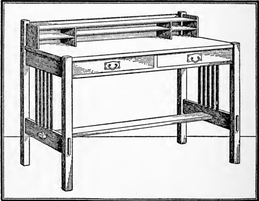
four-inch ones for the bottom crosspieces. The mortises at the upper ends should extend in for five-eighths of an inch. For holding the two ends and the back of the pigeonholes on top, mortise grooves one-half inch wide and three-eighths of an inch deep should be cut. Next proceed with the two bottom crosspieces, and tenon them on each end to fit the mortises already cut in the legs. These pieces
