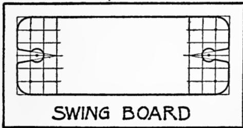
example to show that even in the making of the simplest things there is a right way and a wrong way. The usual way is to cut a V-shaped nick
