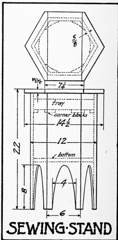
fit everything together, and provide means for clamping while the glue sets. To strengthen the side seams and to act as a support for the tray, make six little blocks as shown in the working drawing, and fasten them in place with glue and screws. The tray may be made as deep and in as many compartments as desired. The top is more apt to retain its shape if made of three pieces, fastened with glued tongue-and-groove connections.
