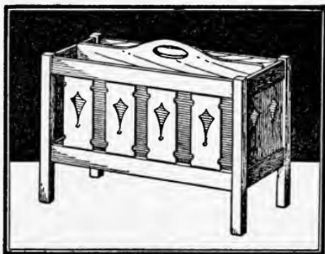
The accompanying design is very light, and the central division permits the paper to be placed on edge at either side,
