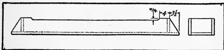
porch rail. A good substitute for the metallic lining consists of thoroughly coating and impregnating the inside and drip holes with heavy crude oil or tar residue, such as may be obtained from the gas works. Two or more applications should be given, after each of which the box should be placed in the sun until thoroughly dry.
