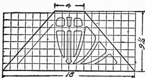
Quite the most difficult feature will be the construction of the shade. The dimensions of one of the four sections are given in the accompanying sketch. Accurately lay out the pattern on a sheet of paper and transfer it to each of the four pieces, which may be of several materials. If wood is used, the cross grain at the top and bottom must be reënforced with strips glued on the inside. Considerable care will be necessary in fitting the corner seams and in sawing out the pattern.
