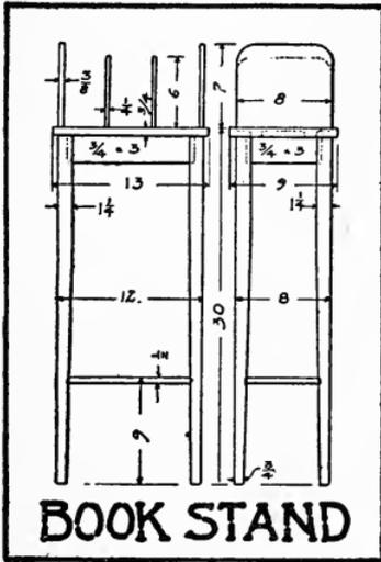
This piece is fastened to the legs by cutting off its corners slightly and then notching out the inner corners of the legs to match, all of which must be accurately done, or the legs will not stand parallel. You can now set up the whole with glue, and put in
