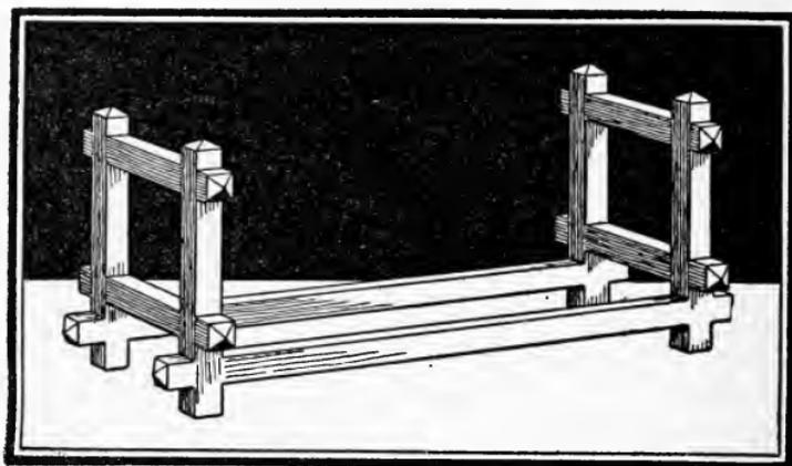
First cut the several pieces to the proper lengths and then point up the ends, taking due care that all
