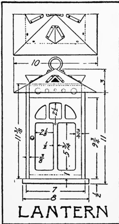
responds with the slope of the top. Lay out the pattern for the side openings, and after transferring it to the wood, proceed with the sawing. Finish all edges accurately and smoothly, and bore the vent holes near the top.
