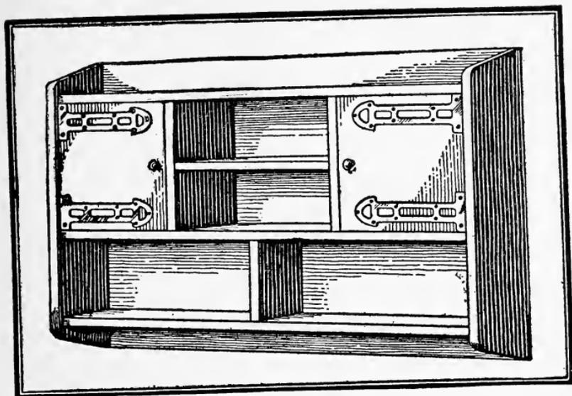
The construction is so simple that little need be said in this regard. The ends and shelves should first be made and connected, after which the back
