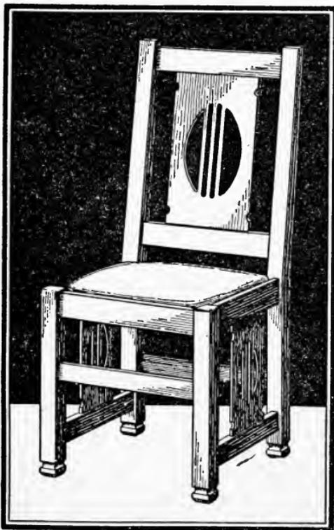
after which shape up the upper ends and feet. The front legs will now be made ready and similarly mortised, noting, of course, that the front crosspiece is placed higher than the rear one.
