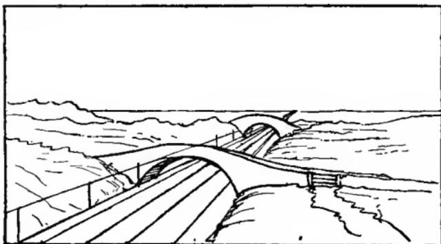
Vanishing points, for lines parallel to each other, and running away from spectator on a horizontal plane.
