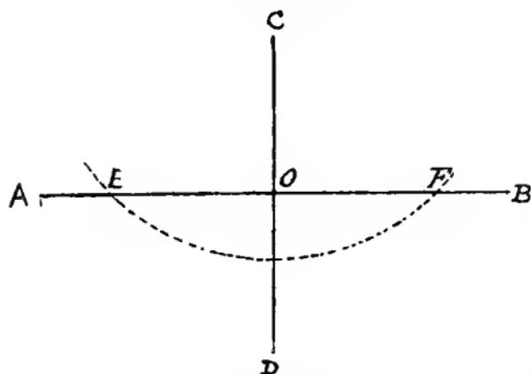
To find foci: with compasses take  $\frac{1}{2}$  long axis (A O); from point C or D make an arc cutting long axis in E and F. E and F are the foci; the points for the pins.
