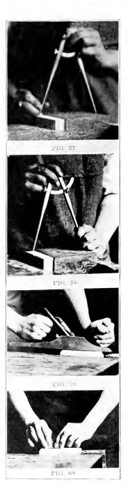
the  $\frac{1}{4}$ " lines and strike an arc. Do the same from the other  $\frac{1}{4}$ " line, Fig. 57. At the intersection of these arcs place one leg of the dividers and draw the bottom curve, Fig. 58. On the other end do the same.
