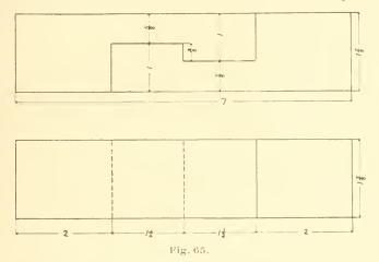
a good joint. Proceed in the following manner: Plane a piece to dimensions given, observing rules as in Exercise No. 1. Lay out end line and measure from that for the next line, as explained in Exercise No. 6. Measure from the first line for the distance to the third line. Square these lines around the piece, and repeat this operation on the opposite end of the piece. Next set the marking gauge at 5% inch and mark line as designated by A in Fig. 66 gauging from surface
