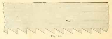
rectly across. The proper angle or rake for teeth of a rip saw may be determined by placing the try square on the points of the teeth, as shown in Fig. 21. The front side of the tooth should be at a right angle to the line of the points of the teeth; while in the crosscut, the test may be made by placing the try square on the back of the saw, as shown in
