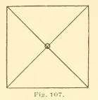
Intersection of these lines will be the center of the piece. At this point place the points of the lathecenters and adjust, so that the work will revolve easily. Tighten the binding screw on the tail-stock spindle and the work is ready to be turned. With the gouge take off the rough corners of the piece in
