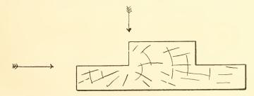
across the grain the fillister plane is best. This plane differs from the rabbet plane somewhat. The cutter is not set at a right angle to the plane, but is arranged obliquely across the bottom of the plane, thereby giving a skew cut. This is necessary to insure a smooth surface in cutting across the grain. It also has a spur or cutter projecting below the bot-
