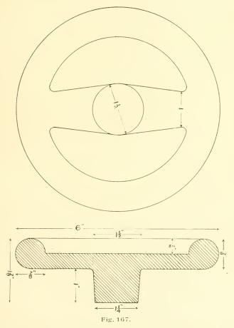
completed. The ring is 6 inches in diameter and 7/8 inch round. To construct the ring proceed in the following man-
