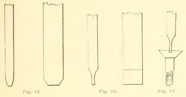
damage the head of the screw. The correctly fitted screwdriver and its position in the slot of the screw are shown in Fig. 17.
