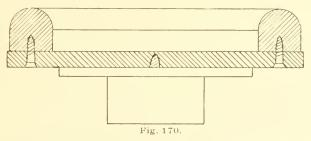
square edge scraping tool cut out the edge of disc until the center appears as in Fig. 171 and is of proper diameter
