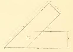
the joint is 45 degrees as shown in Fig. 58. The work of
