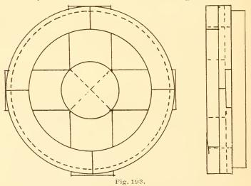
arms. Clamp together with a dog and small hand screw until dry. Place the piece on the lathe spindle and with the square edge scraping tool face off the rim until true, when it is ready for the next course or layer to be glued on. Dress one
