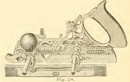
ient tool is the combination rabbet and fillister. This tool will perform the work of both. The plough plane is shown
