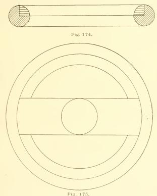
hub in its proper position. See Fig. 175. With the paring chisel and knife reduce the arms to an elliptical form, leaving fillets where the arms enter the ring. Sandpaper the arms,
