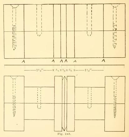
pins  $2\frac{1}{2}$  inches apart as shown by dotted lines in Fig. 182. Place the piece in the lathe and reduce to  $2\frac{3}{4}$  inches diameter. With the compasses mark lines on the piece as shown at A,
