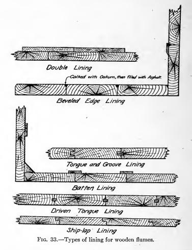
on the waterside of the lining, but they may be placed on the outside to favor the filling of the joints with sediment and to interfere less with the flow; in this position the floor battens are not exposed to the sun and are therefore less liable to warp.
