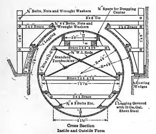
F1G. 72B.—Collapsible inside and outside forms for the construction of Anderson Siphon. Belle Fourche Project, S. D. which could be bolted together, and each part was small enough to pass through the erected form ahead of it (Fig. 72B).
