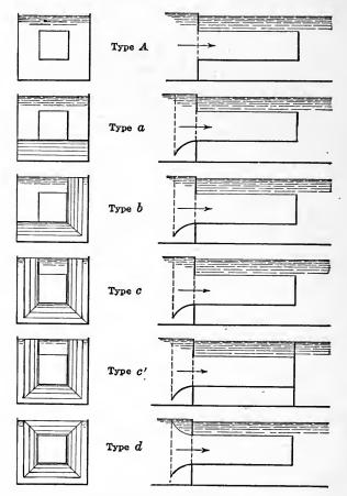
FIG. 12.—Forms of entrance of submerged tubes, 4 feet square, used in. experiments made at University of Wisconsin.
