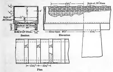
FIG. 47.-Reinforced concrete flume of Hamiz, Algeria.
