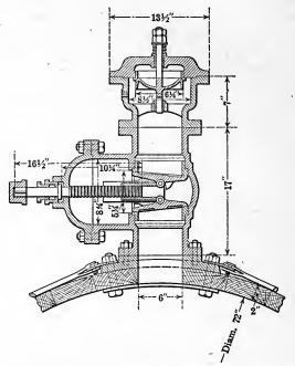
FIG. 62.-Air valve used on pipe line of Pioneer Power Plant, Ogden, Utah.
