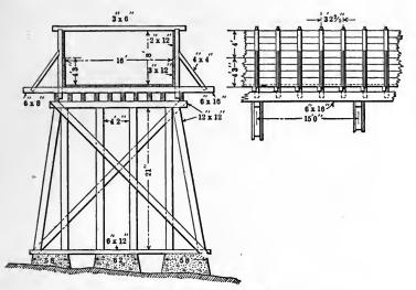
FIG. 35.—Flume of Kern River Power Co., Calif.
