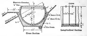
FIG. 24.-Reinforced concrete sectional lining. Tieton Project, Wash.
