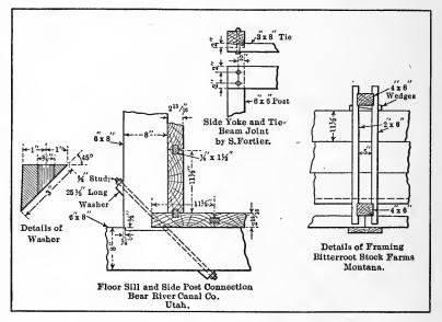
FIG. 38.—Details of framing for wooden flume box.
