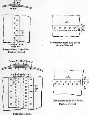
Butt Strap Joint Triple Riveted
