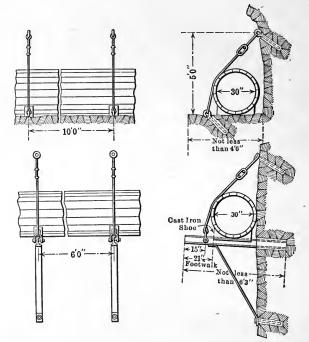
FIG. 68.—Method of supporting Canyon City pipe line on rock bench and vertical bluff. Colo.
