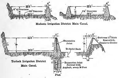
FIG. 28.-Concrete retaining wall, canal sections.
