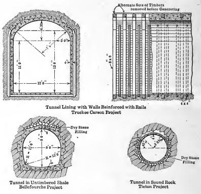
FIG. 26.—Tunnel cross sections.
