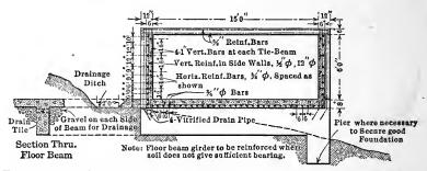
FIG. 31.—Reinforced concrete bench flume. Naches Power Canal, Wash.
