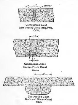
FIG. 20.—Contraction joints for concrete canal linings.
