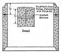
FIG. 70.—Contraction joint for handtamped cement pipe.
