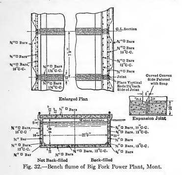
designed for an 8-foot depth of water. The floor is 12 inches thick, the side walls are 10 inches thick, and are designed as slabs supported at their lower end by the floor connection and at their upper end by the horizontal beam or coping, which is divided in lengths of 7 feet 9 inches by the tie beams, extending across the top of the flume.
