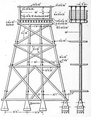
FIG. 34.—Delaney flume. Turlock main canal, Calif.
