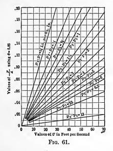
be calculated with the equations for flow of air through orifices. The accompanying diagram (Fig. 61) prepared by Enger and Seely gives the ratio of the area of the valve opening (F) to the cross-sectional area of the pipe A, for different values of U and various pressure differences  $(p_2 - p_1)$ . The diagram is based on a coefficient of discharge through the air inlet valve equal to 0.85.
