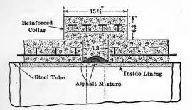
Section of Joint FIG. 75.—Joint of pipes for Sosa Siphon.
