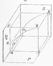
When a line A B (Fig. 34) is entirely included within one of the planes of projection P, it is confounded with its projection in that plane, and is projected on the other planes in  $a'b', a_rb_r$ , along the ground line in each plane.
