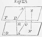
lel when they are so placed that they cannot meet, even if infinitely prolonged. Their lines of intersection, A B and C D, made by a third plane, R, are parallel lines. distance between two parallel planes is measured by any perpendicular, such as E F, drawn from one to the other.
