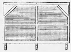
pattern. It appears clumsy in the picture, but the frame being made of oval iron, when covered with patent leather, produces a very strong and handsome article for light vehicles.
