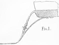
where the step is secured to the concave rocker by wood screws very effectively.
