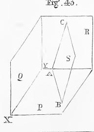
First the solid angles are projected, then the lines of intersection of the surfaces; the projections thus obtained are
