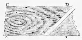
By the help of a mitre square, and a pair of compasses, to square the end of a plank:—Let A, B, C, D be a board of which we wish to make the end square at D, B. Having made the edge A B perfectly straight, assume any point (B, for instance) from which we are required to cut the end square, open the compasses any
