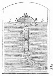
In the diagram, g is a flexible hose of India rubber or other suitable material, extending from the top to the bottom of the can or barrel; the lower end of which is attached to a faucet in the side, allowing nothing to pass which does not first enter the top of the hose, kept in position by a float. f is a short open pipe of thin copper, tied to the upper end of the hose, keep-
