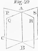
determined by those of three points not in a straight line. Suppose A and B (fig. 20) to be two of those points; a plane merely compelled to pass by A and B could occupy an infinite number of positions, P, Q, R, S, in space, by revolving round the line, A B, that joins the two points, A, B; but if the plane is forced to pass by a third point, C, placed outside of the line A B, its position becomes definitely determined, and the plane P is
