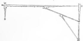
the same manner as those used for coaches, the side-plates running back of the point where the stay strikes the perch in order to strengthen it. For a light buggy these stays are made of  $\frac{3}{8}$  or  $\frac{7}{16}$  round iron. These look much lighter and are stronger than oval.
