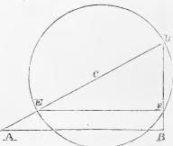
draw another line which shall be perpendicular or square to it.—Let A B be a given line, and D a point above it. It is required to draw a line from the point, D, that shall be perpendicular or square to A B. From D, draw any line, as D A, to cut AB; take
