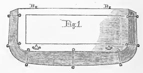
A A in Fig. 1 represent two one-inch check-loops screwed to the seat bottom, two inches from the back side and six and a half from the ends. B B represents two knobs, driven into the front of the seat, as in this instance, or may if chosen, be driven on top, hidden by the cushion. C C (Fig. 2) are two hard pieces of leather stitched upon
