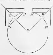
Now in order to show how this is done, let A B E F be the circle, and A D B the square. Having the blade A D equal in length to the stock B D, apply it, as shown in the figure, so that the ends meet the circle at the points A and B, and with a mitersquare draw a line in the direction D C, which will tend to
