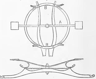
In each diagram A shows the transom stay—the first a bird's eye, and the second a vertical view—which can be raised or lowered to suit the height of the front of the body. In using this stay in place of wood, no furchells are required, the front and back stays being bolted on the fifth-wheel, as shown at B B.
