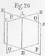
planes, intersecting each other in any manner by the edge A B, and again that the lines C D, E F, are perpendicular to that edge; those lines will Then measure the plane angles of the dihedral angles that are comprised respectively between the planes P P, Q Q. The angles, such as C A E, DAF, opposed by the edge, are equal. And again, the same angle, E A D or C A F, is their supplement (art. 15).
