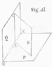
dicular to their com mon line of intersection. Suppose S (Fig. 41) to be a plane perpendicular to one of the two planes of projection to the horizontal plane P for instance, the trace A C of the plane S on the vertical plane Q is perpendicular to X Y. Consequently, the plane P, being perpendicular to the two planes Q and S, is perpendicular to their
