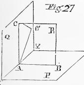
P and Q (fig. 27), is perpendicular to their common line of intersection, X Y, and reciprocally.
