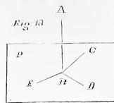
plane, P (fig. 18), when it forms right angles with all the lines, B C, B D, B E, bearing on the base of the plane. The line, A B, would be oblique to the plane if it did not fulfill this condition.
