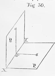
to their common line of intersection (Art.37). The lines a a ", a a " of the third plane with the two others are respectively equal and parallel to the projectants  $A\alpha'$  $\Lambda a$ , as forming the four sides of a rectangle. Moreover it can be supposed that the two projectants are transplaced parallel to their primitive position, each one following the direction of the
