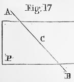
When a straight line, A B, has two points, A and C, within a plane, P (fig. 16), it is entirely within: this is a consequence of the definition of the plane (art. 9).
