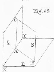
projection P and Q (Fig. 42), has its traces A B, A C, on each plane, oblique to their common line of intersection X Y. So that if one of its traces were perpendicular to the common line of intersection of the planes of intersection, for instance to that of the vertical plane, the plane S would then be perpendicular to the horizontal plane(Art. 37), which is contrary to the hypothesis.
