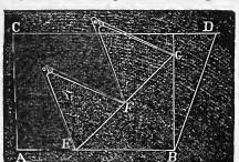
straight, open the compasses at any random distance, and placing one leg at A B, and the other at any point, as at F, in the direction B F, keep one leg at F, and turn the other round until it touches the edge
