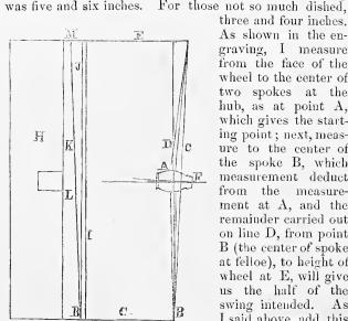
three and four inches. As shown in the engraving, I measure from the face of the wheel to the center of two spokes at the hub, as at point A, which gives the starting point; next, measure to the center of the spoke B, which measurement deduct from the measurement at A, and the remainder carried out on line D, from point B (the center of spoke at felloe), to height of wheel at E, will give us the half of the swing intended. As I said above, add this half of the swing—
