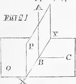
pendicular to a plane, Q, (fig. 21), is perpendicular to that plane. The line X Y, on which line two planes intersect each other, is their common line of intersection. In general, when two planes, P and Q, are perpendicular to each other, it is necessary that any line, A B or B C, drawn upon one plane, and perpendicular to their common line of intersection,
