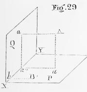
Suppose P and Q (Fig. 29) to be two planes of projection, the first horizontal and the second vertical, A is a point in space: if, from the point A, the perpendicular Aa and Aa' are drawn, the first on to the plane P, and the second on to the plane Q—the lower ends of the lines, a and a',
