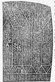
From the bottom line to the next (B), give  $\frac{5}{9}$  inch, and where springs are used, allow  $\frac{3}{4}$  of an inch fullness, as marked at D. Where no springs are used,  $\frac{1}{2}$  inch allowance will be amply sufficient, and  $1\frac{1}{2}$  inches for the diamond, E. Leave 5 inches from the top of the back for working.
