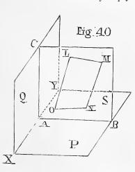
Suppose LMN O (Fig. 40) to be a perpendicular surface to the two planes P and Q, the plane S of that surface will cut the two planes P and Q by the lines A B, A C, which are styled the traces of the plane S on the two planes of projection. The surface being supposed perpendicular to the planes P and Q, the traces A B, A C, of the plane S on those planes, are perpen-
