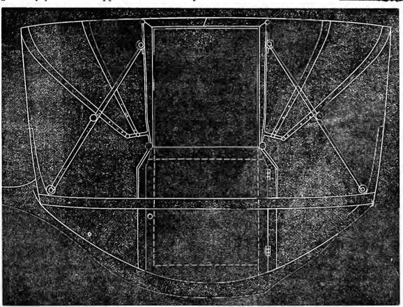
SKELETON OF A LANDAU SHOWING THE ARRANGEMENT OF THE BOWS. - HALF-INCH SCALE.
