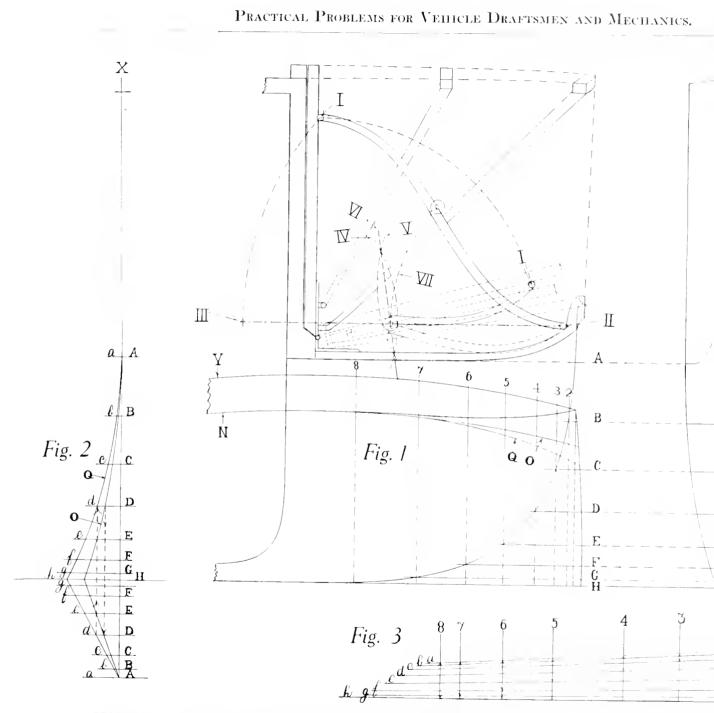
PRICKING OFF CORNER PILLAR ON TWISTED OR WINDING SURFACES OF A LANDAULET BODY W FOR LAYING OUT JOINT IRONS.
