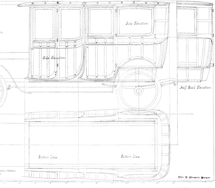
FIEL OF AN EXTENSION-FRONT BROUGHAM BODY, SHOWING SIDE ELEVATION, HALF FRONT AND HALF BACK ELEVATION AND BOTTOM VIEW.
