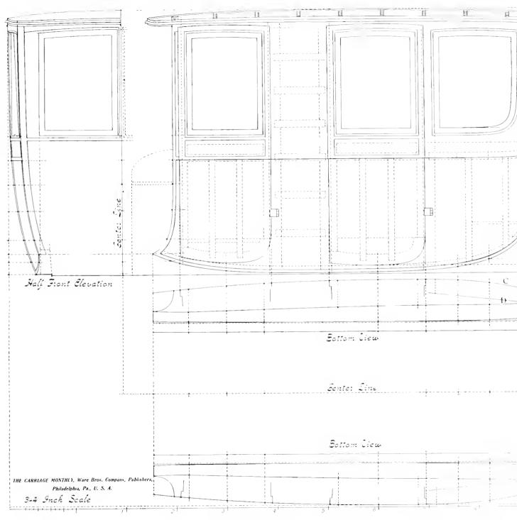
FOUR DOOR CLOSED LIMOUSINE BODY WITH REAR SQUARE CORNERS, FITTED TO A STR
