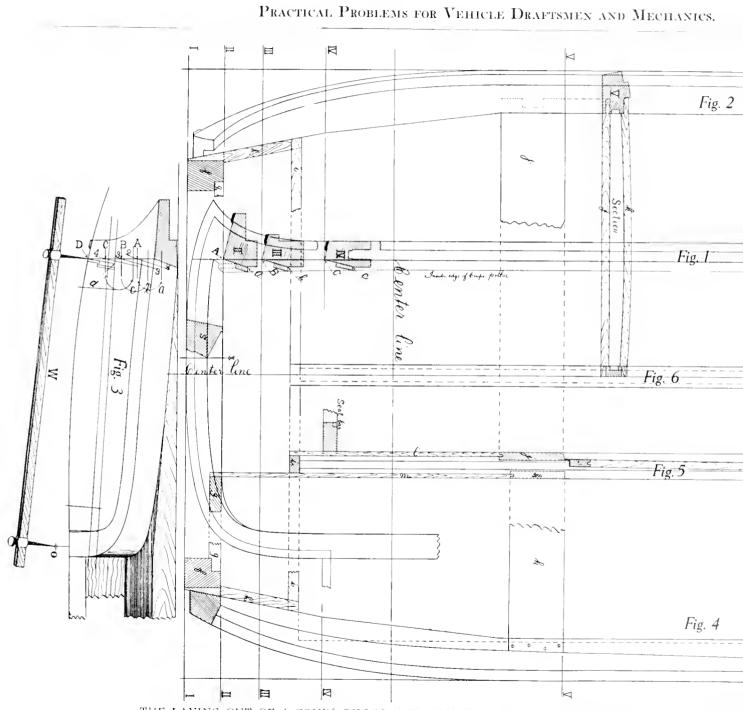
THE LAVING OUT OF A COUPÉ FILLAR AND CONSTRUCTION OF FORWARD PART OF AN ENCI
