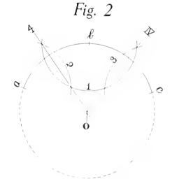
AN ARC FOR WHICH WE WISH TO FIND THE CENTER OR THE RADIUS.
