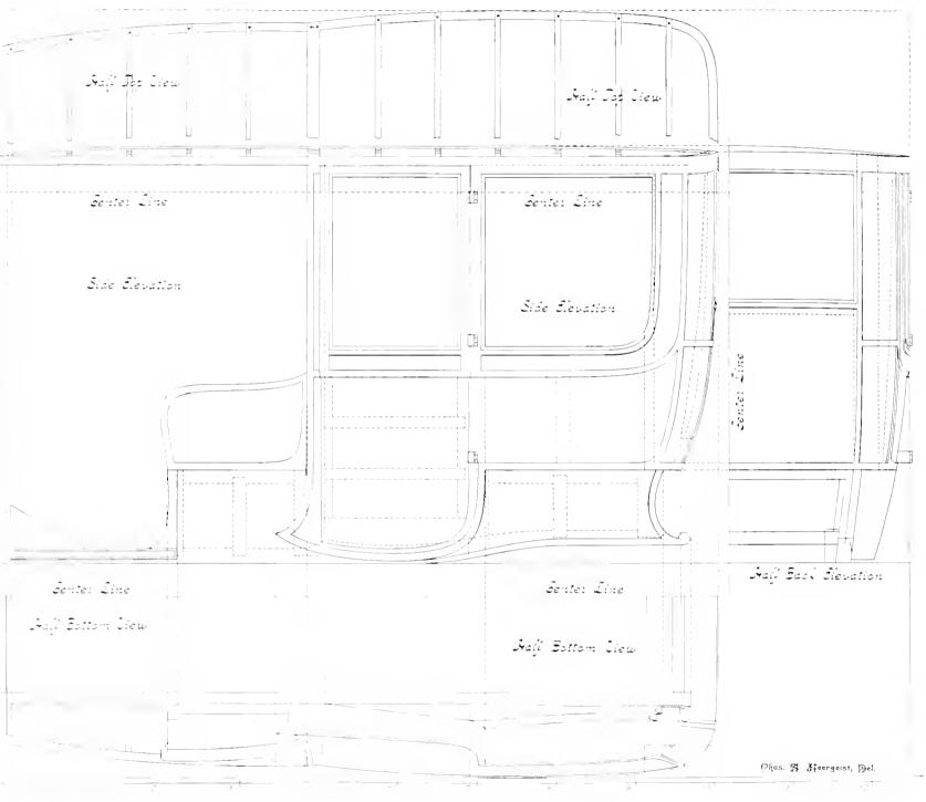
IN SIZE LIMOUSINE BODY WITH SOLID REAR CORNERS, FITTED TO A THREE-INCH DROP FRAME.
