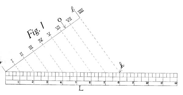
s to divide a line  $61\frac{1}{2}$  inches long into s. The easiest and quickest method is
