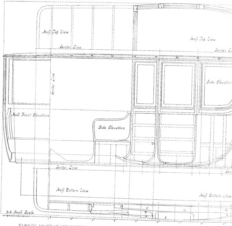
WORKING DRAFT OF LIMOUSINE BODY, WITH ENCLOSED FRONT AND ALL GLASS FRAMES TO DROP: ILLUST HALF FRONT AND HALF BACK ELEVATION AND BOTTOM VIEW.
