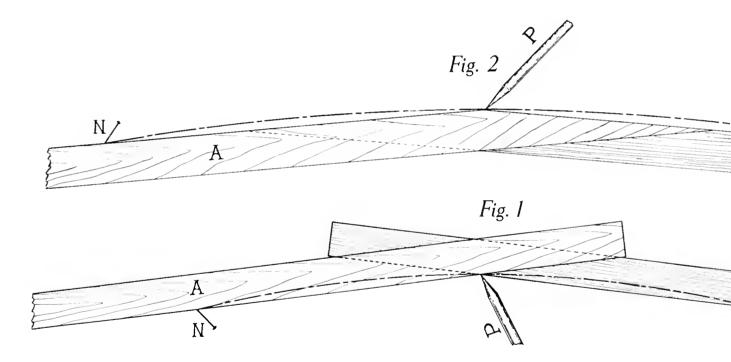
FOR laying out true sweeps or curves where it is impractical to strike the radius with the compasses or trammel points, we illustrate the following example, and although the principle has long been in use, it is unknown to a great many mechanics.
