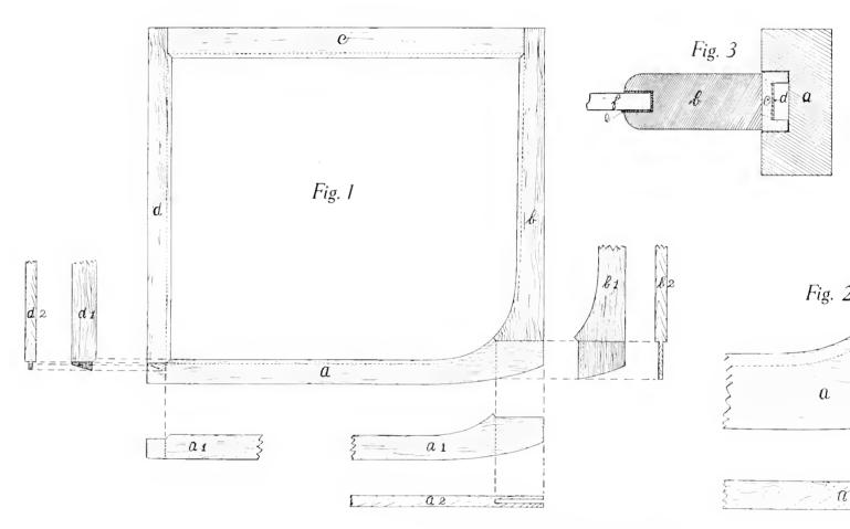
THE CONSTRUCTION OF GLASS FRAMES.
