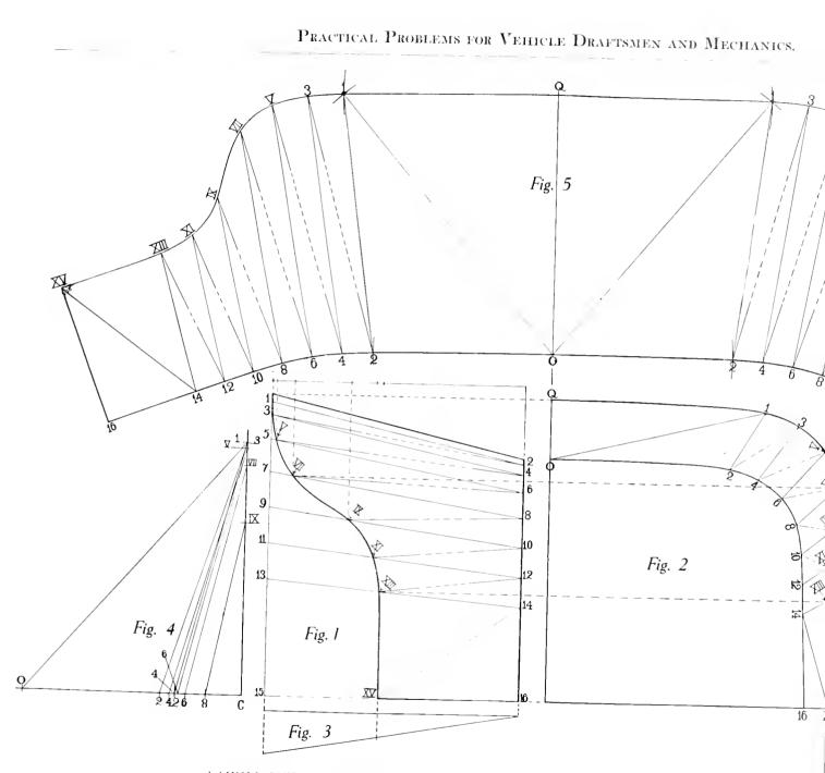
LAYING OUT PATTERN OF PANEL FOR A METAL SEAT BY THE SYSTEM OF TRIANGUL
