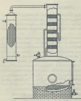
lighter constituents are removed and the distillate consists wholly of the heavier ones. That is, in the distillation of a crude turpentine from a pot still, the first part of the distillate is a fairly light product, containing relatively small proportions of heavy oils. This first portion is followed sooner or later, depending on the proportion of light oils in the crude oil and the speed of distillation, by a product containing continually increasing pro-
