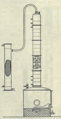
FIG. 2.—A periodic column still, with the chambers separated by hooded plates.
