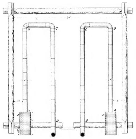
FIG. 9.—-Sketch showing the arrangement of furnaces and flues in a barn adapted for curing yellow tobacco; F, F, brick furnaces; A, B, C, D, sheet-iron flues.
