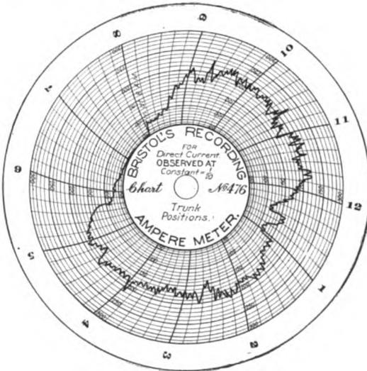
Fig. 166.— Automatic Load Line. Trunk Positions.
