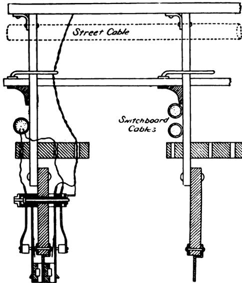
Fig. 12.—Section through Shelf of Distributing Board.
