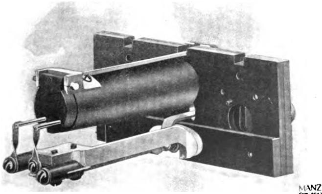
*Fig. 39.—Rear View Automatic Drop and Jack.*
