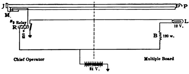
Fig. 114. — Testing Line to B Operator.
