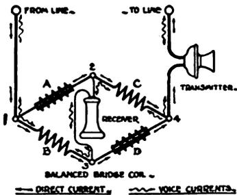
Fig. 86. — Wheatstone-Bridge Substation Circuit.
