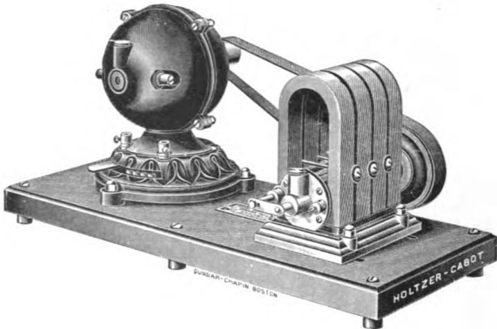
*Fig. 126. — Ringing Machine for Small Offices.*
