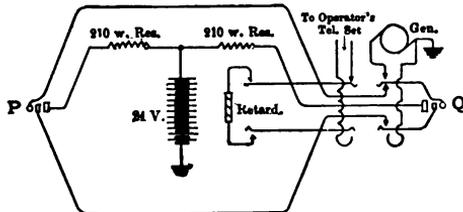
Fig. 144. — Connecting Cord Circuit.
