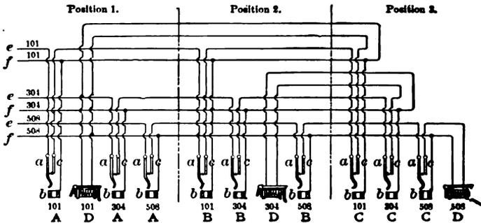
Fig. 60.—Series Multiple Board Circuit.
