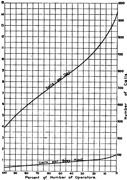
Fig. 160. — "A" Operator's Load.
