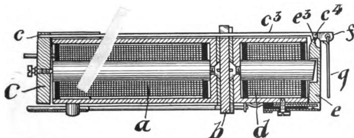
Fig. 64. — Self-restoring Drop.
