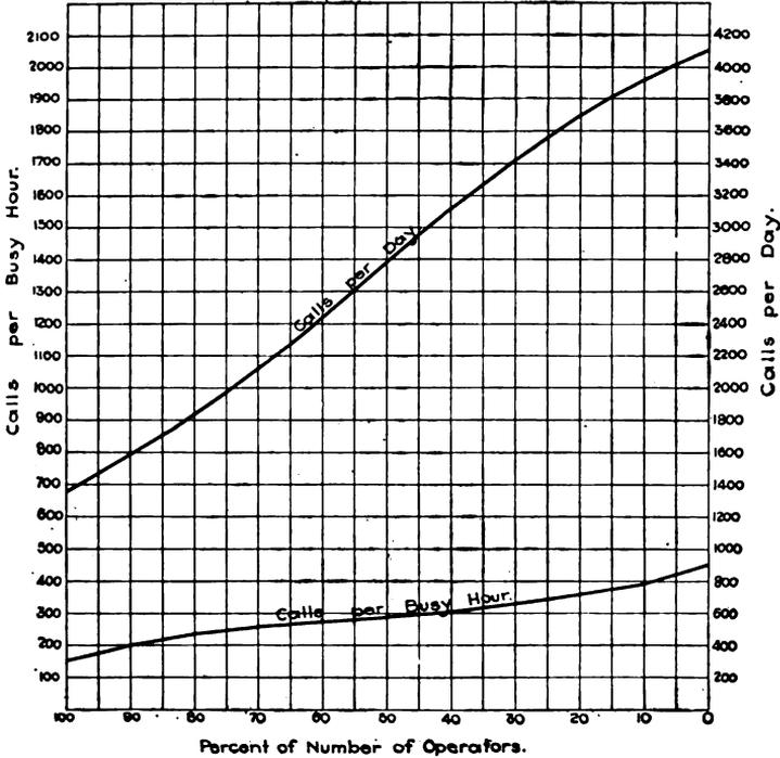
Fig. 162. — "B" Operator's Load.
