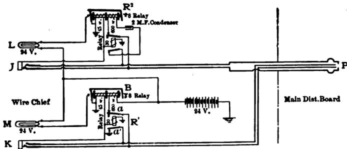
Fig. 145. — Testing Trunk to Main Distributing Board.
