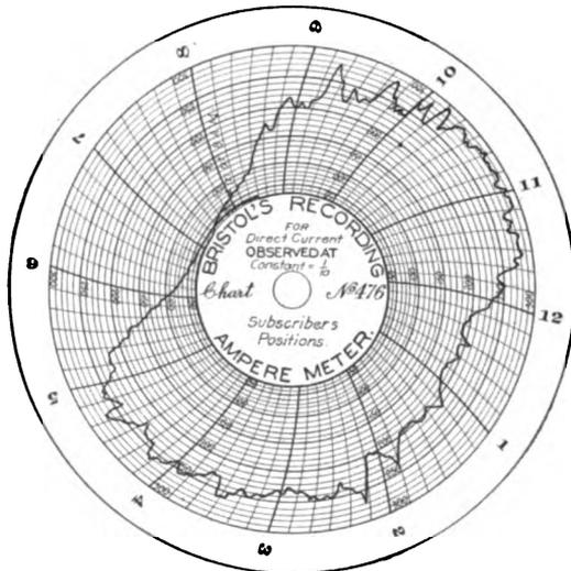
Fig. 167.—Automatic Load Line. Subscribers' Positions.
