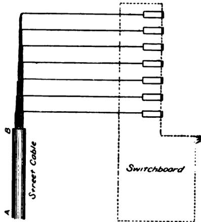
Fig. 5.—Diagram of Switchboard without Distributing Board.
