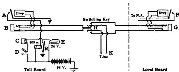
Fig. 118. — Circuit Toll Board to Local Board.
