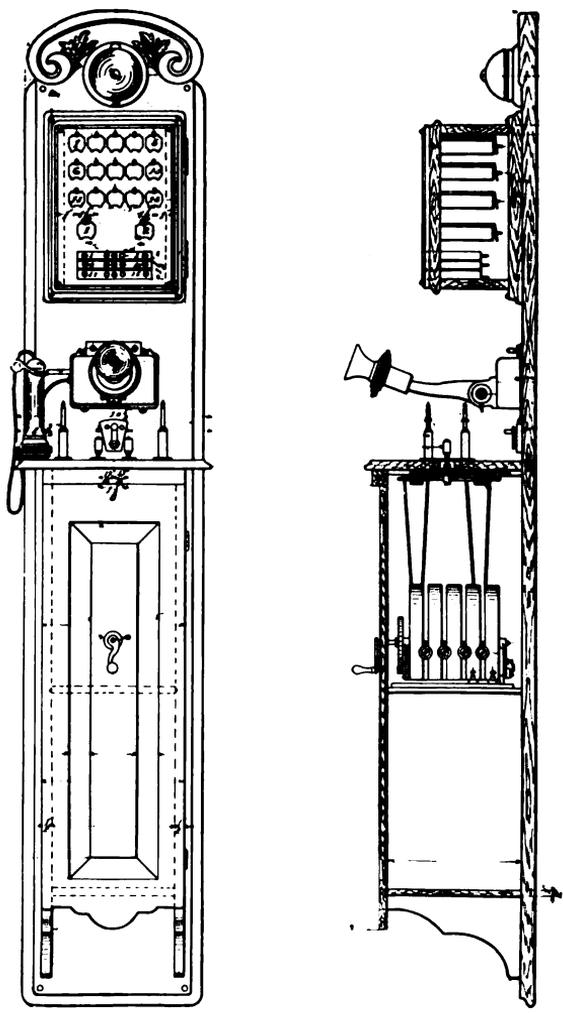
Fig. 40. — Rural Switchboard, Design No. 1.
