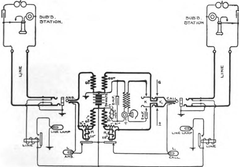
Fig. 56. — Non-Multiple Lamp Signal Switchboard Circuit.
