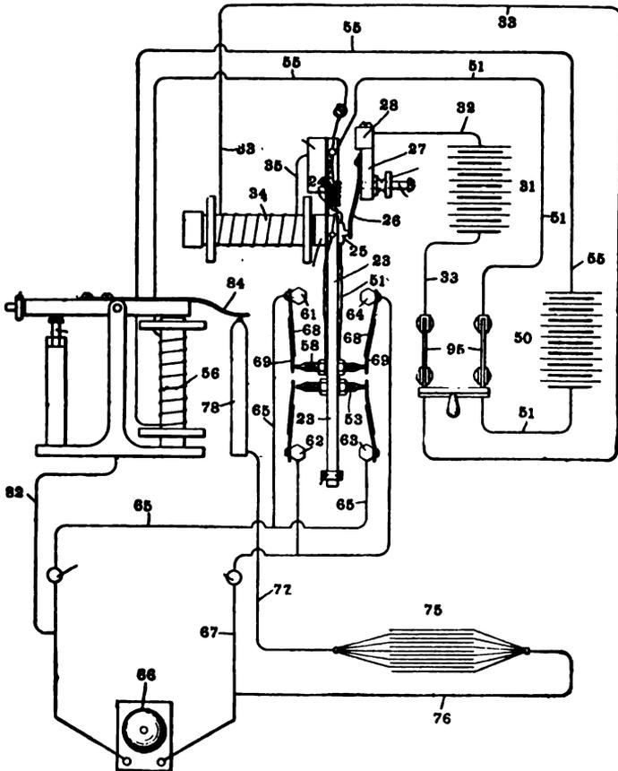
Fig. 138.— Circuit of Warner Pole Changer.
