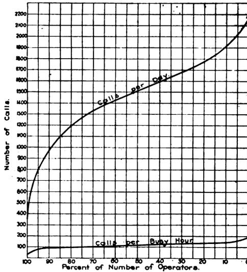
Fig. 158. — "A" Operator's Load.
