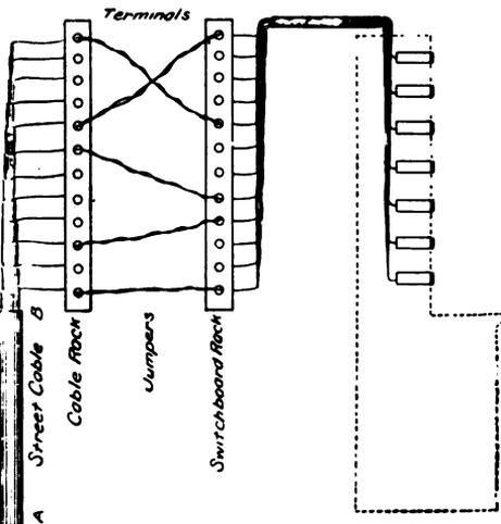
Fig. 6.—Diagram of Switchboard with Distributing Board.
