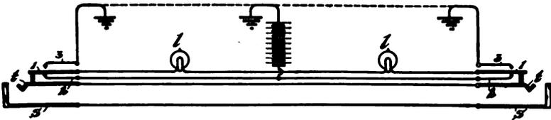
Fig. 58.—Simple Transfer Circuit.
