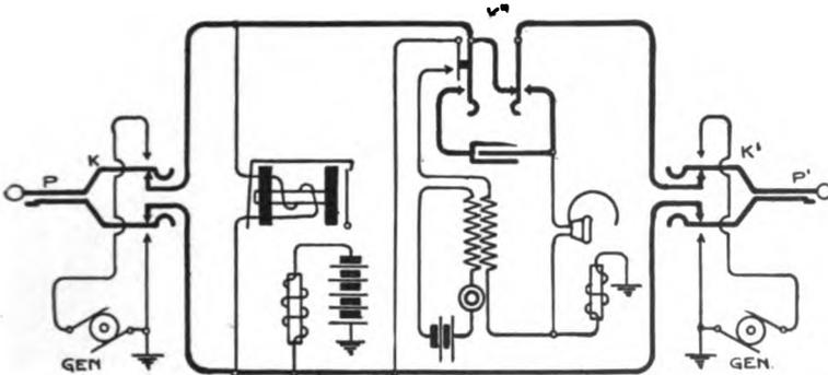
Fig. 61. — Cord Circuit Multiple Board.
