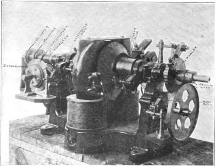
*Fig. 131. — Complete Ringing Machine. Howler End.*
