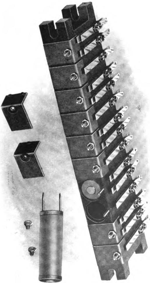
*Fig. 105. — Relays Mounted on a Strip.*
