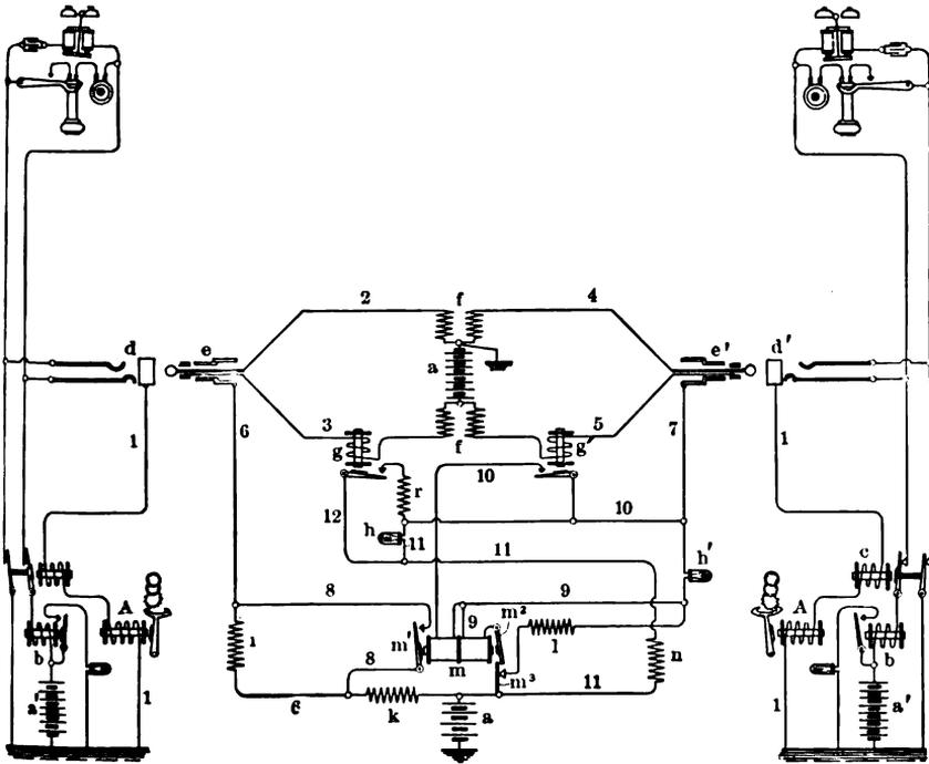
Fig. 109. — Meter Circuit Meter at Central Office.
