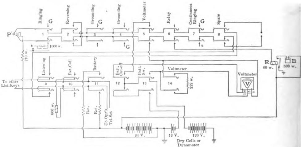
Fig. 147. — Testing Cord Circuit.
