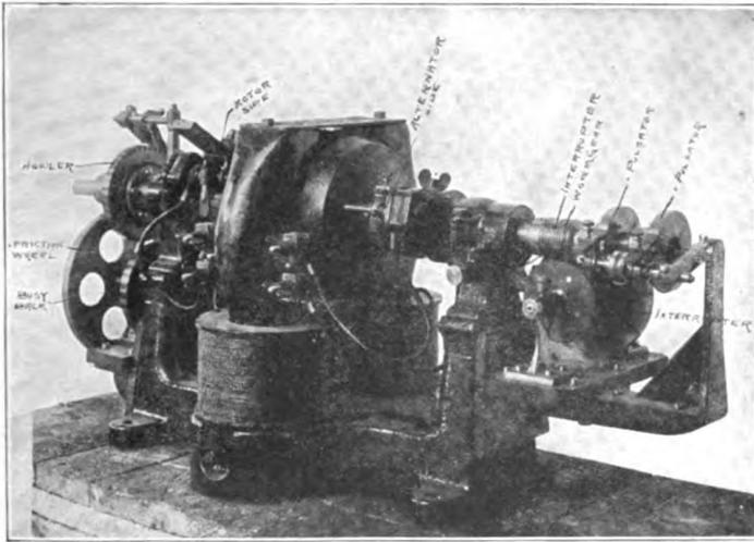
*Fig. 130. — Complete Ringing Machine. Pulsating End.*
