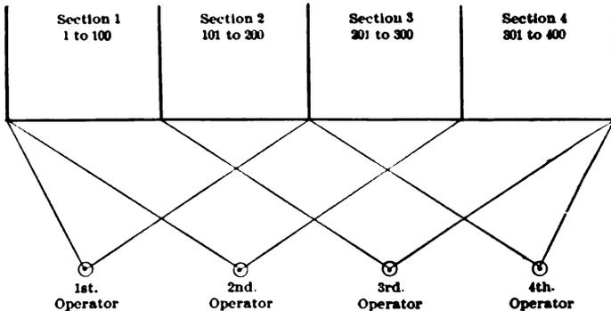
Fig. 59.—Diagram Illustrating Multiple Board.
