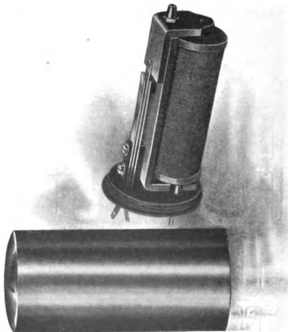
*Fig. 49.—Encased Relay.*
