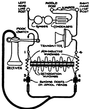
Fig. 87 — Wiring of Circuit of Fig. 80.
