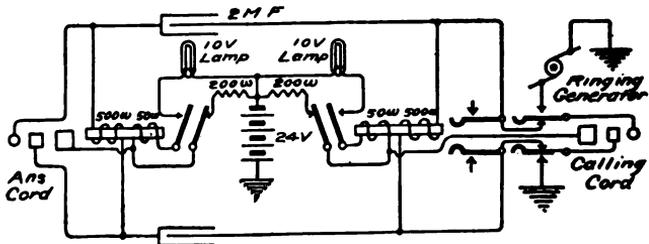
Fig. 57.—Circuits for Magneto Stations — Lamp Signal Switchboard.
