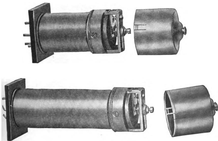
*Fig. 50. — Cap Covered Relay.*
