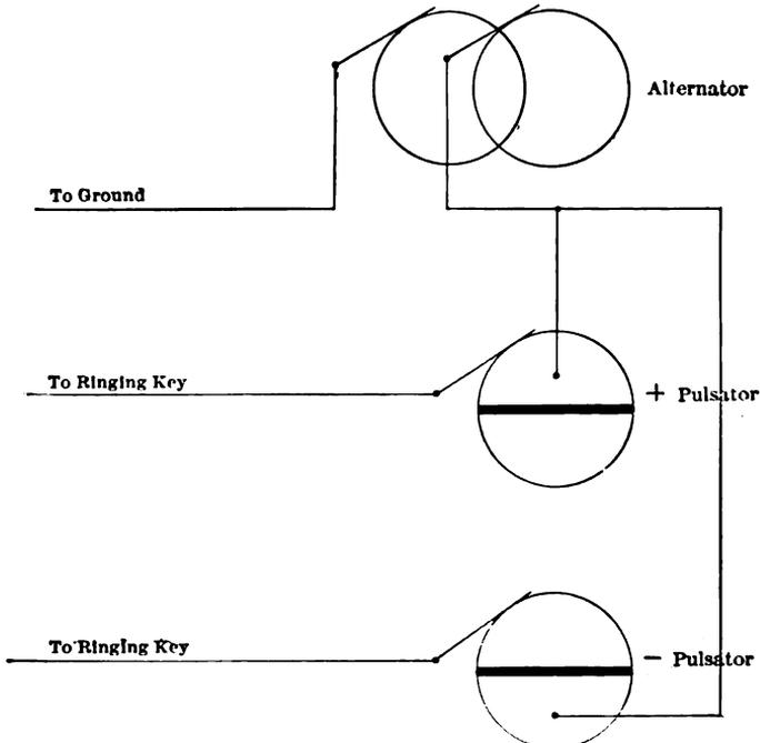
Fig. 132. — Pulsator Circuit.
