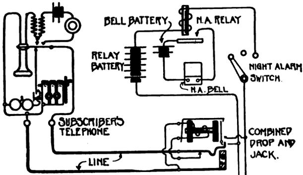
Fig. 20.—Simple Subscriber's Circuit.
