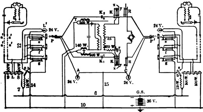
Fig. 79. — Jack Cut-off Common Battery Circuit.
