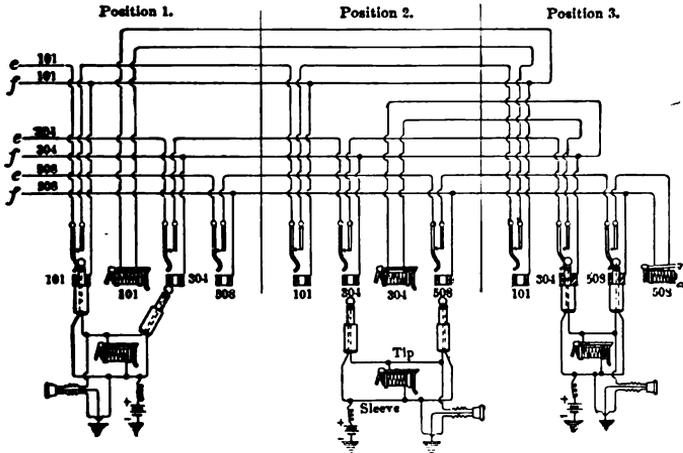
Fig. 62. — Busy Test Series Multiple Board.
