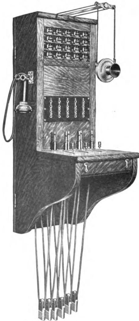
*Fig. 41.—Rural Switchboard, Design No. 2.*
