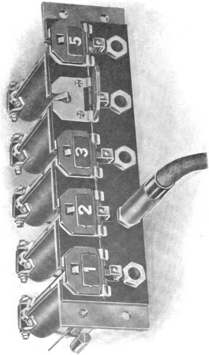
*Fig. 37. — Bank of Combined Drops and Jacks.*
