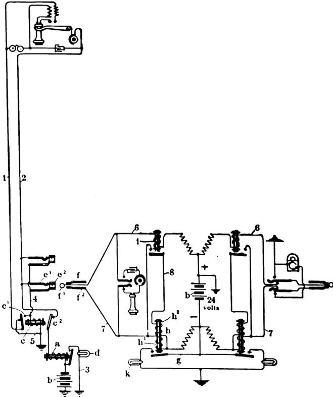
Fig. 77. — Two-wire Common Battery Circuit.
