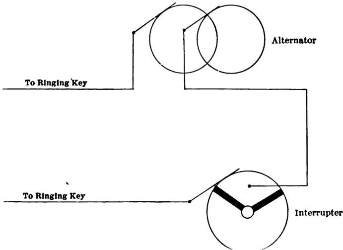
Fig. 133. — Interrupter Circuit.
