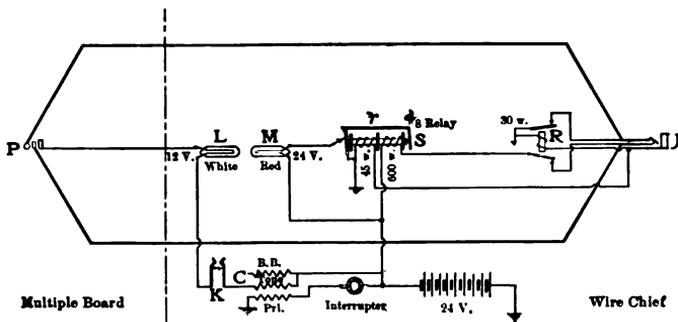
Fig. 146. — Testing Trunk to Multiple Board.
