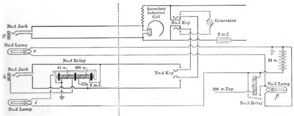
Fig. 115. — Listening and Pilot Circuits.
