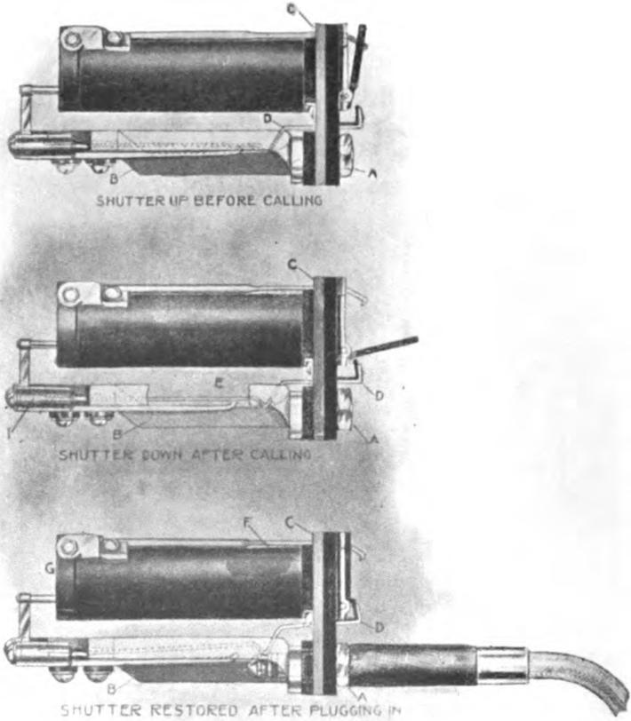
Fig. 38.—Sections of Mechanically Restoring Drop.
