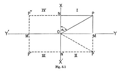
the position of P with reference to O. MP and NP, or ON and OM, are then called the *rectangular co-ordinates* of P and are usually written x and y. Thus, if P is defined as being 13,256 ft. north of OY and 27,450 ft. east of OX, we write:
