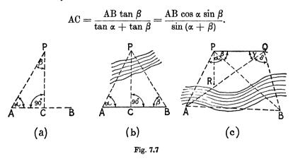
In fig. 7.7c, AB is inaccessible, but P is accessible. Choose an auxiliary point Q, measure PQ, and observe angles  $\alpha$ ,  $\beta$ ,  $\gamma$  and  $\delta$ . In triangle PAQ compute PA, and in triangle PQB compute PB. Then, in triangle PAB, PA, PB and  $\alpha$  are known, and angle PAB can be computed. Lay off point R such that  $\angle APR = 90^{\circ} - \angle PAB$ . Then R is a point on the perpendicular from P on AB. TRAVERSING
