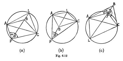
through A, B and C, the co-ordinates of P can be found if the angles  $APB = \alpha$  and  $BPC = \beta$  are observed. In figs. 6.12*a* and *b*, P is outside the triangle ABC, and in *c* it is inside it.
