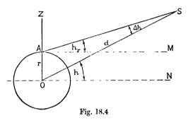
In fig. 18.4, O is the centre of the earth, A the place of observation on the earth's surface, Z the zenith at A, AM the horizon plane at A, and ON is parallel to AM. Then the observed altitude of the sun S from A, corrected for refraction and dislevelment, is the angle SAM =  $h_r$ , but, if S were observed from O, the observed altitude would be the angle SON = h. Then the angle ASO =  $\Delta h$  is the correction which must be applied to  $h_r$  to give h.
