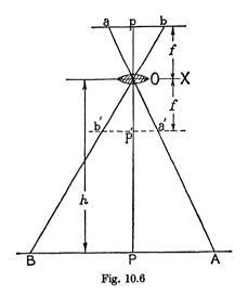
plate at **b** on BO produced. These points will therefore be the images of A and B, and their positions on the picture trace will be at **a'** and **b'**, where **b'p'a'** is parallel to **apb** at distance Op' = f below the lens. From the figure,
