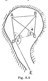
sides and diagonals measured. This provides sufficient data, as well as several checks, for the solution of the quadrilateral and for determining the bearing of the first leg, DE, of the traverse.
