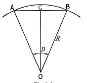
at the centre O of a circle of radius R. From O draw OC perpendicular to ACB. Then
