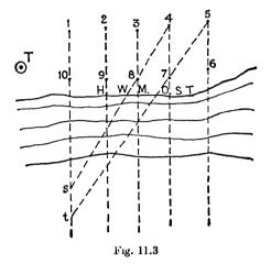
When sounding across rivers, the simplest way, if the stream is not too wide, is to stretch a rope across it between fixed points with marks
