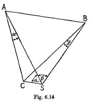
and ABC, but the fixing will be strengthened if we can get a value for ACB which depends on observation. To get such a value, set up the instrument at the satellite station S, as close as possible to C, measure the distance SC, and observe the angles  $ASC = \alpha$  and  $ASB = \beta$ .
