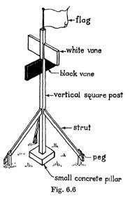
will be visible up to distances of two or three miles. If longer sights are involved, say up to about ten miles, a more solid signal, consisting of a solid wooden post 8-12 ft. high and with cross pieces as shown in fig. 6.6 makes a good signal.
