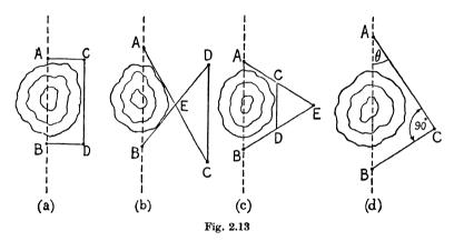
Case 1 (a).—In fig. 2.13a the line crosses a lake between A and B and the distance AB is required.
