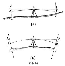
the two points. Similarly, a ray bent by refraction will be equally bent between A and B; hence the amount of bending observed on the staffs will be equal and will be cancelled when the difference of readings is taken.
