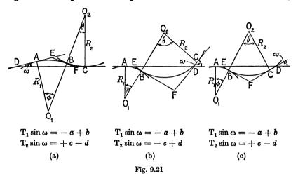
and the signs of the terms on the right in the expression for  $T_2 \sin \omega$ are reversed in the cases of fig. 9.21b. The signs of the terms are given under each diagram in which  $a = R_1$  versin  $\omega$ ,  $b = (R_1 + R_2)$  versin  $\theta$ ,  $c = (R_1 + R_2)$  versin  $\phi$ ,  $d = R_2$  versin  $\omega$ .
