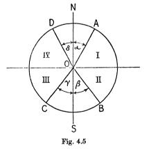
N $\delta$ W respectively. Magnetic compasses are often graduated on the quadrantal system, with the letters, N, E, S and W marked on the card or rim, and accordingly magnetic bearings are commonly booked and expressed in terms of reduced bearings, with the proper distinguishing letters before and after them to specify the quadrant.
