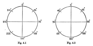
curves by means of small deflection angles, the second system, called the *half-circle* system, is the more convenient. In the whole-circle system, there need never be any doubt about how an angle is to be reckoned, but with the half-circle system it is important to note whether an angle is to be reckoned left or right of the zero mark, and this may lead to error unless great care is taken both in reading and booking.
