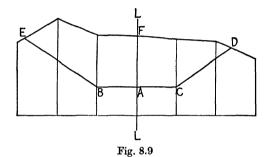
Fig. 8.9 is a cross-section used for taking out quantities during the construction of a railway. The line LL is the centre of the line, which here is in a cutting, the depth of cut being given by the line AF, where A is a point on the centre line at the proposed height of bottom of *formation*, or bottom of cutting, above datum.
