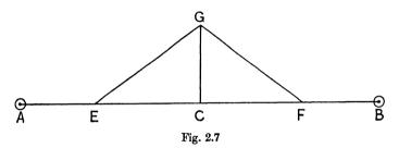
(fig. 2.7). Then, if the ends of the chain are held at E and F, an arrow is held at the centre of the chain, and the two lengths pulled equally taut, the arrow will be at a point G such that GC is at right angles to AB.
