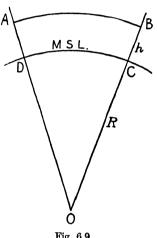
(M.S.L.). Once this is done, all lengths computed from the base through the triangulation will likewise be reduced automatically to mean sea-level.
