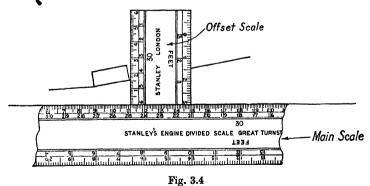
the graduated edges. The main scale is laid on the plan against the line from which the detail is to be plotted, and weights are put on the ends of the scale to hold it in position. The offset scale is placed alongside the main scale as shown in fig. 3.4, with one end against CHAIN SURVEYING
