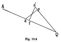
plotted on the plan, appear on the photograph. If only one point appears, join Q, the plotted position of O on the plan, to A, the plotted position of the fixed point, and on QA mark off Qf, fig. 10.4, equal in
