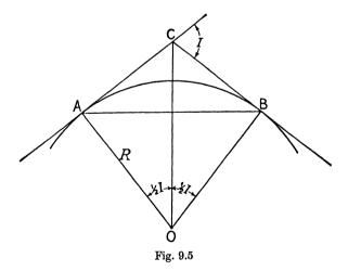
point of intersection of the tangents. Let C in fig. 9.5 be the point of intersection of the tangents, A and B the beginning and end of the curve of radius R, and I the angle of deflection, or intersection angle, of the tangents AC and BC. We need the distances CA and CB, which are called the *tangent lengths*, A and B being called the *tangent points*.
