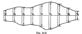
In other cases it is convenient to divide the central part of the figure into a series of triangles, as in fig. 12.3, and calculate the areas of the triangles, the areas of the small portions between the boundary and the sides of the triangles being taken out by the trapezoidal or by Simpson's rule. If ABCDEFGA is a closed traverse, the area included in it may also be calculated by co-ordinates by the rules given in Chapter V, p. 59.
