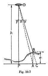
the point above datum, and is inversely proportional to the height of the lens. For points whose elevation is above datum, the displacement is radial outwards from the plate point of the photograph, and for points whose elevation is below datum it is radial towards the plate plumb point.
