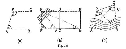
At points C and B on AB lay out CD and BE perpendicular to AB and equal to PF. Then D and E are points on the line through P parallel to AB. In fig. 7.8c, P is accessible, but AB inaccessible. Choose an auxiliary point Q, measure PQ, and observe angles  $\alpha$ ,  $\beta$ ,  $\gamma$  and  $\delta$ . From these compute angle PAB by using the triangles PAQ, PBQ and PAB in turn and lay off PC such that  $\angle APC = 180^{\circ} - \angle PAB$ . PC is then the parallel required.
