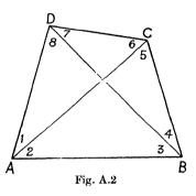
be a small difference between the two computed lengths and it is desired to "iron out" this difference as well as to make all three angles in each triangle add up to 180°. An approximate adjustment of the figure which does not require the use of the method of least squares may be obtained as follows:
