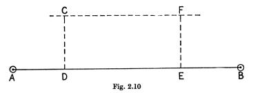
centre of the line. Having obtained the length of CD, use the arrows to put a mark at F so that CF = FD. Measure the distance EF and prolong the line to G so that FG = EF. Then the line CG is parallel to AB.
