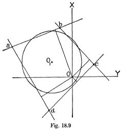
If several stars, say 4, are observed, this will give several position lines such as ab, bc, cd, da in fig 18.9, enclosing a figure abcda, inside which can be drawn the circle with centre  $O_1$  which most nearly touches all four lines. The rectangular co-ordinates of  $O_1$  with reference to O yield the quantities which, added algebraically to the assumed coordinates of O, give the most likely fix for the point of observation.
