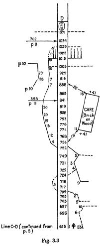
at chainage 718, with an offset of 9, and there are other offsets to it on the right at 729, 731 and 749 and to the left at 756, 768, 778, etc.
