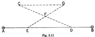
In the above case the point C is supposed to be accessible. If it is inaccessible, as in fig. 2.12, establish the foot D of the perpendicular CD on the line AB by the method described on p. 15 and obtain the distance DC by one of the methods described on pp. 17–18. A point F on the line CF can now be obtained by laying out EF perpendicular to AB and making EF equal in length to DC.
