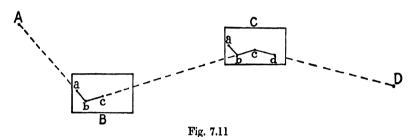
If the plan on the plane-table is on a very small scale, the plotted legs of the traverse will be very short, and hence there would be a very short length of line to lay the alidade against when orienting the table. Consequently, in order to avoid unnecessary errors, it is advisable in all cases to mark the directions of the various legs on the edge of the plan, so as to have reasonably long lengths against which the alidade can be laid when the table is being oriented at a new station.
