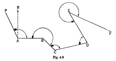
line is known, or can be observed, and the angle between each pair of lines has been measured. This is a practical problem which arises in the computation of every theodolite traverse.
