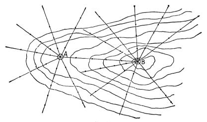
fixed by bearing and distance from the last point, and a similar series of radiating lines of spot heights observed. In this way, the ground is covered with a series of spot heights which, in turn, are plotted on the plan, and from these plotted heights the contours are interpolated.
