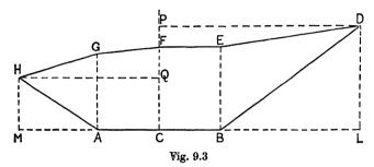
Continue the line AB right and left until it is intersected at the points M and L by the verticals HM and DL from H and D, and through H and D draw the horizontal lines HQ and DP to meet CF at Q and P. Then HQ = MC and DP = LC are the horizontal distances for the slope stakes at H and D from the centre line, and we see at once that
