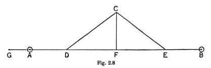
perpendicular to EC and DC respectively. Then line out a point H so that it lies on the intersection of the lines DF and EG. Finally, from H lay out HK perpendicular to AB. The line KH when produced should then pass through C, as should be verified by standing behind a pole at K and seeing if K, H and C are on one straight line.
