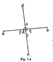
marks can then consist of ordinary wooden pegs, preferably creosoted, with tacks or nails driven in on top to mark the exact centre.
