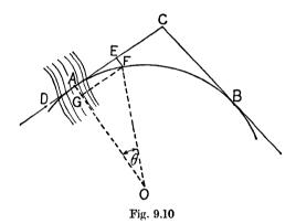
there. From G lay out GF = AG making angle  $CGF = 2\delta$ . This gives the point F on the curve. If the instrument is set up at F, and sighted on G, it will be aligned on the tangent at F and the curve can now be laid out in both directions from F.
