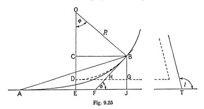
From O draw the perpendicular OE on the tangent AT and produce the circular curve in the direction of OE to meet OE at D. Through D draw DHG parallel to AT, meeting BF in H, and through B draw BC parallel to EF.
