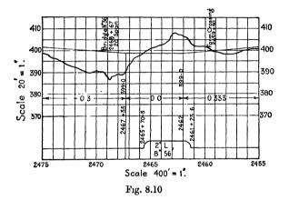
decided change in slope. These spot heights are plotted as a *longitudinal section* or *profile* which not only shows the general slope, rises and falls in the ground, but also the gradients which the bottom of the formation will follow.
