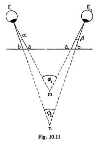
depth is lost for values of  $\alpha + \beta$ ,  $\phi_1$  or  $\phi_2$  less than about 20", the exact amount differing slightly with different observers.
