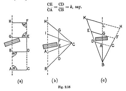
Set out points F and G in line with D and E and measure CF and CG. Produce CF and CG to I and H, making
