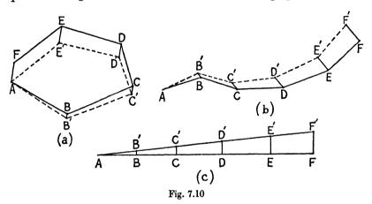
total length of the traverse, and at F draw the line FF' perpendicular to AF and proportional in length to the closing error at F. Join F' to A and on AF lay off the lengths AB, BC, CD, DE and EF proportional to the lengths of the different legs. Draw lines BB', CC', DD', EE' perpendicular to AF at B, C, D and E to meet AF' in B', C', D' and E'. Then the lengths of these perpendiculars represent the amount of the adjustment necessary at each point.
