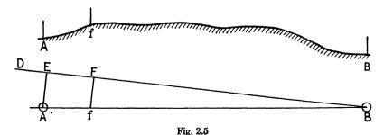
A from B as closely as possible, and range and chain a straight line BD in that direction, leaving intermediate numbered pegs along BD at the end of each chain length. From A lay out a line AE perpendicular to BD at E (p. 14) and measure the length of AE and the chainage of E. Then, points such as **f** can be found by drawing a perpendicular to BE at F and laying out Ff such that  $Ff = EA \cdot \frac{BF}{BE}$ .
