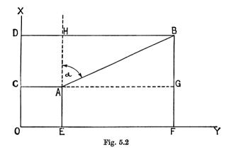
perpendicular to OX and OY, the angle BGA is a right angle. Also, the rectangular co-ordinates of A are  $OC = x_1$  and  $OE = y_1$ , and of B,  $OD = x_2$  and  $OF = y_2$ . Hence, in the right-angled triangle AGB,
