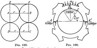
FIG. 189.—Area of an interspace bin. FIG. 190.—Moments due to grain in an interspace bin.
