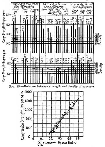
FIG. 16.-Relation between strength of concrete and cement space ratio.
