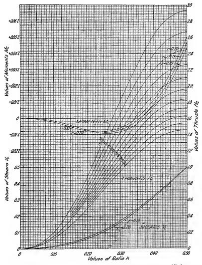
FIG. 59.—Influence lines for moments, thrusts and shears at crown; filled spandrel arch, type A<sub>2.5</sub>.
