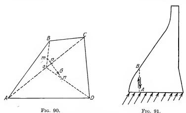
FIG. 91.--Shear stresses in a masonry dam.
