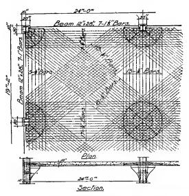
FIG. 36.—Reinforcement in a flat slab.
