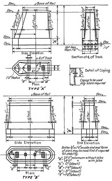
FIG. 143(A).-Standard mass bridge piers of C. M. & St. P. Ry.
