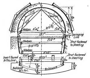
FIG. 212 .- Forms for a large concrete sewer.
