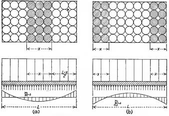
FIG. 192.-Moments in slab under a bin cluster.
