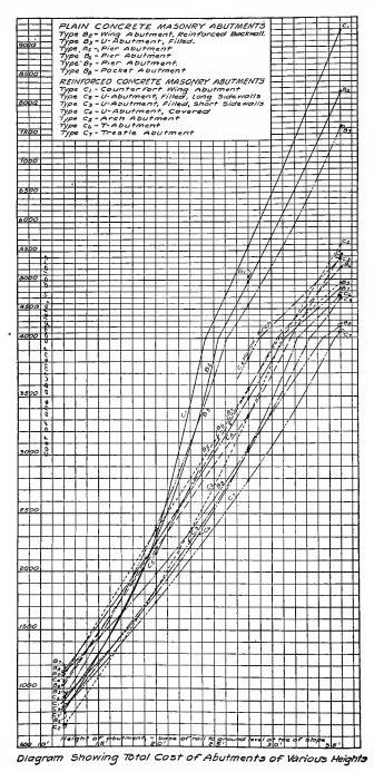
FIG. 140.-Relative costs of railway bridge abutments of various types.
