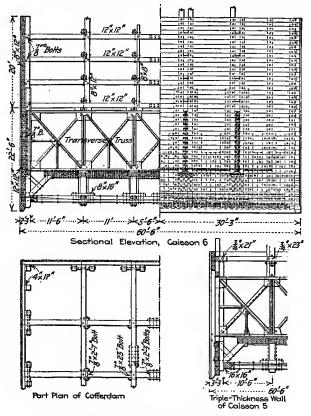
FIG. 255.-Details of the Metropolis bridge caisson.
