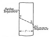
FIG. 196.-Temperature drop in a chimney wall.
