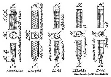
FIG. 238.—Details of reinforced concrete piles.
