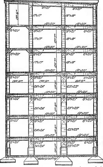
FIG. 33.-General arrangement of slabs supported on beams and girders.
