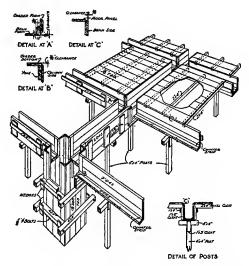
FIG. 206.-Beam and girder forms, bottom attached.
