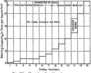
FIG. 221.-Chart for allowable soil pressures.
