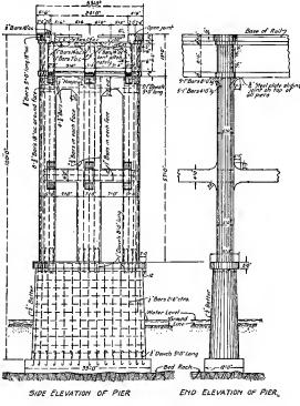
FIG. 146.-Divided reinforced concrete pier.
