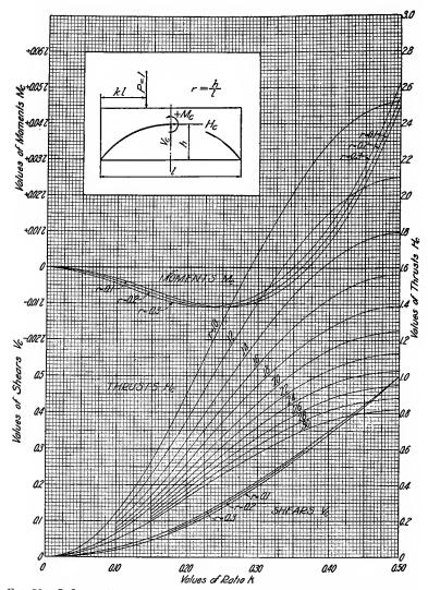
Fig. 52.—Influence lines for moments, thrusts and shears at crown; open spandrel arch, type  $A_{1,\delta}$ .
