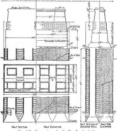
FIG. 247.-Open caisson for the New London bridge.
