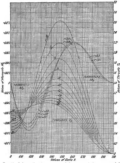
FIG. 56.—Influence lines for moments and thrusts at springing; open spandrel arch, type A<sub>2.0</sub>.
