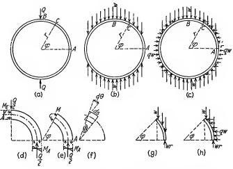
FIG. 176.—Stresses in a pipe conduit due to external loads.
