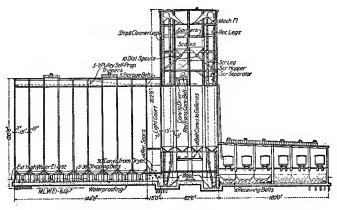
FIG. 193.-Section through Girard Point grain elevator.
