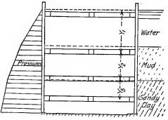
FIG. 245.-External pressures on a cofferdam.
