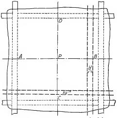
FIG. 35.-Two-way reinforcement in slabs.
