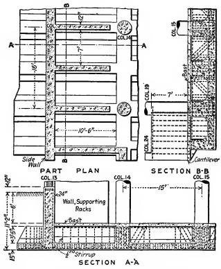
FIG. 229.—Floating foundation under the Felt & Tarrant Building.
