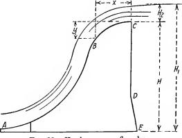
FIG. 82.-Head on an overflow dam.
