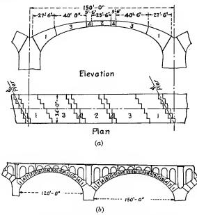
FIG. 69.—Order of placing masonry in arch rings.
