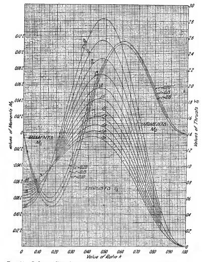
Fig. 63.—Influence lines for moments and thrusts at springing; filled spandrel arch, type  $A_{3.0}$ .
