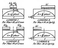
FIG. 44.—Position of live loads for maximum stresses.
