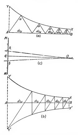
FIG. 48.—Dividing an arch ring by graphical methods to make  $\frac{ds}{t}$  constant.
