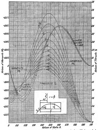
FIG. 61.—Influence lines for moments and thrusts at springing; filled spandrel arch, type A<sub>2.0</sub>.
