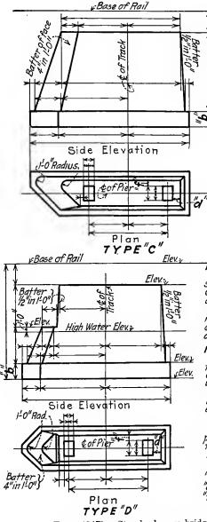
FIG. 143(B).-Standard mass bridge piers of C. M. & St. P. Ry.
