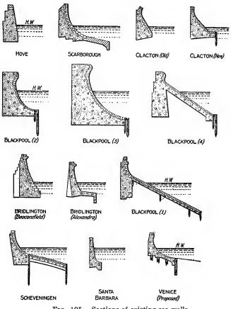
FIG. 105.—Sections of existing sea walls.
