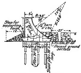
FIG. 106.—Section of sea wall at Galveston.
