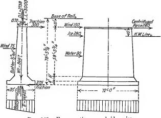
FIG. 142.—Forces acting on a bridge pier.
