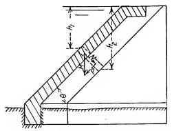
FIG. 98.-Stress distribution in a multiple arch dam.
