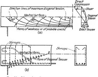
FIG. 28.—Diagonal tensile stress and reinforcement for same.
