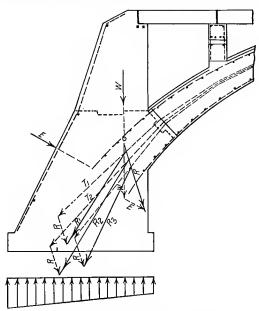
FIG. 70.-Forces acting on an arch abutment.
