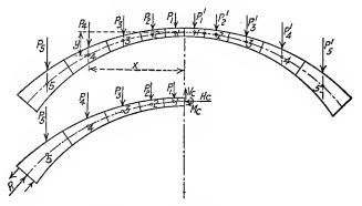
FIG. 46.-Loads and forces on an elastic arch ring.
