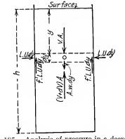
FIG. 185.—Analysis of pressure in a deep bin.
