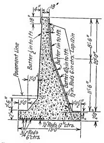
FIG. 123.—Section of a fillet retaining wall.
