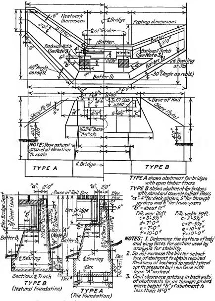
FIG. 136.—Standard bridge abutment of C. M. & St. P. Ry.
