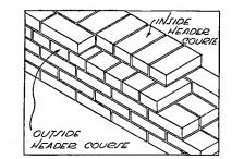
FIG. 7.-Manner of Laying Brick with Common Bond.
