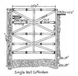
FIG. 241.-Internal framing of a timber cofferdam.
