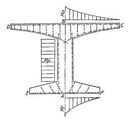
FIG. 168.—Distribution of moment in a cantilever unit.
