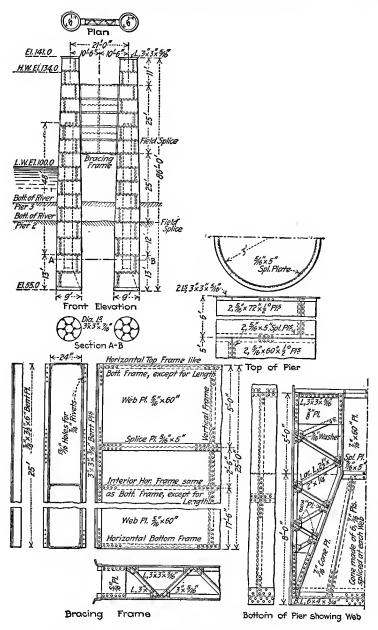
FIG. 249.—Pneumatic cylinders for bridge piers at Trail, B. C.
