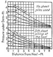
FIG. 83.-Hydrostatic pressure under a model dam.
