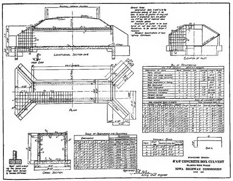
FIG. 182.—Details of standard reinforced concrete box culvert of the Iowa Highway Commission.
