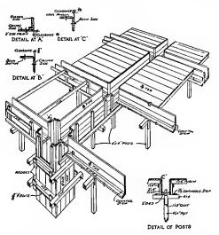
FIG. 207.-Beam and girder forms, bottom detached.
