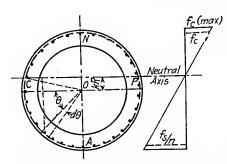
Fig. 199.—Stresses in a reinforced concrete chimney.
