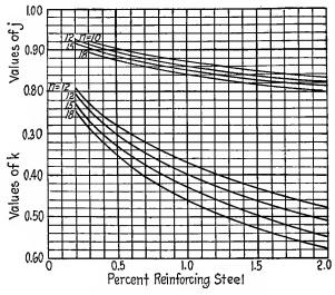
FIG. 27.—Diagram for values of k and j.
