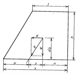
FIG. 88.-Calculation of section of a gravity dam.
