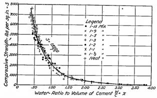
FIG. 20.-Relation between water-cement ratio and strength of concrete.
