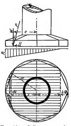
FIG. 201.—Soil pressure under a chimney base.
