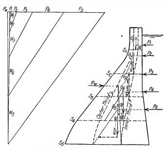
FIG. 89.—Graphical analysis of stresses in a gravity dam.
