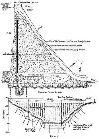
FIG. 86.—Section of the lower Otay dam (proposed).
