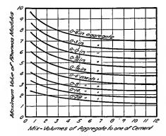
FIG. 21.-Maximum permissible value of fineness modulus.
