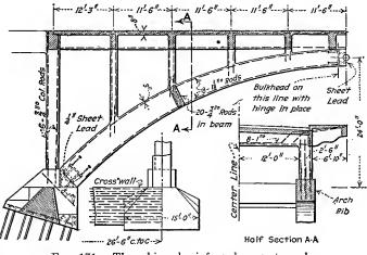
FIG. 171.-Three-hinged reinforced concrete arch.
