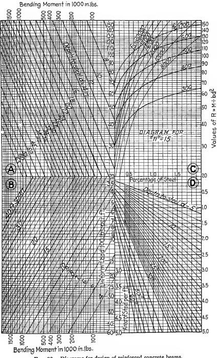
FIG. 39.-Diagrams for design of reinforced concrete beams.
