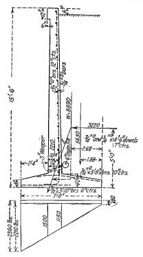
FIG. 114.-Section of a cantilever retaining wall.
