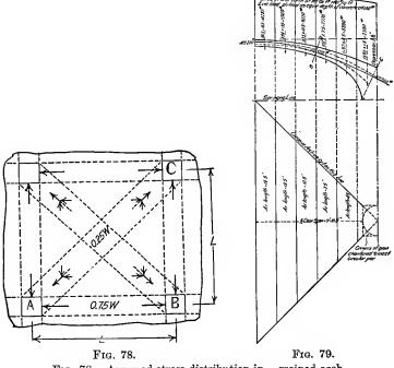
FIG. 78.—Assumed stress distribution in a groined arch. FIG. 79.—Stresses in a groined arch.
