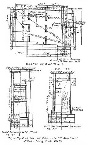
FIG. 131.—Details of a reinforced concrete V-abutment, C. M. & St. P. Ry.
