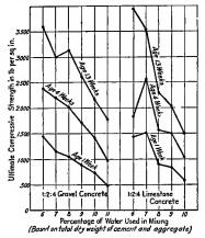
FIG. 17.--Relation between strength of concrete and the amount of water used.
