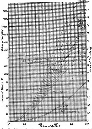
FIG. 60.—Influence lines for moments, thrusts and shears at crown; filled spandrel arch, type A<sub>3.0</sub>.
