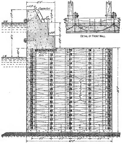
FIG. 119.-Section of Vancouver dock wall.
