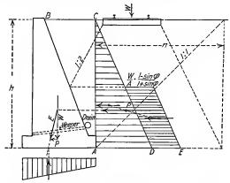
FIG. 111.-Pressure due to loaded fill on a retaining wall.
