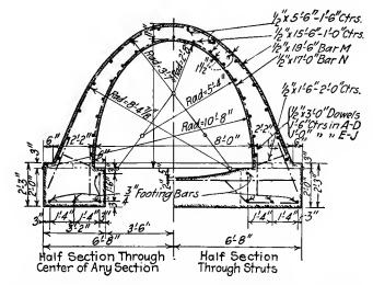
FIG. 181.—Details of a standard arch culvert of the C. M. & St. P. Ry.
