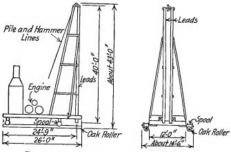
FIG. 235.—Spool roller pile driver, C. M. & St. P. Ry.
