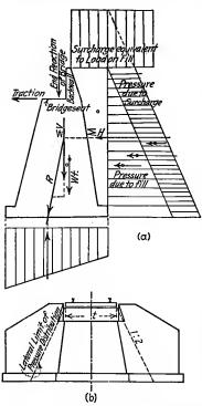
Fig. 126.—Forces acting on a bridge abutment.
