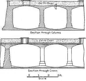
FIG. 80.-Section through groined arches at Washington.
