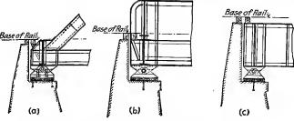
FIG. 135.—Position of superstructure on an abutment.
