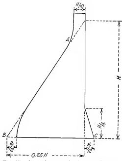
FIG. 87.—Approximate section for a gravity dam.
