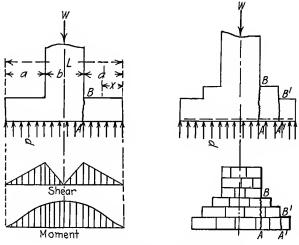
FIG. 224.—Diagrams of wall footings.
