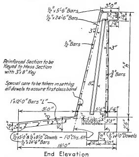
FIG. 124.—Compromise section of a retaining wall of the C. M. & St. P. Ry.
