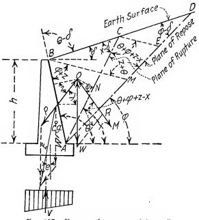
FIG. 107.—Forces acting on a retaining wall.
