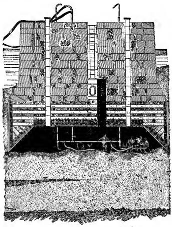
FIG. 252.-Section through a pneumatic caisson.
