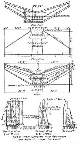
FIG. 127.—Details of a mass bridge abutment of C. M. & St. P. Ry.
