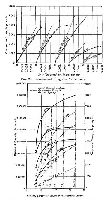
FIG. 25.— Effect of proportions and age on properties of concrete.
