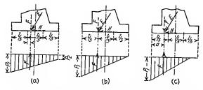
FIG. 112.—Distribution of pressure under a retaining wall.
