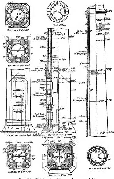
FIG. 197.—Details of a chimney of common brick.
