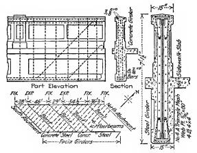
FIG. 158.-Steel girder encased in concrete.
