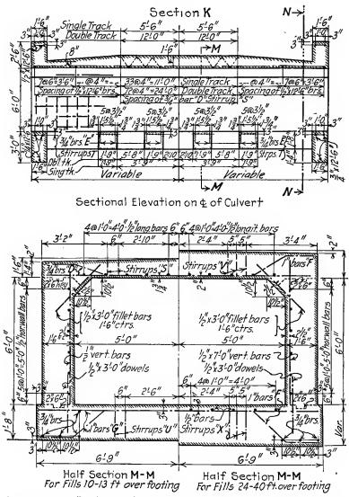
FIG. 180.—Details of a standard rectangular culvert of C. M. & St. P. Ry.
