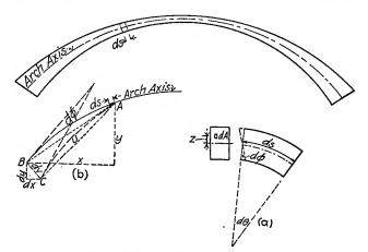
FIG. 45.—Deformation of a curved beam.
