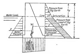
FIG. 118.—Forces acting on a quay wall.
