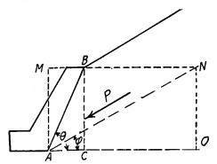
FIG. 108.-Retaining wall inclined towards the fill.
