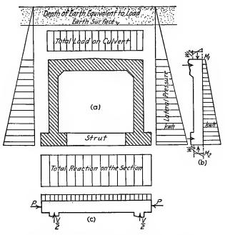
FIG. 174.-Forces acting on a rectangular culvert.
