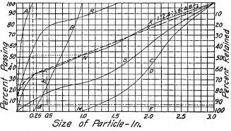
FIG. 18.—Sieve analysis curves and curve of maximum density.
