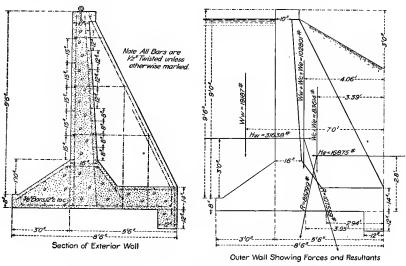
FIG. 120.—Section of reservoir wall at Webb City, Mo.
