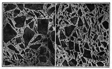
FIG. 13.-Sections through concrete.
