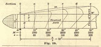
\* Under a uniformly distributed load, the bendg mom, at cen of span, is WL/8; and the bendg moms, M, and the resulting longitudinal unit stresses, s, vary as the ordinates of a parabola, as indicated by the dotted parabola, rme, at top of Fig 19, which corresponds to a uniform load = 400 lbs = 2 W. The unit shears, v, in a given hor section, then decrease uniformly, from a max, at the supports, to zero at the cen of the span. Compare 3d and 4th figures, p 474.
