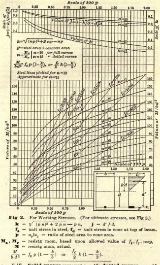
$n = E_s/E_c$ . Solid curves represent n = 10; dotted curves, n = 15. Steel lines plotted for n = 10; approx for n = 15. 11. Hence the **position of the neutral axis** (given by k) depends solely upon the ratio, p, of steel area to conc area, and upon the ratio, n, of elasticity betw steel and conc. For approx values of k, see ¶ 12.
