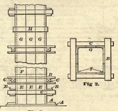
Fig 1. Figs 1 and 2. Column Form.
