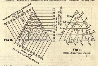
13. The results, obtained in a certain case, with diff mixtures of these three grades of fineness, are shown in Fig 2, which is similar to diagrams used in connection with alloys of three metals.
