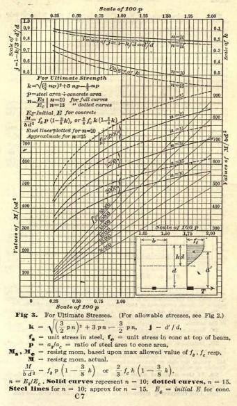
**20 d.** It can be shown (T & M, pp 175-6) that, with given M, given unit stresses, and given unit prices, the **cost** of a reinfd conc beam, per unit of length, **varies** inversely as d, directly as  $\sqrt{b}$ , and directly as  $\sqrt[p]{b/d}$ . Hence, for a given bd, the deeper the beam, the less is the cost; but practical considerations (such as practical limits to reduction of b, requirements as to head room, etc) often limit the extent to which this economy can be carried in practice.
