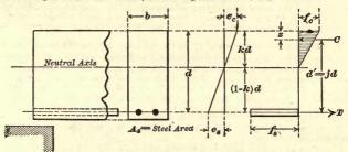
Fig 1. Reinforced Concrete Beam. Theory.
