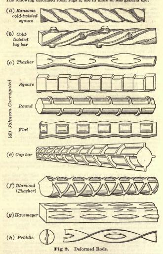
21. Ransome. (a) Square steel rods, twisted cold. Twisted either at mill, or (conveniently and inexpensively) on the work.
