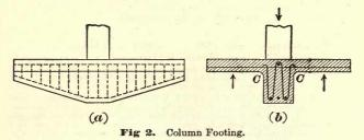
d d', d d'. Fig 2: Combined beam and slab. Side wings of slab tend to bend upward, breaking away from the beam at C and C.
