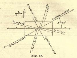
108. Let Fig. 18 represent a small element in a bar under tensile & shearing stresses; and let it be required to determine the positions of these planes and the corresponding max stresses. Let
