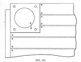
with the back bonnet off. The line A on the valve overlaps the line B on the steam chest toward the center of the cylinder.
