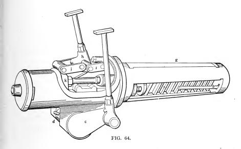
of the head e and turning the rod, an adjustment of the valve setting can be made, as will be shown later.
