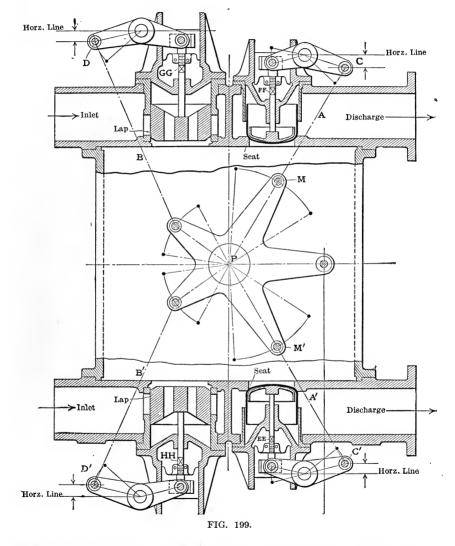
inlet pins DD' are —— inches from the horizontal line, and adjust the valve stems GG until each of the top inlet valves are lapped —— inches. Next turn the engine over, set the piston at the bottom of the stroke, the wrist plate again being central, adjust the valve stems HH until each of
