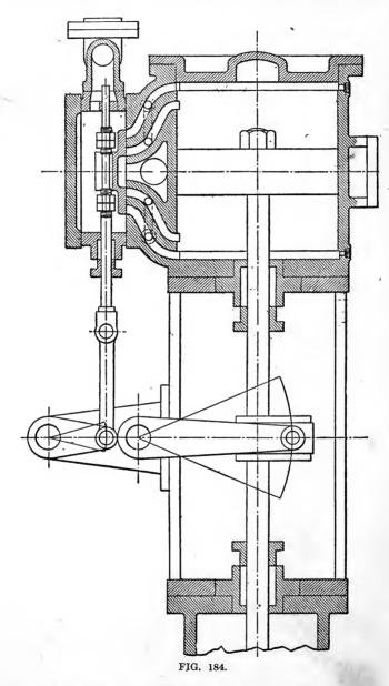
tional plans of the steam cylinders of a compound pump, with the pistons in positions that correspond to lines A—B and B—C in the diagram Fig.
