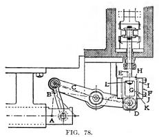
the arrangement gives the greatest velocity of valve movement at the points of opening and closing and provides a long dwell between these points.
