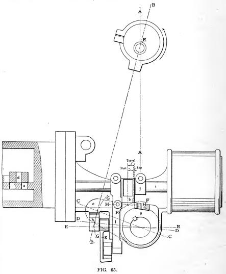
For the sake of simplicity, each valve, i.e., outlet and inlet, is shown with its gear separate for the moment, eliminating one while the other is under consideration. The cross section of the valve and seat is not in
