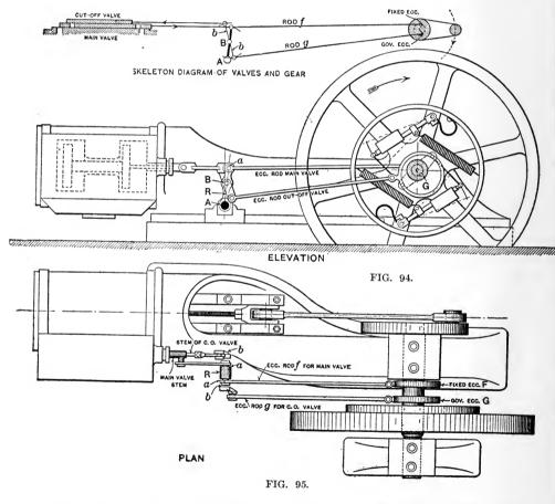
and a flat cut-off or auxiliary valve riding inside of the main valve. The single short port at each end of the cylinder serves alternately for the purposes of admission and exhaust.
