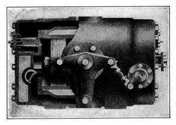
FIG. 196. — AIR CYLINDER WITH AUTOMATIC DISCHARGE.
