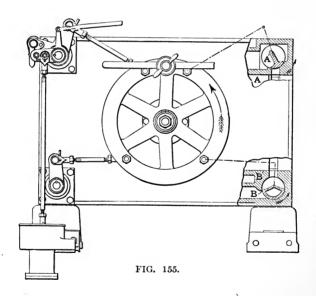
155, at A and A'. Logically, the steam exhausts over the edges of the exhaust valve and port nearest the cylinder center; these edges are shown at B and B', Fig. 155. In the figures the direction of travel of both valves when opening is indicated by arrows.
