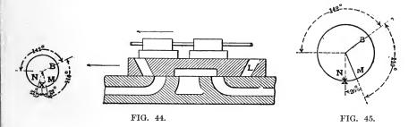
valve. Finally if the cut-off eccentric were moved to the position X, Fig. 45, at the time the main eccentric stood at M, the cut-off valve would not effect the cut-off at all. The cut-off eccentric is thus shown to be in position to cut off at the latest possible point, without reopening the port, as shown in Fig. 40.
