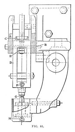
and the bottom of the brass drip cup C is the exact width of a steel gauge, or  $\frac{7}{8}$  in. Then make the stem fast to the guide by means of the nuts at E.
