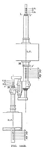
showing in each case (by marks on the valve, remember) measured and compared and if found unequal, the length of the connections changed by an amount equal to one half the difference between the two openings, lengthening or shortening as required so as to throw the valve toward the end at which the smallest opening was shown. For instance, suppose the smallest opening was shown at the "crank end," the connections should be shortened, and vice versa.
