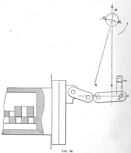
the other, the valve is lapped as shown with the point b where it is. This is the extreme of travel for the valve and stem in this direction.
