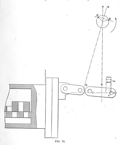
It will be seen by this that the valve moves four times between the points of closure and opening, which is a distinctive feature of this valve.
