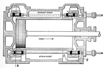
FIG. 108. - HORIZONTAL SECTION OF CYLINDER.
