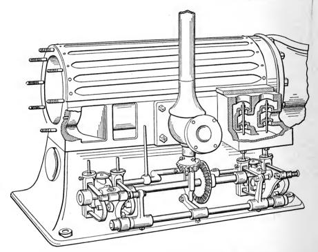
FIG. 135. - SECTIONAL VIEW OF VALVES AND STEAM PASSAGES.
