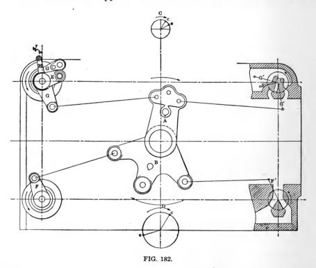
have been set with the wrist plates central, release the wrist plates and roll the eccentrics around the shaft to test them and the reach rods, and see that they are of the right length to make the wrist plate travel equally each side of the center line.
