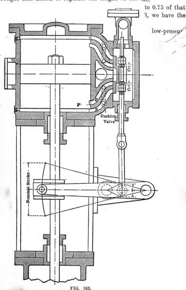
is a connection, provided with a valve, between the two high-pressure exhaust pipes. The object of this connection is to equalize the pressure in
