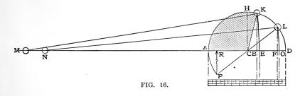
for the latter. To equalize the compression, therefore, it is customary to use less inside exhaust lap at the head end than at the crank end. Or, the crank end may be made line and line if the cylinder clearance is small, and the lap at the head end is cut away so as to give negative lap at that end
