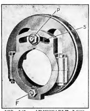
FIG. 143. — ADJUSTABLE LOW-PRESSURE ECCENTRIC.
