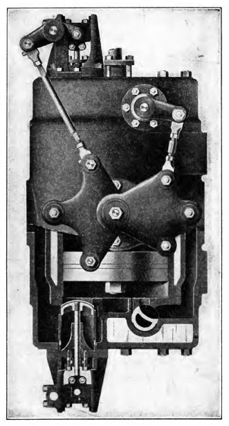
FIG. 197. — AIR CYLINDER WITH MECHANICAL DISCHARGE VALVE.
