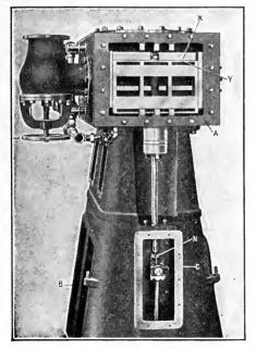
FIG. 141. - LOW-PRESSURE VALVE SIDE SHOWING LEAD ON TOP END.
