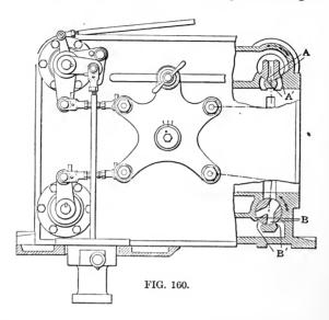
those illustrated in Figs. 155 and 156 in having less heavy wrist plates to suit higher engine speeds, and in being equipped with double-ported steam and exhaust valves.
