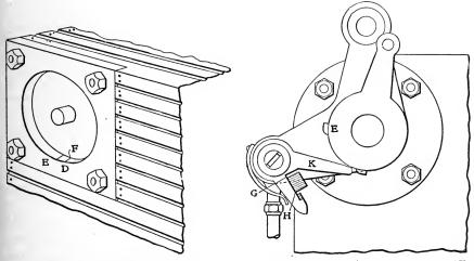
FIG. 59. — SHOWING MARKS ON VALVE SEAT.
