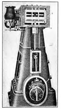
FIG. 144.—LOW-PRESSURE VALVE SIDE SHOWING LEAD ON BOTTOM END.
