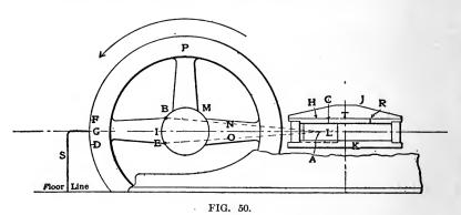
head rests at the end of the stroke, in order to find the "dead center." The writer believes the process illustrated in Fig. 50 is an accurate process.
