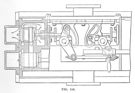
the other end to force the valve back without the aid of the cam motion when the return begins. This is evidenced by the fact that when steam pressure is on the cam is kept pressed against the driving roll at all times and after long use there is no sign of wear on the back side of the slot.
