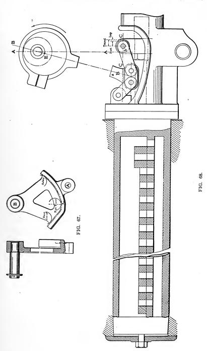
toggle stub end has come up toward the line CC; the point b has reached a position corresponding to the near edge of the ports and the valve has just cut off or closed for compression.
