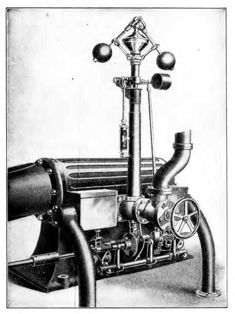
FIG. 132. — VALVE GEAR OF THE PUTNAM ENGINE.
