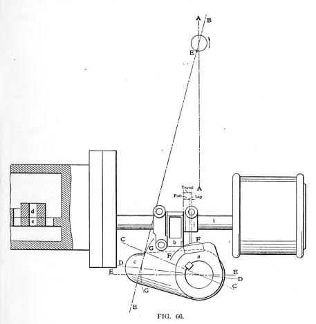
the pusher crank at the top of its movement, D D is the pusher-crank center at the lower end of its travel, E E is the center line of the pusher-crank shaft, F F is the line of travel of the pusher-plate edge, G G is the line of travel of the pusher-crank pin, a is the pusher, b is the latch, c is the pusher crank, d is the valve, e is the valve seat, f is the lifter, g is the trip cam, h is the trip-cam yoke, i is the valve stem and j is the head.
