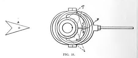
around so that both points correspond and the eccentric will then be on one "dead center." From the points J and L scribe the arcs OP and QR, ending at the points O and Q on the edge of the strap. From the points O and Q scribe arcs intersecting at the point S on the edge of the strap. With the chisel make a mark on the strap at S. Bring the eccentric around so that the point F corresponds with the point S, and the eccentric will be on the opposite end of the travel.
