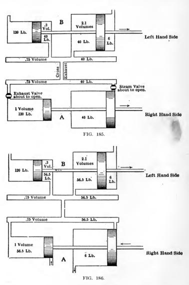
pands from the high-pressure cylinder through the intermediate space into the low-pressure cylinder doing useful work upon the low-pressure piston.
