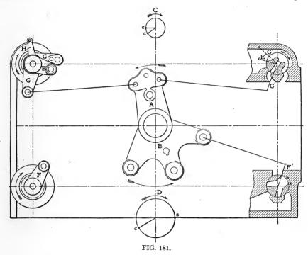
at the same time, although they may appear to be arranged to the contrary. On an ordinary Corliss engine the valves will hook up without releasing when the regulator is at its lowest working position, but with this type the valves are released alternately every stroke, no matter how low the regulator, unless it is in the safety position, when the valves would not pick up at all.
