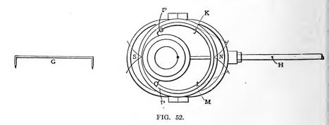
driven by one eccentric. Also assume that the builders have made all proportions, lap, width of ports, and bridges correct. Take out the cut-off valve and start to adjust the action of the main valve, bearing in mind it should be set practically the same as any D slide valve.
