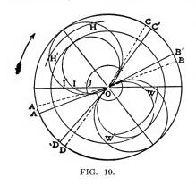
lier (at O-A), the lead being increased an amount equal to I-I', while cut-off takes place later (at O-C'); O-B' in the figure comes ahead of O-B, showing that release is earlier the greater the eccentricity and, since O-D' comes after O-D, it is plain that compression is later. Since the upper valve circle cuts the arc drawn from O as the center, with a radius equal to the outside lap plus the width of the steam port, in the points W' and H', the admission port
