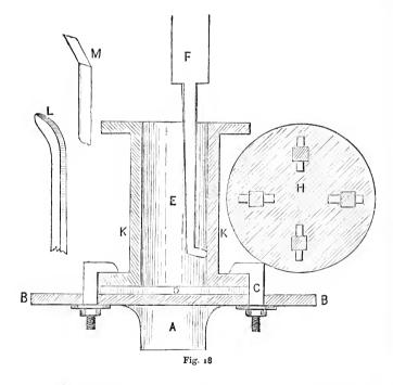
sawn diagonally, and is an excellent mode of drawing to explain machinery. F is the tool, which is supposed to have almost reached the bottom. It is merely a flat steel
