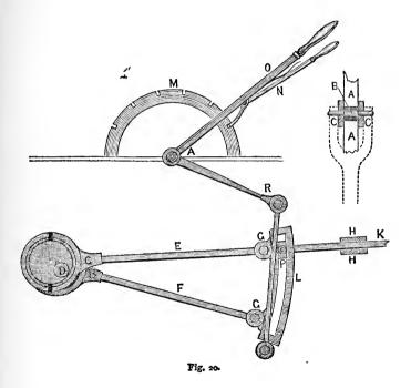
of the eccentric rod E, and also that of F. K is the rod of the slide-valve, working between guides, HH; but if there are two stuffing-boxes to the valve-casing, these
