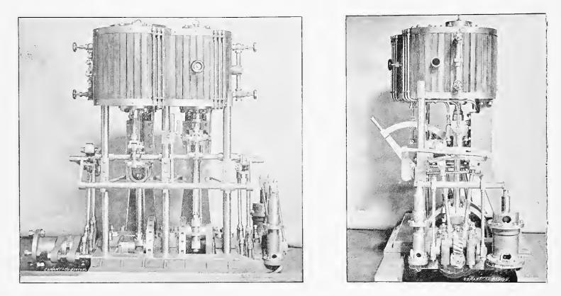
COMPOUND YACHT ENGINE, WITH AIR AND FEED-PUMP ATTACHED -Designed and Built by the Edward S. Clark Co., Boston, Mass.
