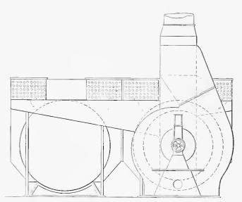
FIG. 4.-REAR ELEVATION, SHOWING POSITION OF FAN ENGINES.
