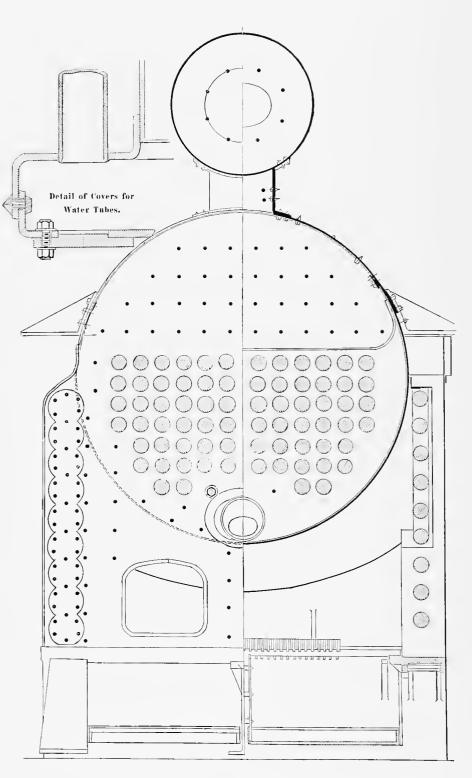
SLOAT'S FIRE AND WATER-TUBE BOILER.
