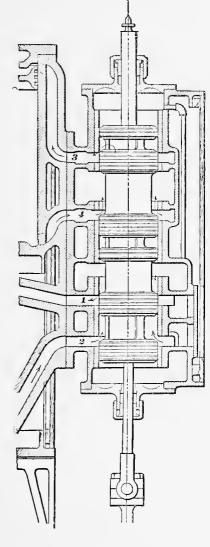
FIG. 3.—CANFIELD'S BALANCE VALVE.
