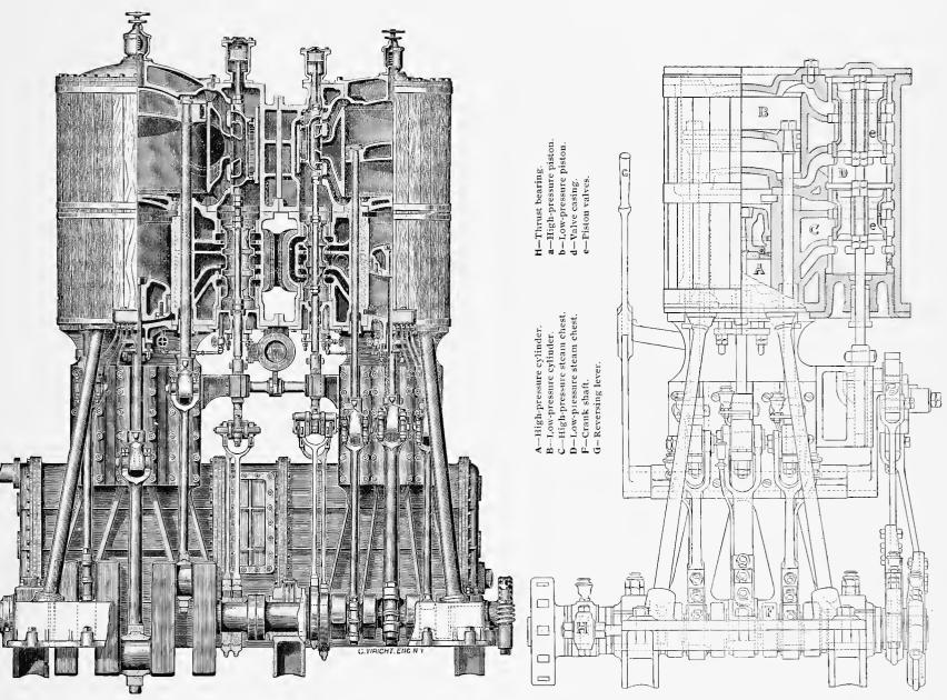
Wells' Patent Quadruple-Expansion Engine.
