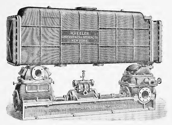
RECTANGULAR PATTERN OF THE WHEELER-ADMIRALTY SURFACE CONDENSER MOUNTED UPON COMBINED AIR AND CIRCULATING-PUMPS.
