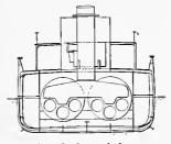
York and Maracaibo. In order to cross the bar at the latter port, the draught is limited to 10 feet only, which enables the vessel to carry 900 tons dead-weight. The gross tonnage is 1,500 tons; the speed is 11 knots, and 12 knots were made on a trial of four hours' duration, which places her in the fourth class of the U. S. ocean mail service. The en-
