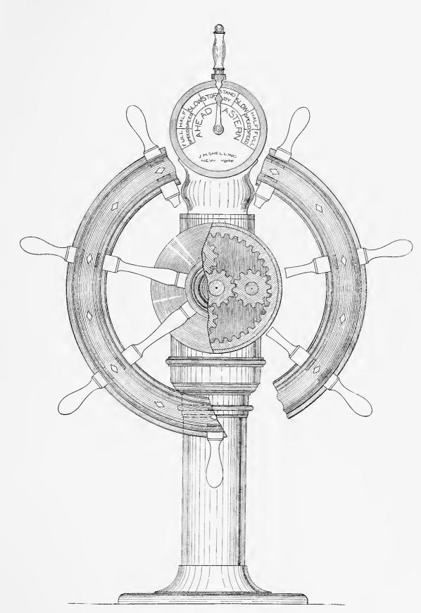
SNELLING'S COMBINED HAND STEERER AND ENGINE-ROOM TELEGRAPH.
