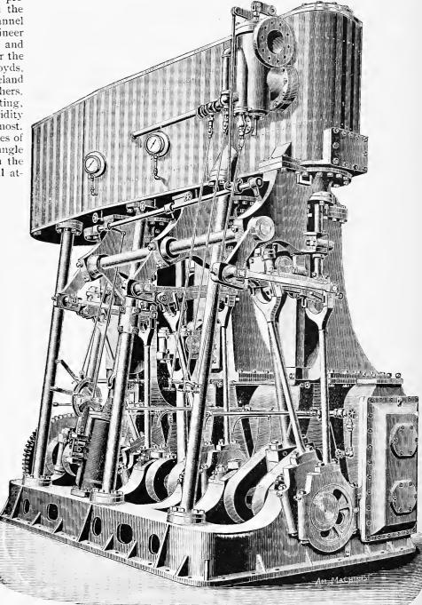
TRULE-EXPANSION ENGINE OF THE BRIDGEPORT LINE STEAMER NUTMEG STATE.
