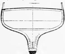
by softened curves, a broad hull with a weak depth on the lines of the celebrated Sappho and under that upper one another very narrow one, very high, intended to receive the ballast. The length of the second receptacle is so great, in proportion to its width, that its resistance is hardly more than the surface friction, and, notwith-
