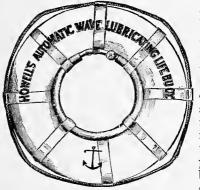
the tube there is inserted a light brass tube, small enough to fit snugly into the rubber, thus forming a tight joint. On either side of the brass tube there is fitted a brass rose (similar to that on a sprinkling can or watering pot), which is soldered to the former. There is also fitted a brass cap which is screwed into the metal tube. to be used for filling the rubber pipe with oil. When the buoy is hung at the stern or on the vessels' quarters,
