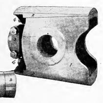
Fig. 14. Typical Crosshead and Pin for Large Size Engine
