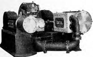
Fig. 20. Typical Cross-Compound Engine
