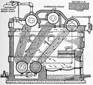
Fig. 75. Section of a Separately-Fired Type of Superheater
