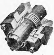
Fig. 11. Stuffing Box Packed with Metallic Packing
