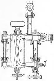
Fig. 99. Section of Sight-Feed Lubricator
