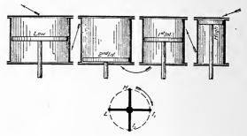
Fig. 57 Diagram Showing Quadruple-Expansion Cylinder Arrangement
