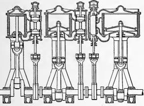
Fig. 22. Section of Essential Features of Triple Expansion Engine
