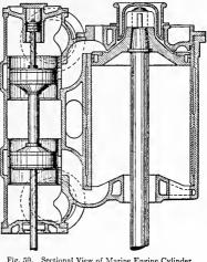
Fig. 59. Sectional View of Marine Engine Cylinder, Piston and Steam Ports
