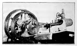
Fig. 23. Simple Slide Valve Engine of Side-Crank Type
