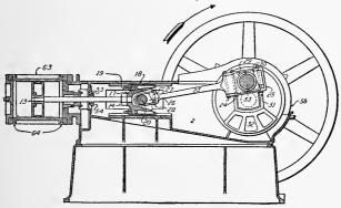
Fig. 6. Side Elevation of Modern Simple Engine
