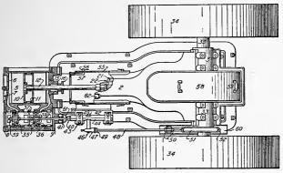
Fig. 5. Plan View of Modern Simple Engine
