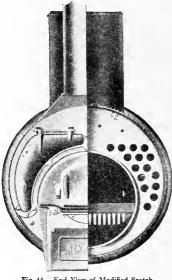
Fig. 44. End View of Modified Scotch Marine Boiler
