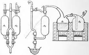
Fig. 1. Early Form of Steam Pumping Engine
