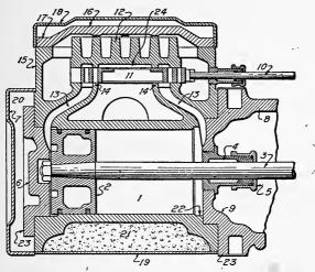
Fig. 8. Cylinder and Valve Mechanism Shown in Section
