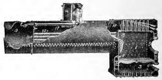
Fig. 43. Traction Boiler of the Locomotive Type
