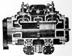
Fig. 35. Cylinder and Valve Arrangement in Skinner Unaflow Engine. Piston on Head-End Dead Center and Exhaust Taking Place Through Central Ports
