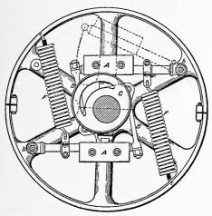
Fig. 93. Diagram Showing Action of Buckeye Shaft Governor
