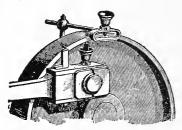
Fig. 97. Form of Wiper Crank Pin Oiler
