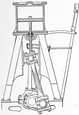
Fig. 58. Section of Typical Vertical Marine Engine
