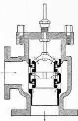
Fig. 92. Section of Valve and Valve Seat of Waters Governor
