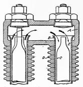
Fig. 74. Section of Foster Superheater Tubes
