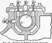
Fig. 18. Section of Babbitt Lined, Quarter-Boxed Main Bearing
