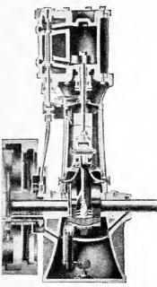
Fig. 24. Vertical High Speed Engine
