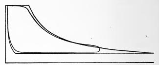
Fig. 71. Superposed Ideal and Actual Indicator Diagrams
