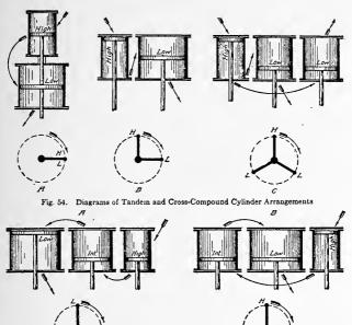
Fig. 55. Djagrams Showing Triple-Expansion Cylinder Arrangements
