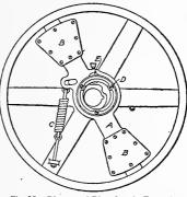
Fig. 95. Diagram of Rites Inertia Type of Shaft Governor
