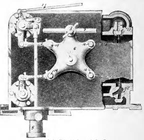
Fig. 27. Corliss Valve Mechanism in Detail
