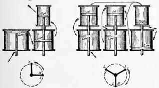
Fig. 56. Diagrams Showing Other Triple-Expansion Cylinder Arrangements
