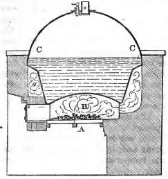
the kind called a flange boiler, the upper part being made to project over the flue, which went round the lower part; as will be readily understood from the sketch.
