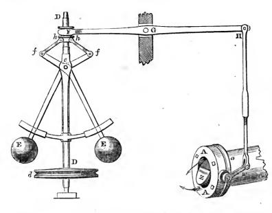
E e are attached by a joint at e, and they have heavy balls E E fixed at their lower ends, to form two pendulums, which being carried round with the axis, their balls E E will describe a horizontal circle, and their centrifugal force will cause them to recede from the axis D, in opposition to their own weight, which tends to approach them to that axis (see an explanation of
