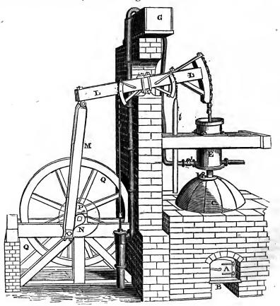
The fly-wheel Q is made heavy in the rim, but balanced on its axis so as to be equally heavy on all sides; the millwork which the engine is required to turn is connected with the other extremity of the axis P of the fly-wheel.
