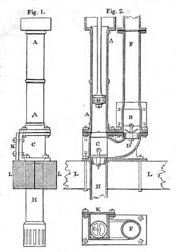
Fig. 1 is an elevation of the forcing-pump taken endways, of the engine, as it would appear to a spectator standing beneath the great lever of the engine. The barrel of the lifting-pump, if it had been represented in this view, would have stood close by the side of the barrel A A, in the same relative position as fig. 2, but much nearer together.
