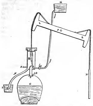
rod M with the bucket of the pump will be drawn up, with a corresponding motion, and will raise the water through the barrel of the pump, till it runs out at the spout. To cause the return of the piston J, when it is released from the pressure which occasioned its descent, a sufficient counter weight is applied to the rod M of the pump, to overbalance the piston, and draw it upwards to the top of the cylinder, as shown in the figure.
