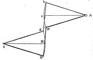
Suppose two equal levers A B and C D to be placed one beneath the other, in the same vertical plane, and to be movable about the fixed centres A and C, so as to be capable of assuming the different positions represented by the dotted lines, and by the strong black lines in the figure ; their extremities B and D are connected together by the link B D, so that if one lever is moved up or down, the other must accompany it, and CHAP. VI.]
