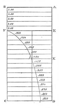
Let A B C D represent a section of the cylinder of a steam-engine, and E F the surface of its piston. Let us suppose that the dense steam was freely admitted from the boiler, whilst E F was in contact with A B, but that as soon as that steam had pressed it down to the situation E F, the steam-valve was shut. The steam will, nevertheless, continue to press down the piston by its own elasticity and force of expansion; but as the steam expands, its elasticity and pressure must diminish.
