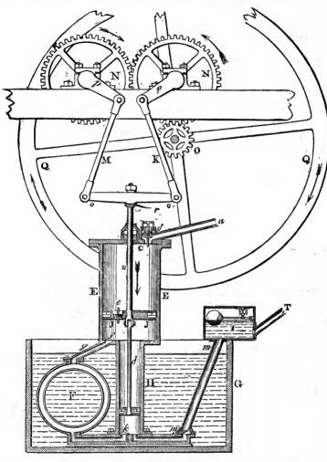
upon the piston. e Is a valve in the piston to admit the steam to pass from the upper part of the cylinder into the lower part.
