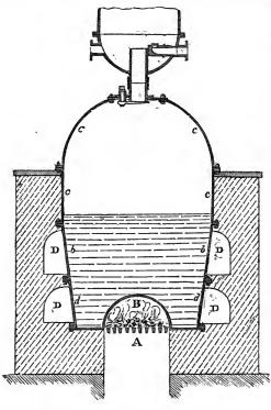
flange all round its lower edge; and by this it was united to a cylinder c c, placed with its axis vertical: it was 10 feet diam. and 4 feet deep, cast in one piece, and united by a flange to another piece, b b, of 4 feet deep, 10 feet diameter at the top, but tapering to 9 feet diam. at the bottom. This cylindrical piece was joined by a flange, to another piece, d d,  $3\frac{1}{3}$  feet deep, 9 feet diameter at top, and 8 feet at bottom.
