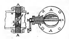
A thin circular plate Z is fitted into the aperture of the steam-pipe, by means of an axis Z Z, which passes across its diameter; and it can be turned by this axis from the outside, so as to present either its thin edge or its flat surface to the steam; in the latter case it quite fills the circular aperture of the steam-pipe, so as nearly to stop the passage of the steam.
