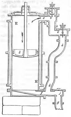
the piston. In this construction the equilibrium-valve e becomes also the exhaustingvalve, for when it is opened it allows the steam to pass from the top of the cylinder to the condenser. In these engines a valve was sometimes placed in the eduction-pipe at j, but it was only used to regulate the rapidity of the flow of the steam through fand g to the condenser, and was not connected with the working gear; it was always kept partially open.
