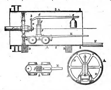
he contrived a small wheel carriage to go into the cylinder, and form a fulcrum or support for a lever or steelyard, from one end of which the end pivot of the axis of the boring head was suspended by a link, and on the other end of the lever, a sufficient weight was applied, to counterbalance the weight of the boring tool, which being by this meansundetermined to any side, might be expected to cut
