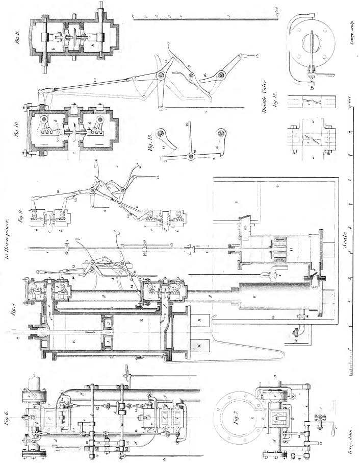
CYLINDER and VAINES of M& WATT'S Palent Rotative STEAM ENGINE.
