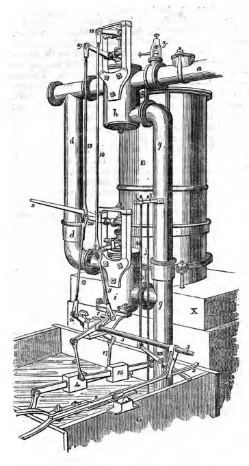
outside of the boxes, in order to open the passages through the valve seats; the two valves of each pair can be opened or shut quite independently of each other.
