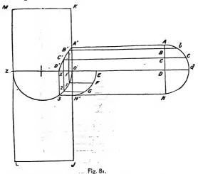
To describe the Pattern for a T-piece formed by two equal or unequal circular Pipes (cylinders of equal or un-
