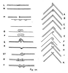
angles of sheet-metal. A and B are or the thinnest metals, such as tin, which require a film of soft solder on one or the other side. Sheet lead is similarly joined, and both are usually soldered from within.
