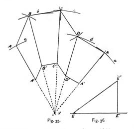
and meeting it in Q, and through O' draw O' Q' perpendicular to XX and cutting xx in e'. Join Q e' and produce it to intersect v V' in V'. Next make va, vb, vc, vd, equal to VA, VB, VC, VD respectively; join a, b, c, and d to V' by lines cutting xx in points a' b' c' and a'; aa', bb', etc., are then the lengths of the edges of the frustum.
