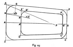
draw A"A perpendicular to AA', then AA' will be the distance between the lines, in plan, of the top and bottom at the head. Make AA' (Fig. 29) equal to AA' (Fig. 27) and A'B' equal to the length of the bottom. Through A' and
