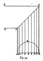
B, etc., and the curve being drawn through these points will give the bottom of the tapering piece.
