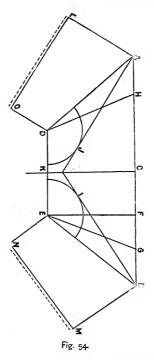
the difference of the top and the shortest side of the base, as from G to F, describe the arcs J and I; draw the rightangled lines JAL and IBM; set off AL and BM equal in length to CG, and draw the lines MN and LO at right angle to BM and LA; also, the lines NE and OD at right angle to NM and OL.
