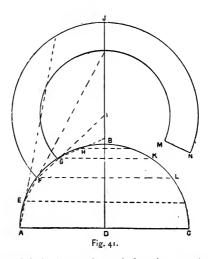
First Method. Assume the vertical section, or axis, to be divided into a number of equal parts, and the roof, or figure, cut by planes through the points of division par-
