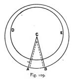
shown by the distance between the two circles and the dot on the line AC (Fig. 109), the circle DE representing the hoop; take the distance from A to the dot on the line AC, and set off three times the distance on the outer circle, as from A to B; draw the lines AC and BC, cutting the centre at C.
