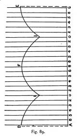
HF (Fig. 88); make OI, OI equal to BG (Fig. 88); also, each of the parallel lines bearing the same figures as 2 2, 2 2, 3 3, 3 3, etc.; then a line traced through the points will form the pattern.
