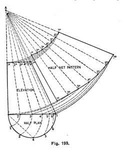
side. Then  $1^x$ ,  $7^x$ , 7, 1 is the outline of the joint in elevation constituting a frustum of a cone in geometrical parlance. Continue lines  $11^x$  and  $77^x$  until they meet at the apex A. Divide the half plan into equal spaces as shown and using point one as center swing these points up to line 17. Then from 1 to 2' and so forth are the bases of the
