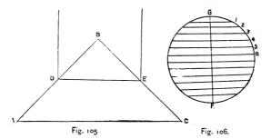
be the pitch of the roof; make DE equal to the diameter of the pipe; describe the circle FG (Fig. 106); make FG the same in diameter as the pipe; draw the line FG; set off on the line FG any number of equal parts; from the points draw lines at right angle to FG, as 1, 2, etc.
