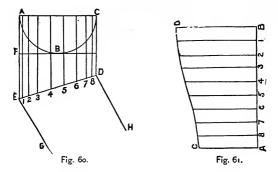
Make BD equal to EA, and AC equal to DC; also, each of the parallel lines bearing the same figures as 1, 2, 3, etc.; then a line traced through the points will form the pattern.
