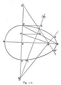
arc to meet the arcs DH and CH' in H and H', and to complete the egg-shaped oval.
