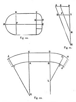
arc BF, also the arc DE; set off BF equal to CD, in Fig. 20; draw the line EF, cutting the centre at L; draw the lines FG and EH at right angles to EL; make FG, equal to DE, in Fig. 20; draw the line HG at right angle to EH.
