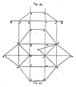
angles to f d. Join d s, then the right-angled triangle, d f s, is the true shape of the hip truss. This will be understood
