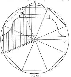
*Cover.*—Describe a circle that will cut the required Octagon (Fig. 67); draw a line that will cut the centre of two sections, as AI; erect the perpendicular line HF; let ABCDEFJ be the given top or cover; divide the curved lines BC and EF into any number of equal parts; from the points draw lines parallel to FH, as 1, 2, 3, etc., H, 1. 2, 3, etc.
