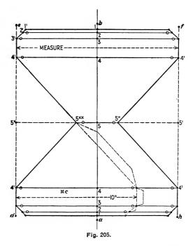
like numbered points in the profile, as shown. Note that the glass line and measuring point is on line 8 and for the layout of Fig. 202; two curbs would be cut with this miter
