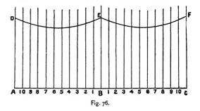
circumference of the collar AB; erect the perpendicular lines AD, BE and CF; set off on each side of BE the same
