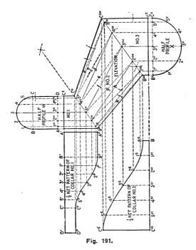
divide the round portion of half profile W into six equal spaces. Project the points in half profile X up to miter line  $B^{or}C^{or}$ , and indicate where they intersect this line,
