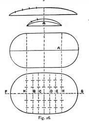
kettles with curved sides, i. e., a true oval or ellipse. A round article will also be made the proper size, if the length of curve be taken at which the cover or bottom must be finished.
