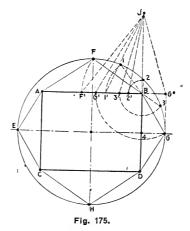
top. This diagram also shows the triangulation and Fig. 176 shows the half pattern. Thus it will be seen that the
