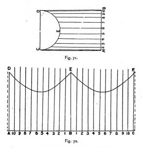
To describe a Pattern for a T Pipe at any Angle.—Draw the line AE (Fig.  $7_3$ ); erect the line AB, the angle required; also, the line ED parallel to AB; make BD equal to the diameter of the Pipe; describe the semicircle BCD; draw the line FG parallel to BD; divide the semicircle into any number of equal parts; from the points draw lines parallel to AB, as 1, 2, 3, etc.
