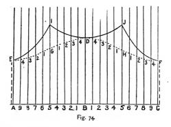
CF at right angles to AC; set off on each side of BD the same number of equal distances as in the semicircle BCD
