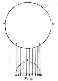
To describe a Pattern for a TPipe, the Collar to be Smallethan the Main Pipe.—Let the circle GH (Fig. 75) equal the large pipe, AB, CD, the branch or collar; describe the
