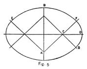
tude, draw the line DF at right angle to BC; make DF equal to AB in Fig. 5; make AB equal to DF and the taper required on a side, draw a line cutting the points A and D, and the line BC.
