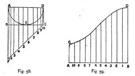
circle; from the points draw lines parallel to BD, as 1, 2, 3, etc., make BD equal in length to AF (Fig. 58), and AC equal in length to BE; also, each of the parallel lines bearing the same figure, as 1, 2, 3, etc.; then a line traced through the points will form the pattern required.
