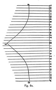
To describe a Pattern for a T Pipe at any Angle, the Collar to be set on one side of the Main Pipe.—Let the circle FE (Fig. 79) equal a large pipe or boiler; make AB equal to the diameter of the collar or branch pipe, BE the angle required ; describe the semicircle ACB ; divide the semicircle into any number of equal parts ; from the points draw lines parallel to EB, as 1, 2, 3, etc.
