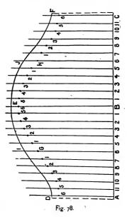
the semicircle CDE; make CF and EH of equal length; with a radius equal to one-half the diameter of the large pipe, describe the arc FH; divide the semicircle into any number of equal parts; from the points draw lines parallel to AC, as 1, 2, etc. There must be an odd number of lines, as in the diagram, so that one of the lines runs through the centre of the semicircle.
