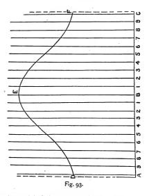
divide the semicircle into any number of equal parts; from the points draw lines parallel to BC, as 1, 2, 3, etc.
