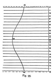
AGB (Fig. 94); from the points draw lines parallel to BE, as I, I, 2, 2, 3, 3, etc.; make BE equal to BF (Fig. 94); make AF and CD equal to AE; also, each of the parallel lines bearing the same figures as I, I, 2, 2, 3, 3, etc.
