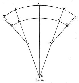
to GE, and the taper required on a side; draw a line cutting the points F and G, and the line BC; with the radius HG and, in Fig. 10, E and F as centres, cut the lines CB and DB, as at L and M; with L and M as centres describe the arcs FK and EH; also, the arcs DI and CG; set off FK and EH, equal to ED in Fig. 8; draw the lines IK and GH, cutting the centres at M and L.
