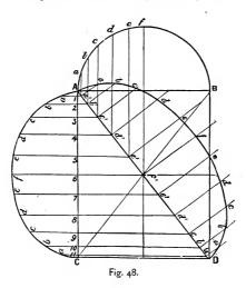
curve of the groin is then generated by the penetration of a cylindroid and cylinder.
