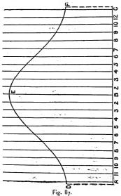
circle CDE; divide the semicircle into any number of equal parts; from the points draw lines parallel to EB, as 2, 3, 4. etc.
