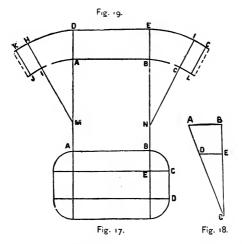
To describe a Pattern for a Tapering Oval or Oblong Article, the Sides to be Straight with Quarter Circle Corners, to be in Two Sections.—Describe the bottom, the length and breadth required as in Fig. 17; the body as in
