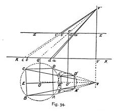
tum (here of a square pyramid). Produce AA', BB', etc., the plans of the edges to meet in a point V; this point is the plan of the apex of the pyramid of which the frustum is a part. Join O, the centre of the square which is the plan of the large end of the frustum, to V. The line OV will pass through o', the centre of the plan of the small
