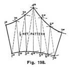
in its design other than that distance 4"  $4^{x_0}$  must equal 4 4', and distance  $4^{x_07'}$  must equal  $4^{o7''}$ . Divide profile X into three equal spaces and project them across locating, thus points 5" and 6". Connect all the points as shown with dotted and solid lines as *a* to *k*.
