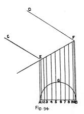
To describe an Elbow Pattern at any Angle.—Let ABCD (Fig. 94) be the given elbow; draw the line AB at right angle to BF; draw the line EF; describe the semicircle AGB; divide the semicircle AGB into any number of equal parts; from the points draw lines parallel to BF, as 1, 2, 3, etc.
