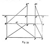
is necessarily given, or else the dimensions from which to draw it. Also the height of the hood, or the slant of one of its faces. The hood is here supposed to be a body of unequal taper with top and base parallel, but not a frustum of an oblique pyramid.
