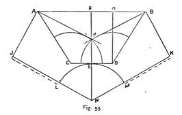
equal in length to one side of the base; make CD equal in length to one-fourth the circumference of the top, and draw the lines AC and BD; C and D as centres, with a radius equal to one-half the difference of the two ends describe the arcs I and H; draw the right-angle lines IAJ and HBK; set off JA and KB equal to FB, and draw the lines JN and KN at right angles to JA and KB; N as a centre, with the radius NE, describe the arc LEM.
