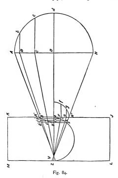
parallel to KJ; make OD equal to the length of the funnel-shape pipe, and through D draw a line AH perpendicular to Od. Now make DA and DH each equal to half
