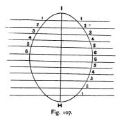
**106**, as 1, 1, 2, 2, etc.; a line traced through the points will form the piece to be cut out; when there is to be an edge turned up, it must be allowed inside of the line traced. The same rule is applied to describe a pattern for a flange for Fig. 86; make HI (Fig. 107) equal BF (Fig. 86), then proceed the same as described above.
