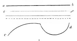
it. In general, though not always, occult lines are shown in diagrams as only useful in constructing them, but meant after the operation is performed to be erased, the determined lines being left in. A Right Line is a line which is perfectly even or straight throughout its whole extent. Lines that follow one
