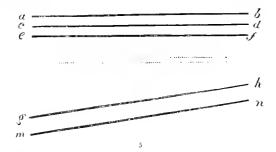
another at equal distance, and which, if produced ever so far both ways, never meet, are called *Parallel Lines*, as a b d e e f, g h n m, Fig. 5.
