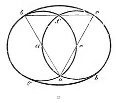
bisect each angle of the figure, as d f e, and from the points d, e, describe eircles intersecting each other at a, f. To complete the boundary line of the ellipse, place one leg of the compasses at a, and with the other describe the line from b to e, and in like manner from f describe the line h g.
