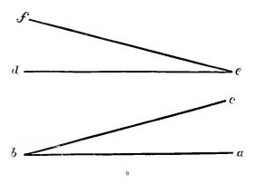
angle; when the lines are right or straight lines,\* as a b, c b, e d, f e, the angle is *Rectilineal*, but if enryed or circular, as f g b, Fig. 10, it is a *Curvilinear Angle*; and a mixtilinear angle is that which
