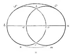
draw to m. Another method.—Draw an equal-sided triangle, as a b c, Fig. 37; the length of the angles will determine the dimensions of the ellipse:
