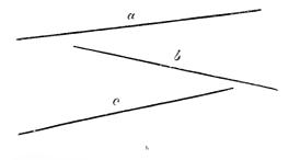
A *Horizontal Line* is that which is parallel to the horizon, or at right angles to a vertical line; a b, is a horizontal line, Fig. 7.
