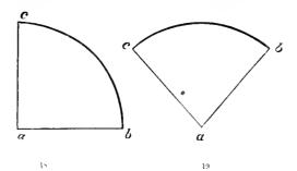
another. A Sector is part of a circle bounded by two radii, or semi-diameters, as a c, a b, Fig. 19. A Segment, as a b, Fig. 20, is a portion of a circle contained by part of the circumference.
