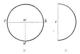
The semicircle, Fig. 17, is described from the centre, c; the quadrant from a, Fig. 18, two lines, a b, a c, being first drawn at right angles to one
