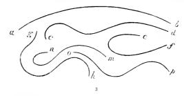
or Eccentric Line e d, e f, g h, n m, o p, is that which is drawn in more than one direction. In geometrical drawing, lines are used in two ways, "apparent" or "determined" lines, as a h, c d, Fig. 4, and "occult" or "partial," as e f, and the two below
