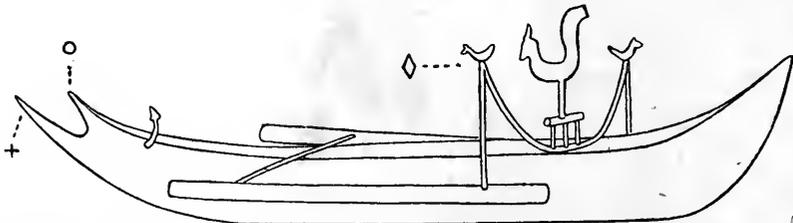
FIG. 21.—SKETCH OF A MIXED DIRECT AND ROD ATTACHMENT, BAWEAN ISLANDS
