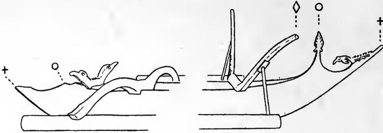
FIG. 20.—SKETCH OF A MIXED DIRECT AND ROD ATTACHMENT, MADURA
