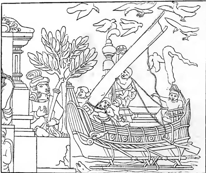
FIG. 26.—INDO-JAVANESE SHIP: ONE MAST WITH RUNGS, THREE STRAIGHT BOOMS WHICH PASS BELOW THE LONGITUDINAL SPAR AND APPARENTLY BELOW THE DOUBLE FLOAT, TWO FALSE BOOMS, THREE CURVED BOOMS WHICH PASS OVER THE LONGITUDINAL SPAR AND BETWEEN THE TWO ELEMENTS OF THE FLOAT (LEEMANS, pl. ccli, 41).
