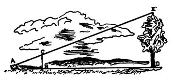
Walk on level ground to a distance from the foot of the tree or object about equal to its presumed height. Lie on your back on the ground, stretched at full length. Let an assistant note on a perpendicular staff at your feet the exact point where your line of vision to the top of the object crosses the staff. Measure the height of this, B C, and your own height to your eyes, A B. Then as A B, B C, A D, D E.
