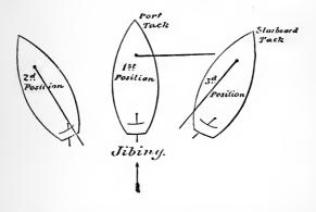
and the main-boom almost amidships; then take a good turn with it, and shift the helm gradually, till the wind is on the starboard side slightly, and the sail has filled with a slat upon that tack; when the main-sheet may be slackened, the peak hoisted, and the yacht kept on her course.
