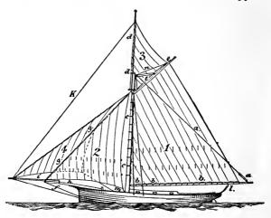
end in a small ball, called the *truck*, through the sides of which are fitted little *sheaves* (i.e., wheels), by means of which, and the use of a small-sized rope, called *signal-halliards*, the flag, or private signal of the boat, is hoisted to the *topmast's* head, and displayed.
