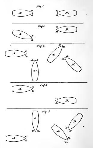
knows that either, first, a vessel is approaching him on his port bow, as B, or, second, a vessel is crossing his bows to port in some direction, as D D' D" (Fig. 3). If A sees a *white masthead light* above the *red light*, he knows that the vessel is a steamer, and is either approaching in the same direction as B (Fig 2), or is crossing to port in the same direction as D D' D" (Fig. 3).
