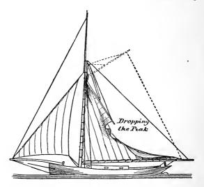
go the peak-halliards of the mainsail, so that the outer clew and head of the sail, that is attached to the gaff, will be lowered down so as to dangle alongside of the mainmast, with the gaff pointing to the deck. This makes of the mainsail, for the time being, a sort of triangular or leg-of-mutton sail, and takes off the leverage of the high part, that the wind might fill in jibing, and thus press over the yacht dangerously. (See diagram.)
