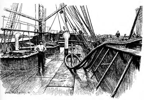
Loading a Tank Steamship with Oil, by Force Pumps.
