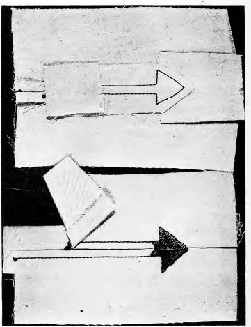
SLOT SEAM FINISHED WITH ARROW HEAD
