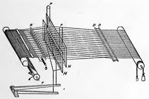
DIAGRAM OF THE WORKING PARTS OF A LOOM. S-Suttle for carrying the woof; *R*--Reed for beating up the woof; *H*-Frame holding heddles, with pullies (*P*) making the harness; *T*-Treddles for moving the harness.
