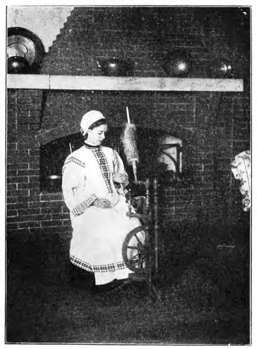
DUTCH WHEEL Spinner Sits in Front of the Wheel—Spinning Flax at Hull House.
