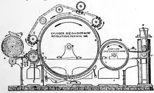
COTTON CARD The roll of webbing A is beaten and transferred to the cylinder HH, carded by the spiked belt E, removed by the "doffer" and formed into a "sliver" which runs into the can M.
