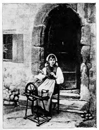
SPINNING WITH CRUDE WHEEL AND DISTAFF Distaff Thrust Into the Belt.
