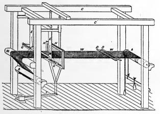
DIAGRAM OF A HAND LOOM *A*-Warp Beam; *B*-Cloth Beam; *DD*-Lees Rods; *H*-Harness, *T*-Treddle.
