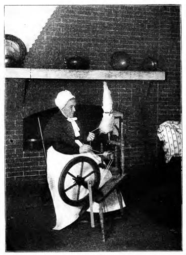
COLONIAL FLAX WHEEL Worked by a Foot Treddle; Distaff on the Frame of the Wheel; "Fliers" on the Spindle, Continuous in Action; Capacity Seven Times That of Hand Spindle.
