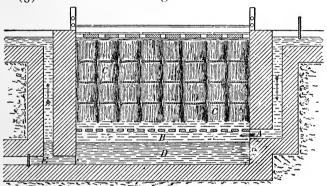
RETTING TANK *A*-Inlet; *B*-Undisturbed Water; *C*-Bundles of Flax.
