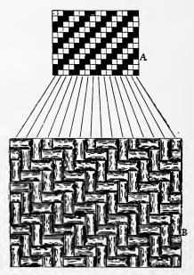
TEXTILE DESIGN A-On cross-section paper; B-Graphic diagram.
