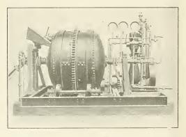
discharged thru a 2-inch pipe; 112-inch stone concrete thru a 3-inch pipe; 2-inch stone concrete thru a 4-inch pipe, and, furthermore, concrete made with the run of ordinary crusher stone thru a 6-Inch pipe.
