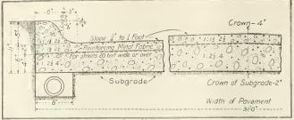
TYPICAL CROSS-SECTION OF EAST MILWAUKEE CONCRETE PAVEMENT WITH INTEGRAL CURB.
