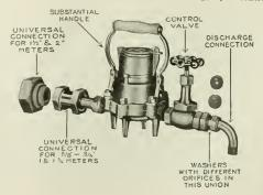
valve of testing meter; turn water on slowly at stop and waste cock, allowing several cubic feet to run so as to expel all air from the meters; then shut of water at testing meter control valve so as to stop the first hand of the service meter exactly at 0.
