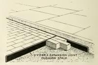
bitumen compound of great ductility and flexibility, which is made up into strips five feet long and of any width or thickness desired.
