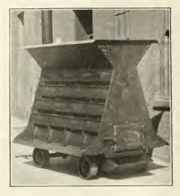
It is surprising what a small amount of fuel is required to heat and dry a large amount of gravel in this machine: but when one sees the actual construction of the machine and observes that practically all the heat from the fire passes out thru the multiple perforations in the furnace sides, thru the voids of the gravel or stone, and then escapes either thru the spaces between the flights or thru their multiple perforations, this efficiency of fuel is readily understood.
