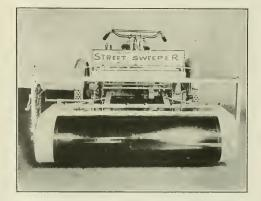
the brush revolves. Thru the agency of another lever, similar also to those used on automobiles, the driver is able at any moment, without dismounting, to turn the cylinder so that its contents will be dropped in a pile upon the street. Provision Is made to haul a wagon body at the rear of the machine large enough to hold ten loads of the cylinder. The use of this would
