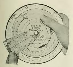
plements of angles or reciprocal functions. Equivalent ratios and reciprocals of numbers may be read at a glance; the operation for multiplication and division is identical.
