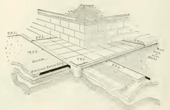
SHOWING VARIOUS USES OF PITTSBURG PAVING JOINT IN STREET AND ROAD CONSTRUCTION.
