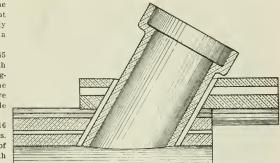
III. SECTION OF NATCO DOUBLE-TILE SEWER AND Y-BRANCH.
