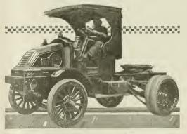
A SPECIAL 4-TON KELLY CHASSIS BUILT TO SERVE AS A TRACTOR WITH FIFTH WHEEL. THIS CHASSIS HAS A 116-INCH WHEEL BASE. ble of carrying six or seven tons, with the majority of that weight carried on the wheels of the semi-trailer. The tractor itself carries no more weight than it would if used as a regular truck, but it is capable of hauling a much larger weight than it can carry.
