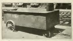
HEATER FOR DRYING AND HEATING SAND FOR FILLER.
