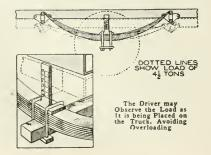
should be exactly opposite the maximum load mark, which is the highest figure on the scale.
