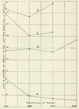
CURVES SHOWING TOTAL LOSS IN PEB CENT BY WEIGHT OF PAVING BRICKS, MORTAR BLOCKS AND CONCRETE BLOCKS SUB-MITTED TO REPEATED RATTLER TESTS OF 900 REVOLUTIONS.
