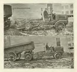
throwing the weight of the front end of the wagon on the caterpillar for traction, and at the same time giving a single vertical pivot so that the wagon may be started backward. It is rubber shod so as to make for speed. This model has already been run at a speed as high as fifteen miles an hour.
