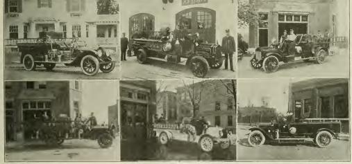
WHITE 5-TON FIRE APPARA-TUS, EQUIPPED COMPLETE WITH LADDERS, HOSE AND CHEMICAL TANKS, OPERATED BY THE FIRE DEPARTMENT OF THE CITY OF QUINCY, MASS.
