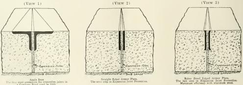
Angle Iron The first steel protection for expansion joints in a Concrete Road used in 1909.
