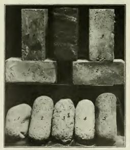
FIG. 1. CONDITION OF VARIOUS BLOCKS DEFORE AND AFTER RATTLER TEST, 1,800 REVOLUTIONS.
