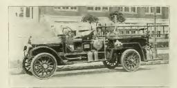
motor and is of the worm drive type. It is equipped with step type fenders, three-way turret pipe, 40-gallon chemical tank, 250 feet of 3/4 four-ply chemical hose, 1,200 feet hose body and all other standard equipment. It will be noted that this car was delivered on Goodyear Cushion Tires.
