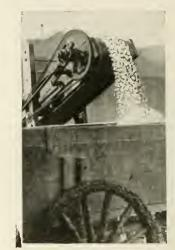
The belt is a regular coveyor belt, is 16 inches wide, 4-ply, ¼-inch rubber top covered and made especially to insure durability. The machine is so constructed that the elevator can be set at an angle of 26 degrees and with ground, where wagon sets, level with track, end of elevator will be  $7\frac{1}{2}$  feet from ground. Machine is guaranteed to carry stone at an elevation of 29 degrees, so it can be raised much higher than  $7\frac{1}{2}$  feet if necessary.
