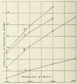
CURVES SHOWING LOSSES IN PER CENT BY WEIGHT IN THE LAST 900 REVOLUTIONS OF RATTLEB TEST OF PAVING BRICKS. MORTAR BLOCKS AND CONCRETE BLOCKS.
