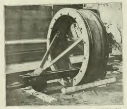
THE TESTING BULKHEAD FOR APPLYING THE PNEUMATIC TEST TO JOINTS IN CAST-HON PIPE LINES, AS DESCRIBED IN THE ACCOMPANYING ARTICLE. PIPES ARE SEVENTY-TWO INCHES IN DIAMETER.
