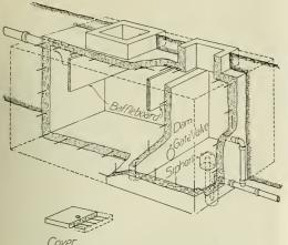
II. SEPTIC TANK, for use where sub-irrigation is practiced, showing tank interior partly exposed as if a portion of the tank were cut away.
