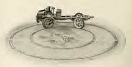
The Walter four-wheel drive tractor making complete turn in circle 25 feet in diameter.
