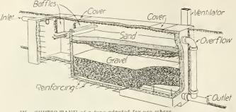
IV. SEPTIC TANK of a type adapted for use where final disposal is made by means of broad irrigation. This view shows the construction as the partly cut away to expose the interior view.
