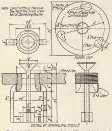
Fig. 65. Details of Sprinkling Filter Nozzle
