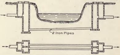
Fig. 15. Sectional Elevation and Plan of Inverted Siphon.
