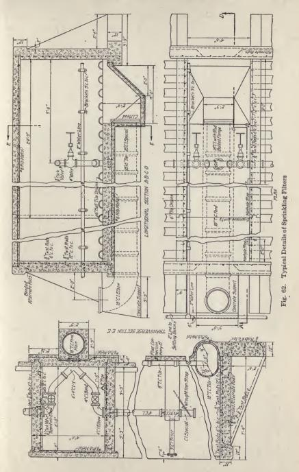
148. Results. The effluent from filters of this type is more putrescible and usually shows a marked reduction in bacterial count over the raw sewage. These filters are self-cleansing, freeing themselves of the accumulated material after it has been mineralized. The effluents are, therefore, not clear, but this suspended material may be removed by settling.
