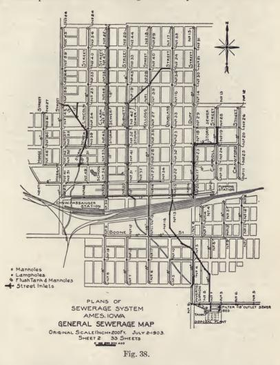
sewers immediately below their profiles, to permit the exact location of manholes, etc., and of the sewer itself in the street.
