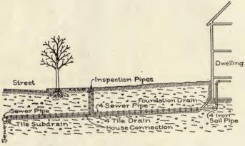
Fig. 6. Street Sewer, Subdrain, and House Connection.
