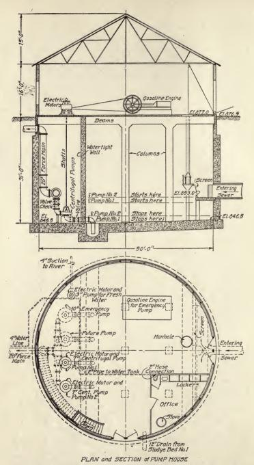
Fig. 71. Plan and Section of Connellsville Proposed Sewage Pumping Station
