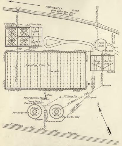
Fig. 55. Plan of Sewage Disposal Plant at Connellsville, Pennsylvania
