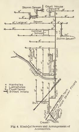
Combined sewers are those constructed to carry both sanitary sewage and storm sewage. With the combined system, the manufacturing sewage also usually goes into the combined sewers.
