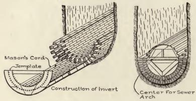
Fig. 41. Diagrams Showing Construction of Brick Sewer.
