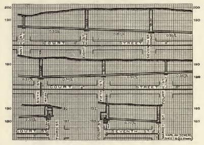
Fig. 39. Typical Sewer Profile Sheet.
