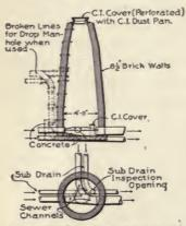
work should be laid with tight shore joints, in 1-to-3 Portland cement mortar; and the manhole walls should be plastered both inside and outside with 1-to-2 Portland cement mortar.
