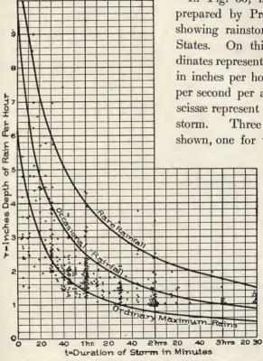
In Fig. 33, is given a diagram prepared by Prof. A. N. Talbot, showing rainstorms in the Central States. On this diagram the ordinates represent the rate of rainfall in inches per hour (which = cu. ft. per second per acre), while the abscissæ represent the duration of the storm. Three curves are also shown, one for very rare rainfalls.
