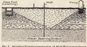
Fig. 3. Showing How Contamination of Well Water may Occur through Proximity of Cesspools and Other Sources of Filth.
