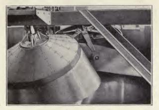
Fig. 44. Reinsch-Wurl Screen in Experimental Plant, Dresden, Germany
