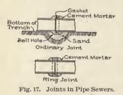
nearly as practicable an absolutely water-tight job. In Fig. 17, the upper joint shown illustrates the form commonly employed.
