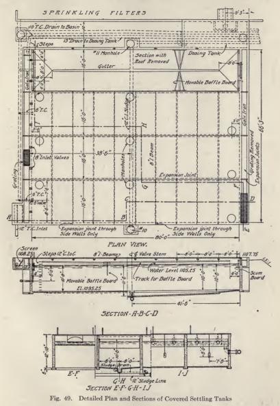
gate valves located immediately below the flow line. A distributing baffle of wood is constructed across the inlet end of each tank oppo-
