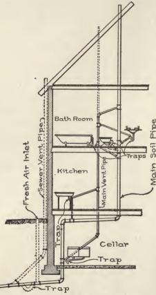
Fig. 35. Diagram of House Sewerage System.
