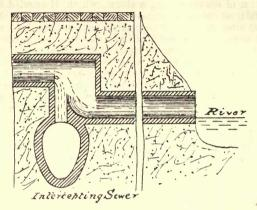
interceptor the opening through which the foul sewage drops is generally made smaller than is necessary, and is afterwards enlarged to suit the requirements of the case as ascertained by trials.
