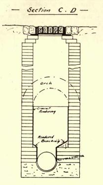
where it is necessary to reduce the diameter quickly. In order to take the cover care should be taken that the form of the dome is not such as to make it difficult for a man to enter and climb down the manhole on the step irons. The curve of the dome should, therefore, be flat, and if the shallow depth of the manhole renders this impossible, a manhole of rectangular form should be used.
