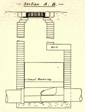
4ft. 6in. above the sewer invert, with a semi-circular arch above that (a flat roof would do as well). The main sewer runs into a half-pipe channel, which is bedded in the manhole. It is equally good if this channel is formed of cement worked to a polished face, but unless the engineer is quite sure of obtaining men capable of making such channels properly it is best to put in glazed stoneware channels in manholes. These channels can be procured
