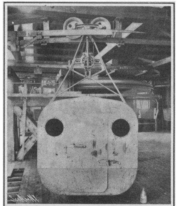
The Passenger Car Used on the Cableway.
