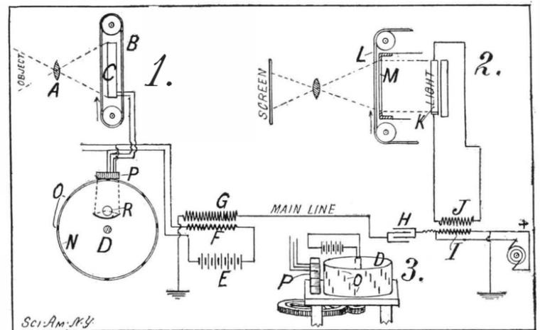
DIAGRAM OF THE APPARATUS FOR TRANSMITTING SIGHT.
