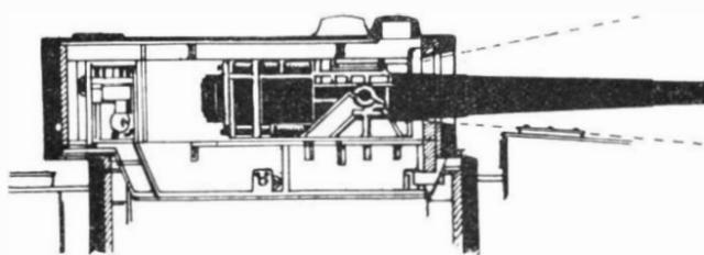
Section Through 13-inch Turret of "Kearsarge," Showing Vertical Front Wall and Large Ports.
