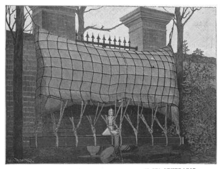
beam is suspended. To the bar chains are lashed which run under the bottom of the ship. The bags are connected by means of pipes with acetylene generators.
