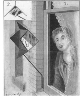
The reflector, it is evident, can be used in armories and towers, the grilled windows of which are so narrow that it is usually impossible to see objects at either side. ----
