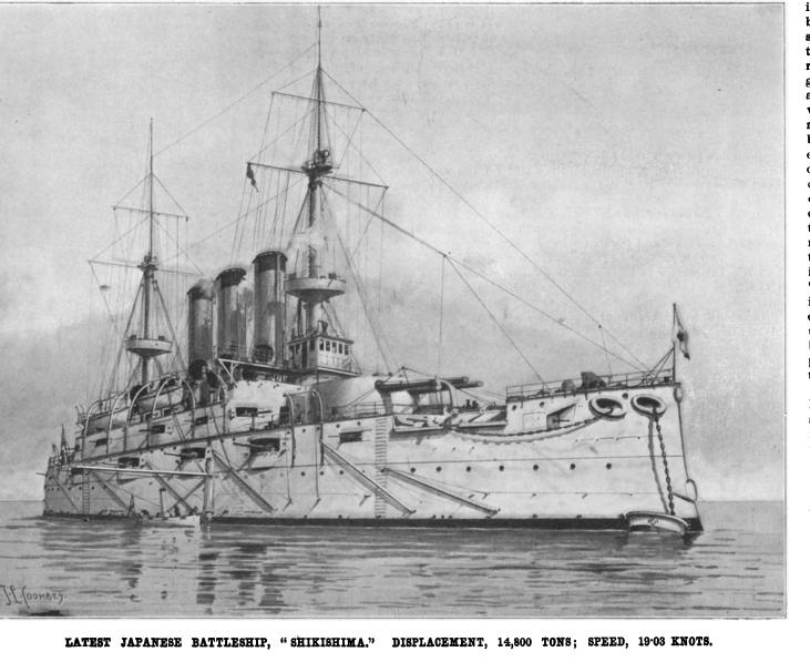
by 6 to 8-inch shields. The intermediate battery consists of fourteen 6-inch rapid-fire guns, which are mounted within casemates on the broadsides, eight of them on the main deck and six on the upper deck. All of these casemates are protected by 6inch armor. The two 6inch guns at each end of the upper deck battery are capable of being
