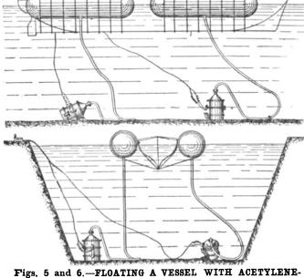
Figs. 5 and 6.—FLOATING A VESSEL WITH ACETYLENE GAS BAGS.
