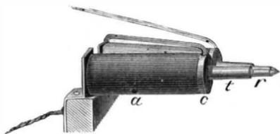
inflames. The apparatus thus constitutes a safety valve, preventing the pressure from rising above a certain degree, which can be regulated at will. The gas which escapes, being at once consumed, cannot give rise to accident.
