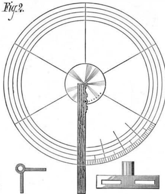
INDEX PLATES FOR GEAR CUTTING.
