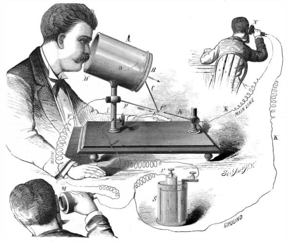
NEW DETAILS OF TELEPHONE ARRANGEMENT.
