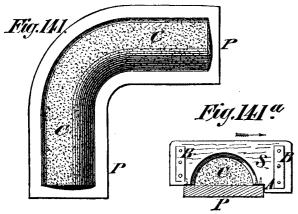
S the strike: this latter is cut from a piece of board from  $\frac{3}{8}$ to 1 inch thick, the semicircular hole cut in it being the size of the required core. The grain of the wood may run in the direction of the arrow. It is strengthened, if necessary, by the two battens shown in Fig. 141 a, at B B. The edges of the semicircle are beveled off, which causes the strike to work more smoothly and correctly over the composition forming the core.
