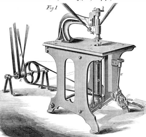
M. T. BOULT'S MOLDING, CARVING, AND PANELING MACHINE.
