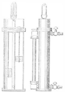
of the large stone, the difference in the weight, operating on a cam lever and a supplementary lever, will raise the safety valve, and admit the steam to the whistle. If water be again pumped into the boiler, and raised high enough to submerge both stones or weights, the gravity of the weights becomes relatively what it would be if both were out of the water, again raising the valve and giving the alarm, either of these causes being determined by inspecting the glass
