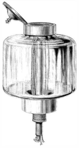
to the journal by capillary attraction. Much practice is necessary to adjust the size of this wick to the amount of oil it is desired to deliver, which depends on the size and velocity of the shaft journal, weight, etc. If the wick fits too tight or the oil gets too low the supply of the lubricant is diminished, while if the wick is loose or the cup too full the amount delivered is too large. The cups, in fact, act on the principle of gravitation as well as of capillary attraction.
