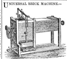
This Machine has been thoroughly tested by the most extensive Brickmakers in the country, who consider it the best. Its principal advantage is that it is a horizontal machine, which makes it superior over any other for making the best Front or Common Brick. Its construc-tion is very simple, and is not liable to get out of order. All machines are warranted. For circular, with full de-scription, address FREEMAN JACOBIE, No. 254 Broad-way, New York, or JOHN BRIDGFORD, Albany, N. Y.
