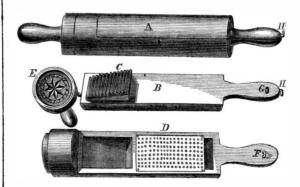
grated spice. E is one end of the roller, which screws on the pin, and when separated is a butter print, as seen. The parts longitudinally separated are held together by a dowel pin at the end of the steak breaker that engages with a corresponding hole in the rolling pin, and by a staple, F, fitting into a recess, G, and secured by the spring pin, H. This combina-
