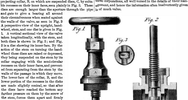
tion, is made through the valve for the steam, of the full size of the pipe. The stem is packed in the usual manner by the screw gland, D.
